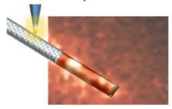
Tip-enhanced Raman spectroscopy (TERS) is a novel technique that combines the high spatial resolution of atomic force microscopy (AFM) with the chemical information of Raman spectroscopy, thus breaking the diffraction limit associated with confocal Raman microscopy. We apply this to study carbon nanotubes and other nanostructured materials.
