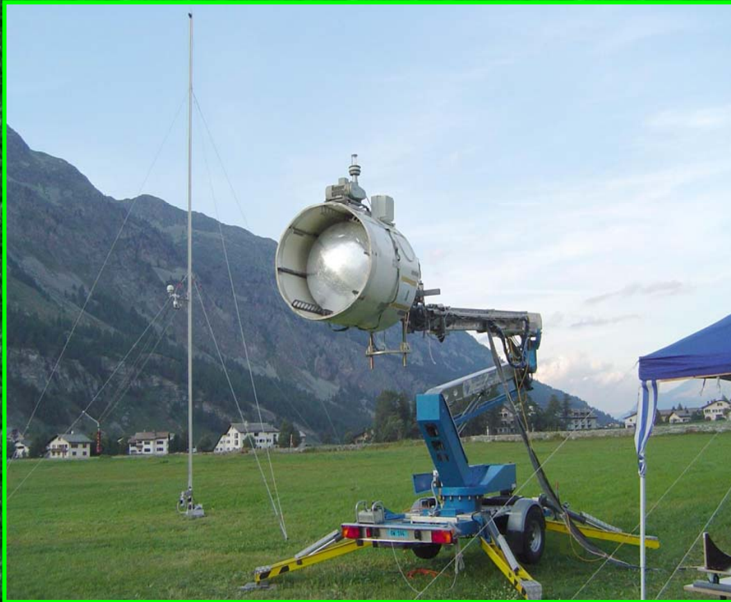
The calibration unit at 3 m in the field
