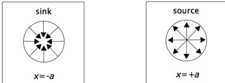
Figure 2.1.: A schematic for a \mathcal{PT} symmetric system. A sink and sink are located at equal distances of a from the origin. The system is odd with respect to parity \mathcal{P} because it physically interchanges the individual subsystems and odd with respect to time reversal \mathcal{T} as it turns the sink into a source and the source into a sink. Therefore the system is even with respect to \mathcal{PT} .
