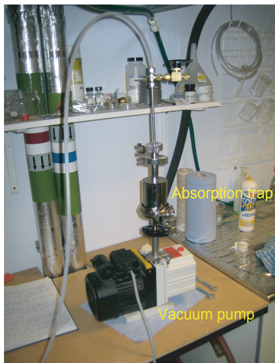
Figure 10: Absorption trap for pump oil
