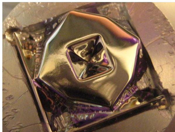
(f) Pyramid etched in HNA for 90 minutes
