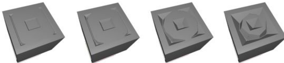
Figure 5.4: Simulation of observed underetching effects - along with the pyramid hollow etching in the centre of the block, we observe underetching effects from the corners of the alignment marks.
