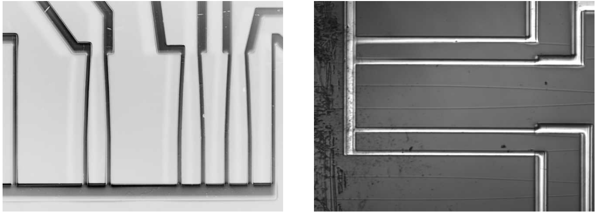
Figure 2.15: Microscope images of sputtered wires. Left, NiCr layer only on a glass slide. Right, NiCr and gold on a waveguide chips. The waveguides can be seen emerging from underneath the heaters. The rugged area to the left is some residue from the mirror coating that has spilled onto the chip top surface.
