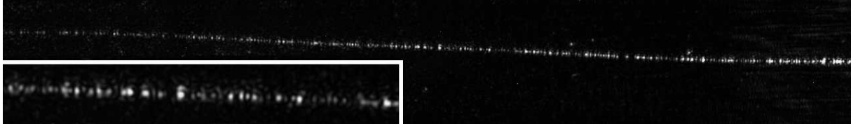
Figure 6.1: Propagation loss in UV-written waveguides. A 30s CCD exposure with maximum gain reveals that light is being scattered at many localised sites along the waveguides. Inset: detail of the central area
