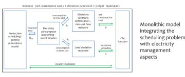
Electricity consumption accounting – discrete time grid with task-time slot relations via event binaries
