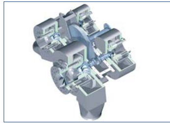
Example of integrally geared centrifugal compressor (reference: www.siemens.com/entry/coc/en)
