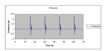
Filling of steam filled pipe with saturated water at atmospheric pressure showing water packing problem when liquid level crosses the cell boundaries
