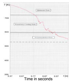
Intermittent contacts ahead of quench front give precursory cooling. Quench front temperature is homogeneous nucleation temperature. 16
