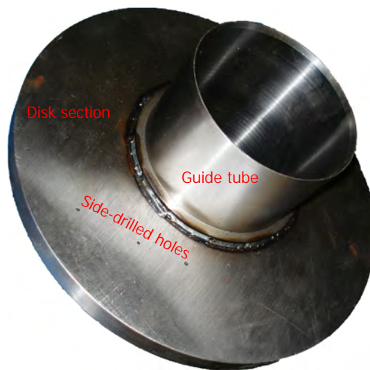
Figure 5.11: A photograph of a rotor bore calibration test piece. The disk section containing the target reflectors (side-drilled holes) and the guide tube are clearly identifiable. The guide tube also extends out of the far-side of the disk section. Note the joining material between the two sections of the test piece. Photo taken by author at RWE npower's Ferrybridge site.
