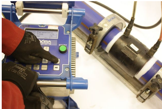
Figure 1.4: Electrofusion welding procedure. Coupler containing heating wires is connected to external current supply. [30]
