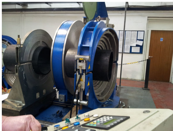
Figure 1.2: HDPE pipes (~500mm diameter) with heater plate between in butt fusion process at Plasflow plc.
