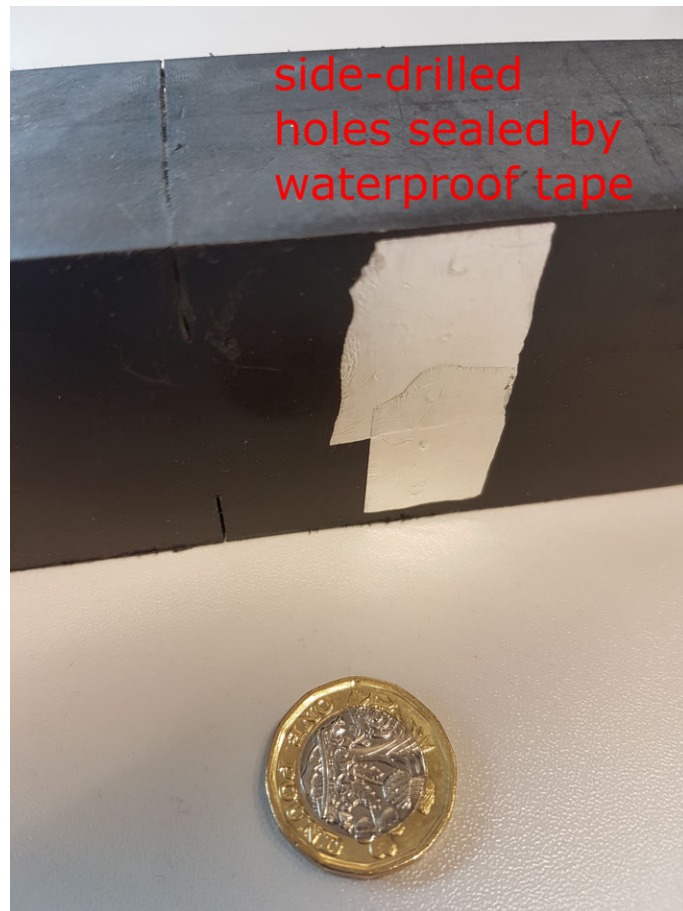
Figure 8.2: HDPE pipe test block SDHs, waterproof tape covering their air gaps, and smoothed outer surface.
