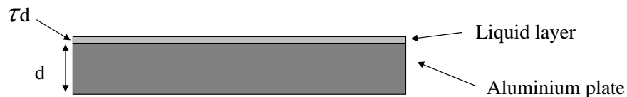
Figure 6.1: Schematic of an aluminium-water bilayer. \tau is the ratio of liquid thickness to plate thickness.
