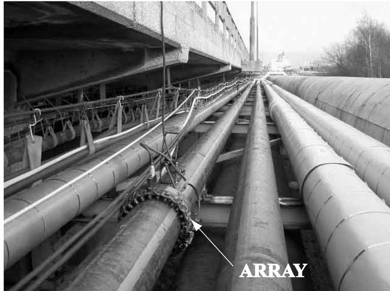
**Figure 1.2:** Transducer array employed for guided wave inspection of pipelines.
