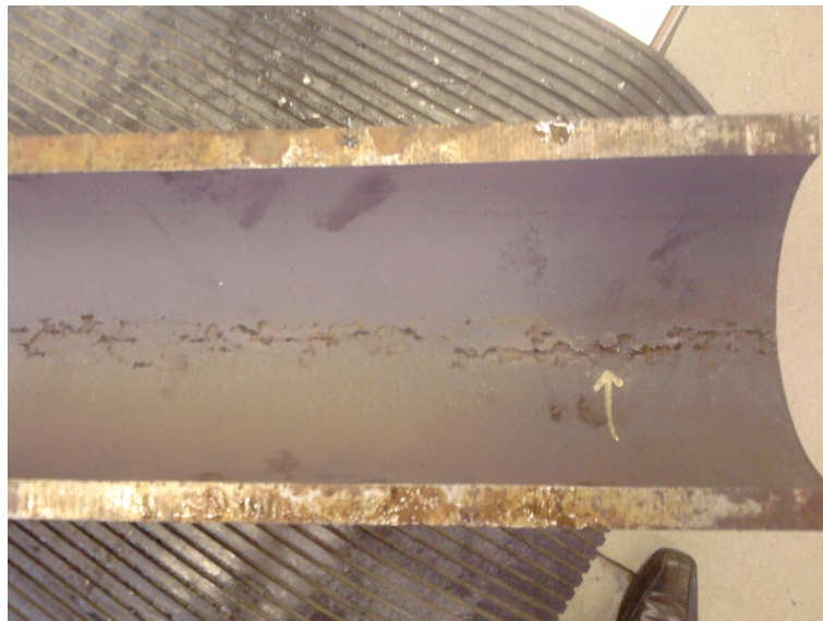
Figure 1.2: Sectioned 4" pipe with longitudinally aligned pitting. Axial cracks have a tendency to develop at the bottom of these pits when they are aligned in this way. Note the pitting is highly localised to one circumferential position with the rest of the pipe remaining relatively smooth.
