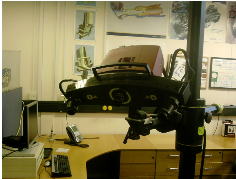
Figure 6.6: White light scanner used to scan the inner surface of a pipe section and provide quantitative data about the condition of it.
