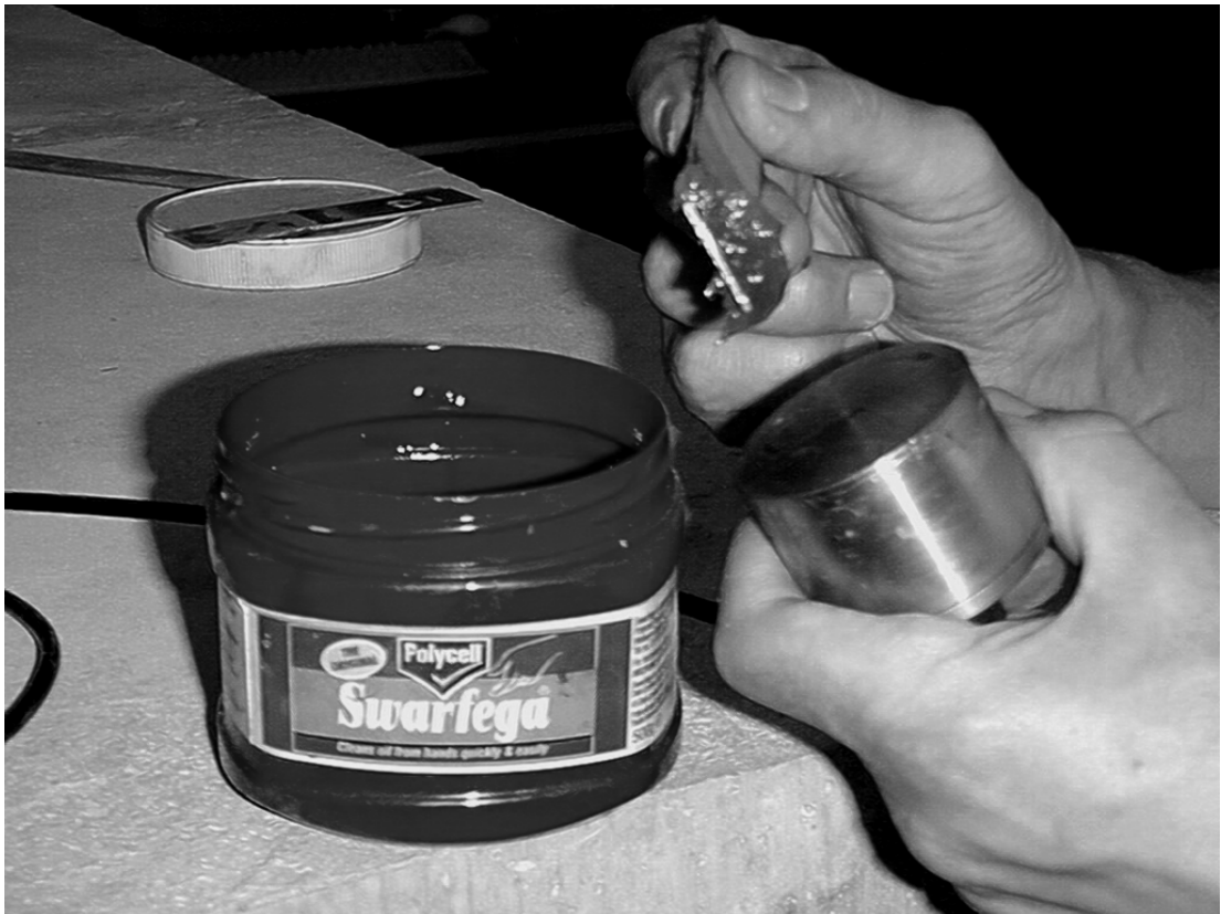
Figure 6.9. Conventional coupling of transducers using Swarfega.
