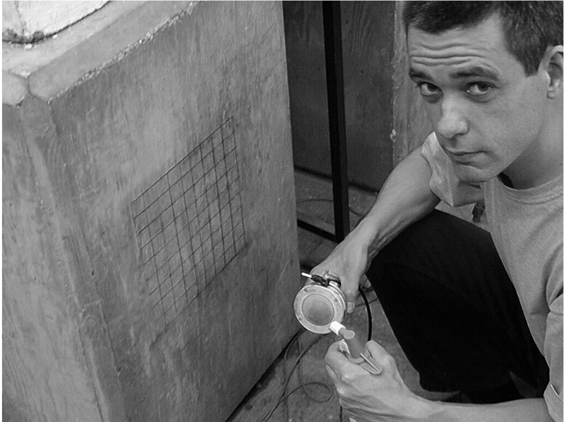
Figure 6.10. Film of water sprayed onto membrane shoe.
