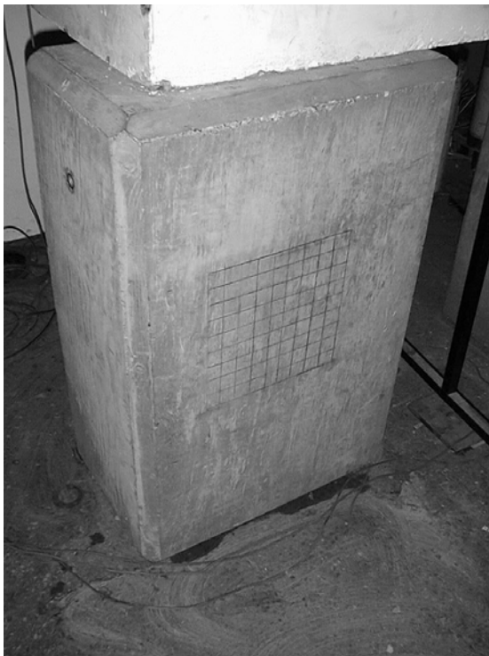
Figure 6.5a. Photograph of grid pattern marked out on the flat surface concrete block.
