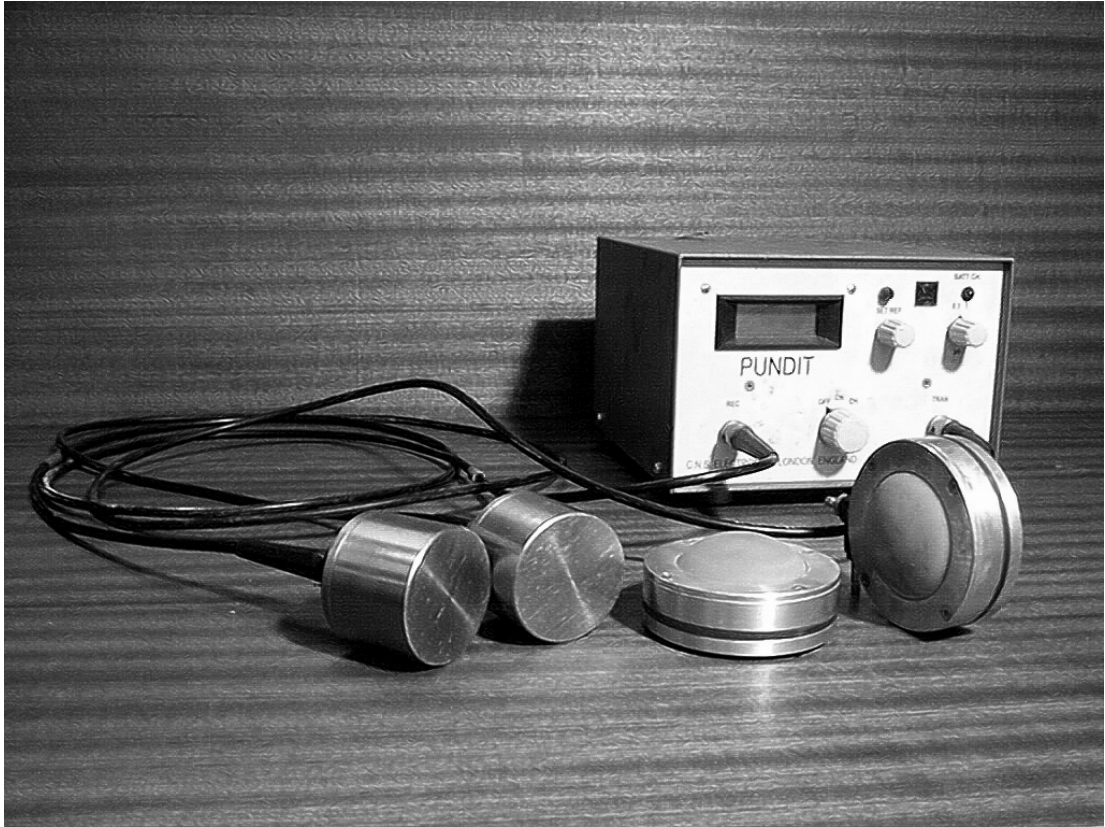
Figure 6.8. Pundit apparatus, 54kHz transducers and prototype membrane shoes.
