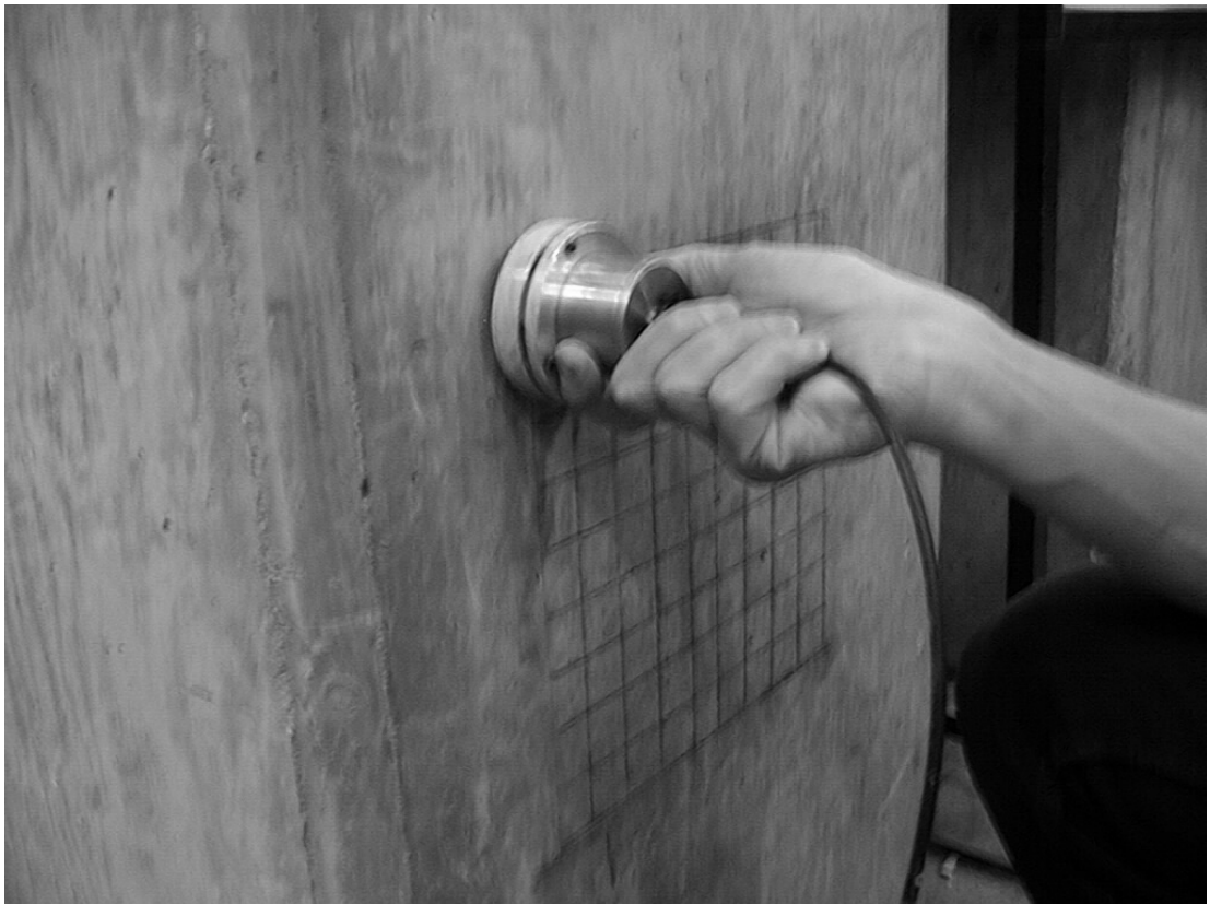
Figure 6.11. Application of membrane device to grid point on concrete block under test.
