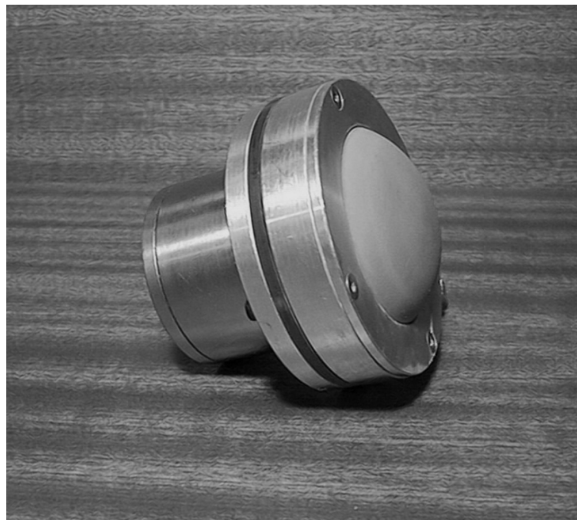
Figure 6.2 Photograph of standard 54kHz transducer coupled to prototype membrane shoe.
