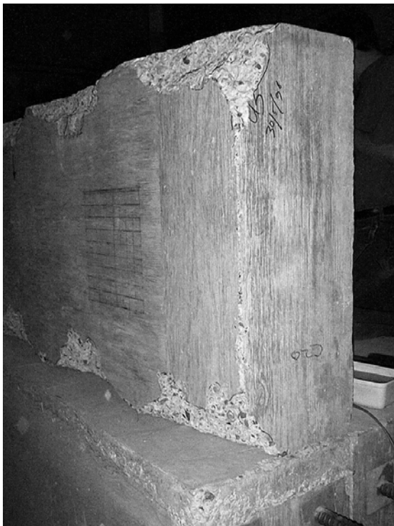
Figure 6.7a. Photograph of grid pattern marked out on the rough surface concrete block – timber shuttered surface side.
