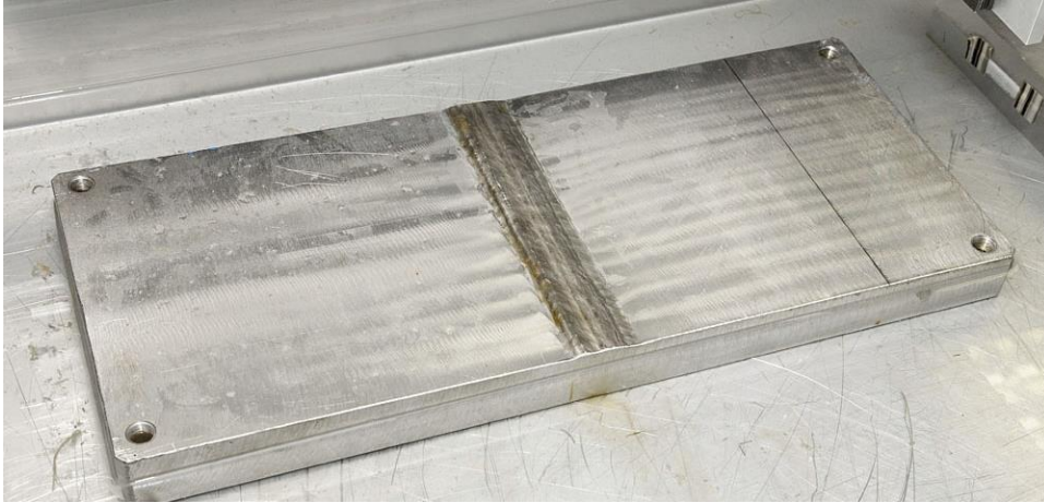
Figure 6-2 Photograph of conformable phased array welded evaluation block 2 (Rolls-Royce, 2008b).
