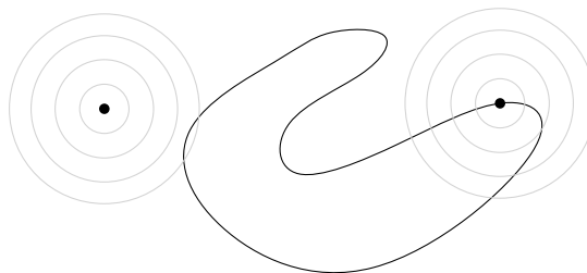
Figure 4.1: The Linear Sampling Method relies on the fact that it is possible to create field values on the boundary of a scatterer, such that a field that appears to radiate only from a single point within the scatterer. However it is not possible to do the same for a point outside the scatterer.
