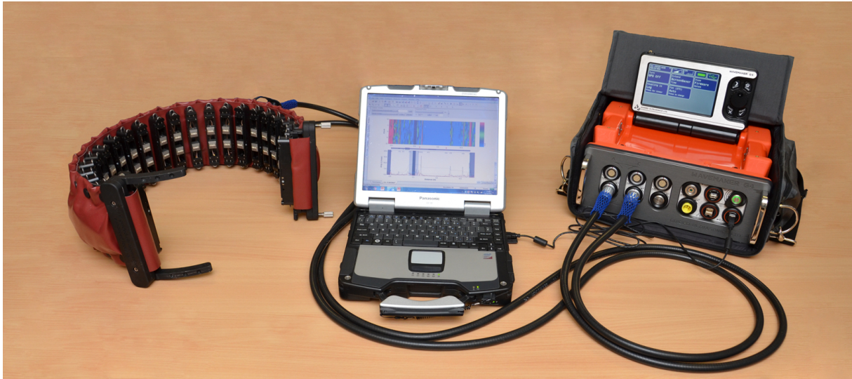
Figure 2.3: Example of commercial guided wave inspection equipment, consisting of a Guided Ultrasonics Ltd. flexible deployable ring sensor [54] (left), a Guided Ultrasonics Ltd. Wavemaker® G4 [54] integrated signal generator and receiver (right), and a laptop computer (centre) to set the inspection parameters and to visualise and analyse the inspection results.
