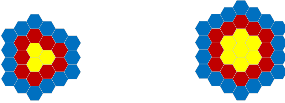
(a) Clusters for T = 2 , T = 4 and T = 6 are illustrated with yellow, (b) Clusters for T = 3 , T = 5 and T = 7 are illustrated with yellow, yellow and red, and all three colors, respectively.
