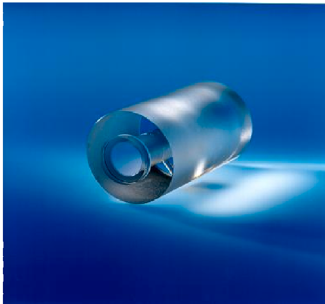
Figure 4.18: Picture of one the ULE cavities used in our experiment.
