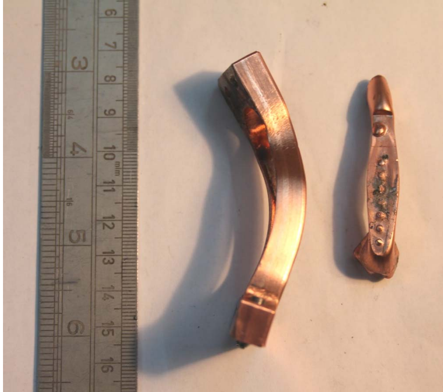
80x20mm electrode, with support (left) and target plate (right)
