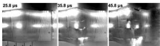
Figure 3: A series of images from a cylinder expansion experiment on the ISP gas gun, where the cylinder has been cooled to \sim 150 K. Time is after impact, where A-D are the location of PDV probes used to measure the expansion velocity.
