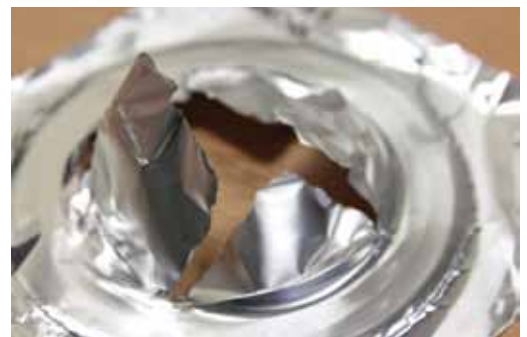
Figure 39: Examples of aluminium diaphragm bulge and rupture.
