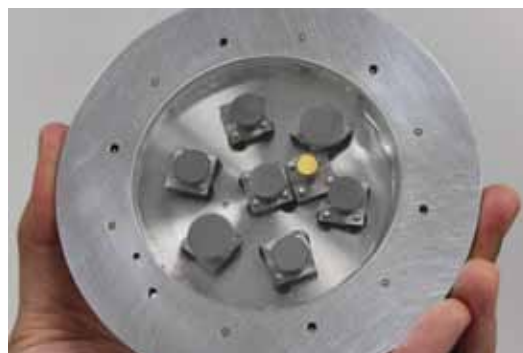
Figure 8: The impact face of the Ta multi-target, showing seven thin foil Ta targets bonded to the rear of a large sapphire buffer plate.
