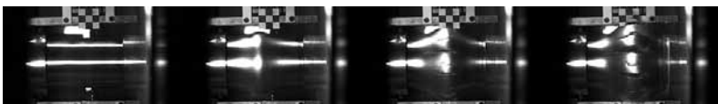
Figure 11: Shows the expansion and eventual failure (left to right) of a stainless steel cylinder that was created using additive manufacturing techniques.
