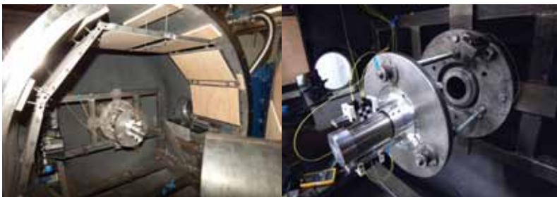
Figure 10: The experimental set up (left) showing the mitigation that was used to reduce the chance of damaging the target tank and the entire cylinder assembly (right).
