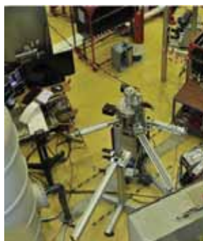
Figure 29: The X-pinch driver used in experiments at CEA Gramat. Use of modern capacitor-switch technology, results in an extremely compact system – 0.5x0.5x1.5metres – supplying ~300kA in 450ns to the X-pinch load.
