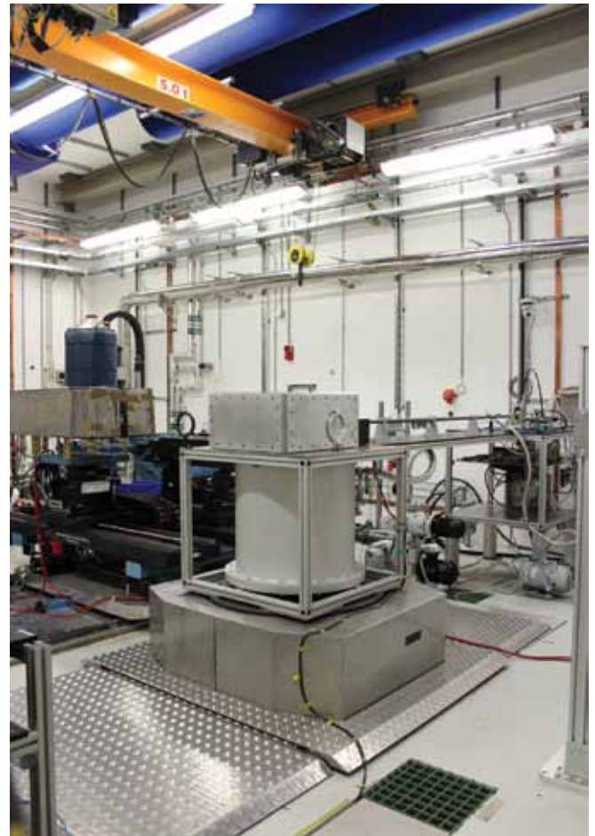
Figure 42: The mesoscale gas launcher installed on the I12 beamline at the Diamond Light Source. The gun has featured in two experimental campaigns, demonstrating the capability for X-ray imaging of dynamic processes in condensed matter.
