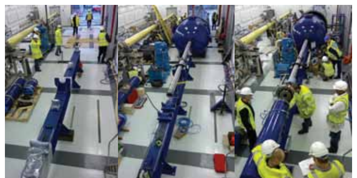
➤ Installation of the large bore gas gun at Imperial (right), completed in February 2011 (above).
