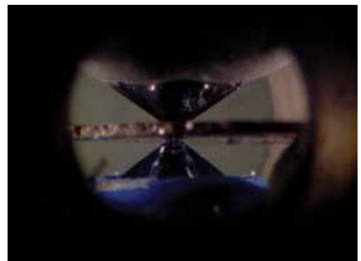
Diamonds in the UCL Diamond Anvil Cell facility
