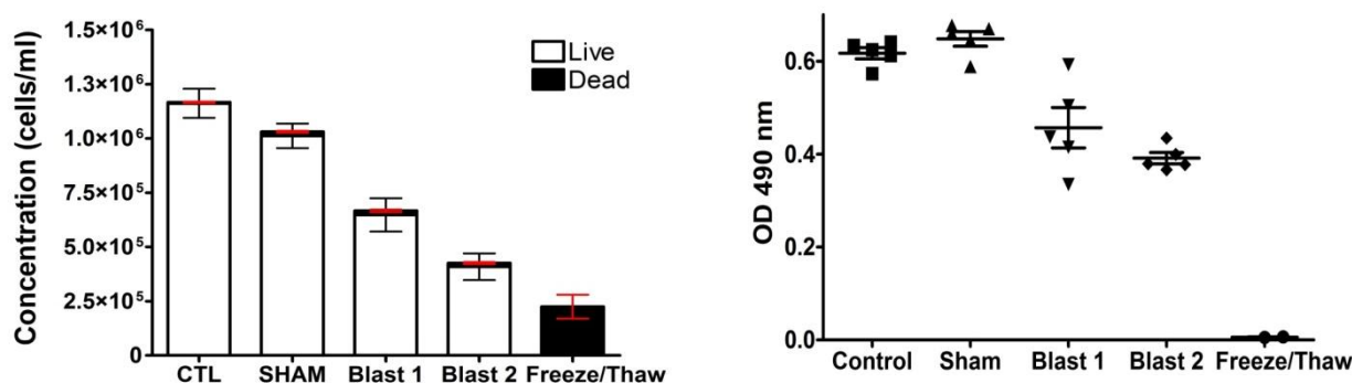
Figure 31: Cell concentration of MSCs subjected to the pressure pulses compared to control, sham samples and the total lysate obtained with freeze/thaw. Right. Cell respiration measured with a MTS colorimetric assay for the same samples as Left.
