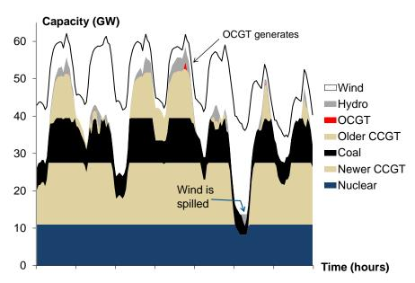
Over the whole year, roughly 60% of the energy produced by the additional wind capacity (comparing 30 GW and 7 GW) displaces output from CCGT stations, and 40% displaces coal output. There is a small reduction in nuclear output (less than 1% of the wind output) and 0.3% of the wind output has to be spilled. The output from OCGT stations is almost unchanged.
