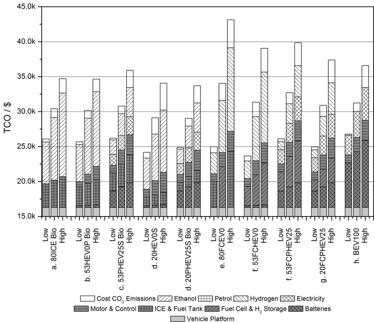
Figure 5: Sensitivity analysis showing the optimistic, central, and pessimistic assumptions for the typical vehicle, for 10 selected power train configurations, all PHEVs have a 25 mile (40 kilometre) AER.
