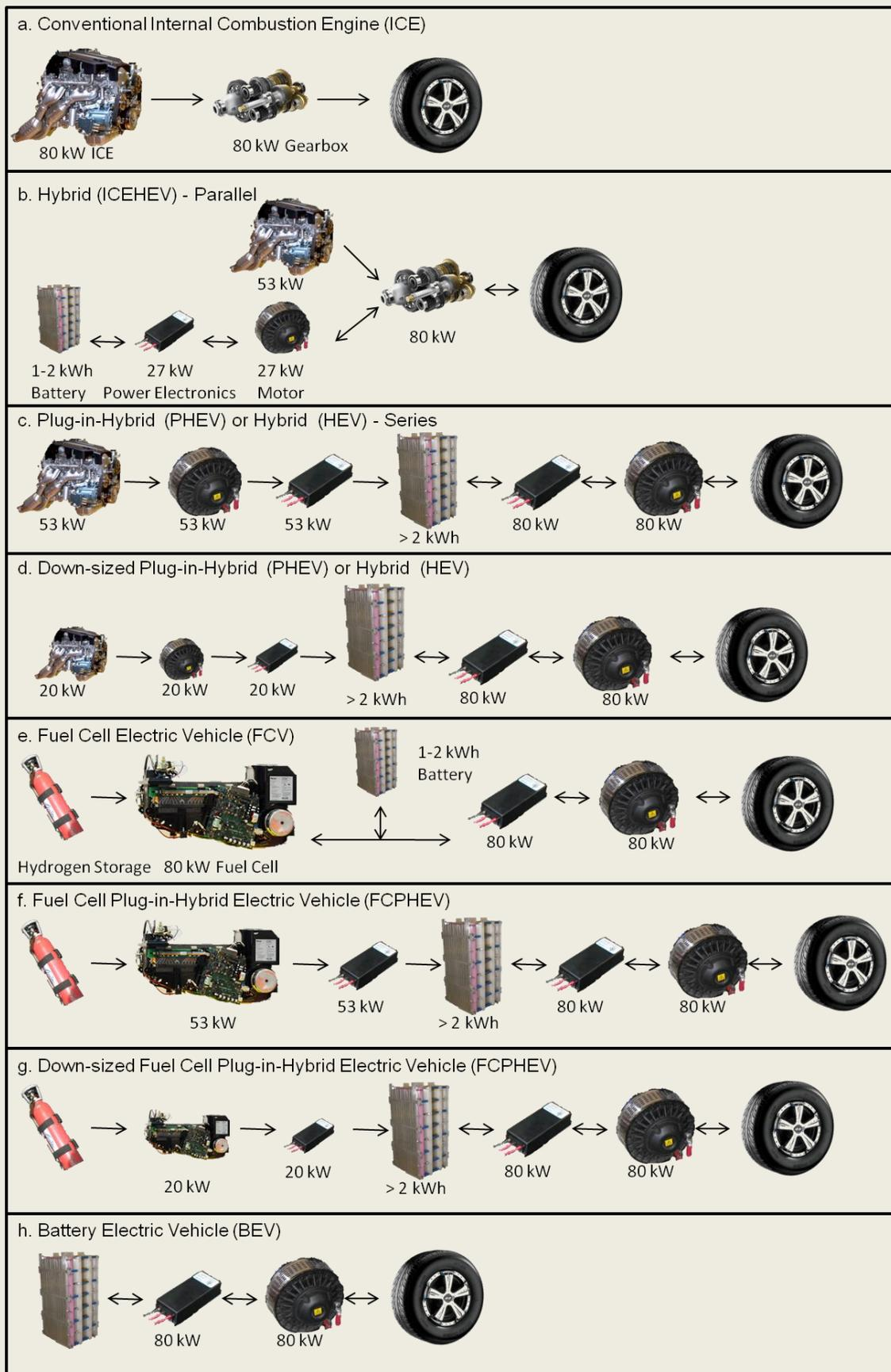
Figure 3. Diagram describing the eight vehicle platforms selected for analysis in the paper; power figures (in kW) are relative to the multipurpose vehicle.
