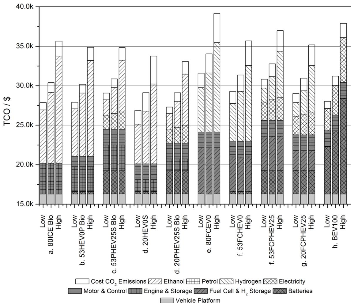
Figure 6: Sensitivity analysis showing the effect of varying energy consumption by a factor of 2. Central assumptions for the typical vehicle. All PHEVs have a fixed battery size and therefore variable AER.
