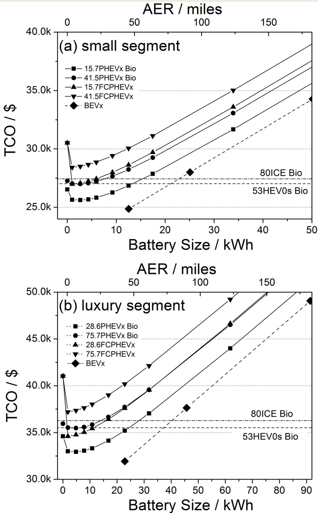
Figure 8: Results of the TCO analysis for PHEV and BEV powertrains for 2 market segments: (a) super-mini and (b) luxury, with variable battery sizes.
