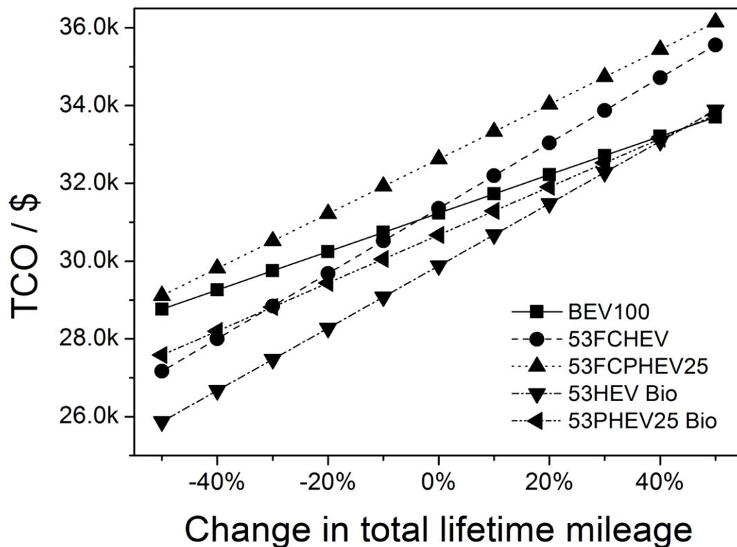
Figure 9: Sensitivity of the TCO of selected powertrains to the utilisation of the vehicle (i.e.: the total miles driven over its lifetime). The figure shows results for the multipurpose vehicle segment under baseline assumptions.
