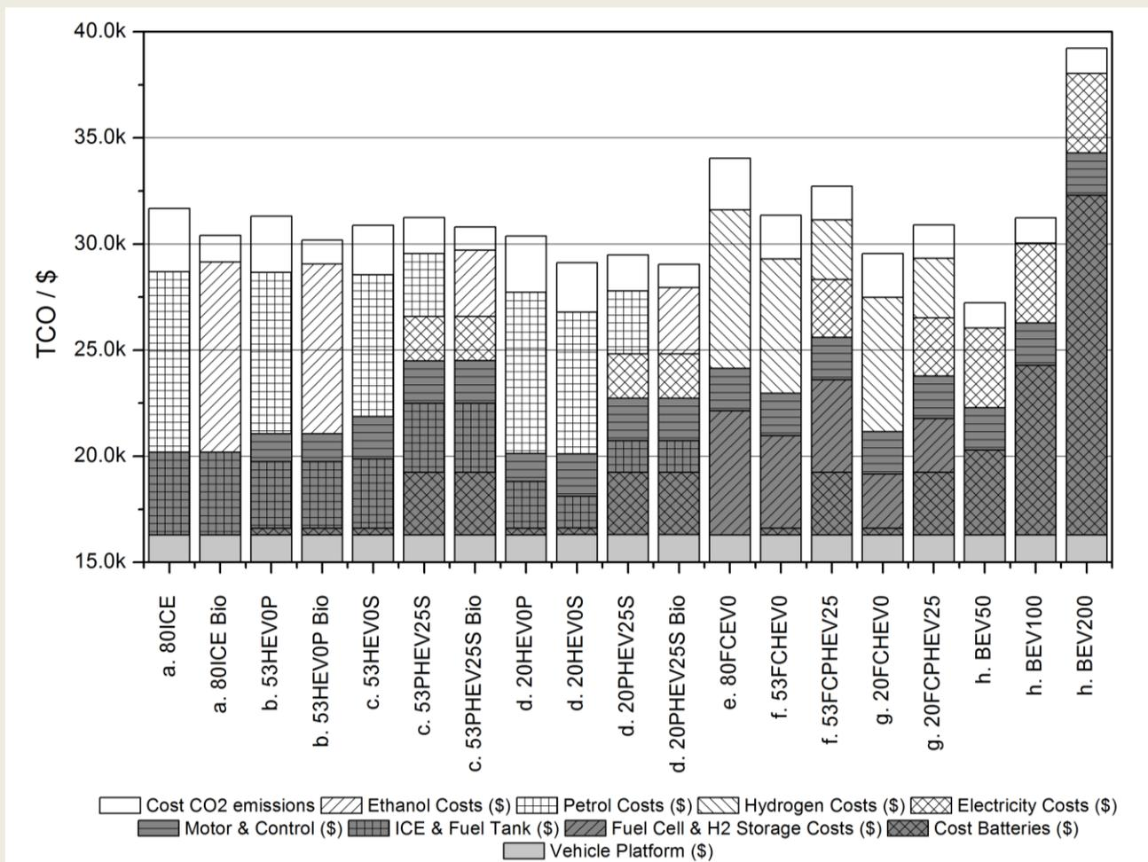
Figure 4: Results of the TCO analysis using the central assumptions for the typical vehicle, with 19 possible powertrain configurations; all PHEVs have a 25 mile (40 kilometre) AER.
