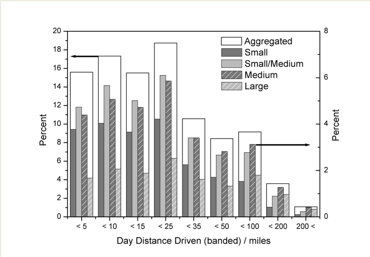
Figure 7: Data extracted from the UK National Travel Survey, showing the aggregated average daily distance travelled by private car in white with the axis on the left, and the breakdown of average daily distance by car types shown in various labelled shades of grey with the axis on the right. Source: <sup>13</sup>
