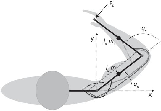
$$\tau_B = \mathbf{H}(\mathbf{q})\ddot{\mathbf{q}} + \mathbf{C}(\mathbf{q}, \dot{\mathbf{q}})\dot{\mathbf{q}}, \quad \mathbf{H}(\mathbf{q}) = \begin{bmatrix} H_{ss} & H_{se} \\ H_{es} & H_{ee} \end{bmatrix},$$
