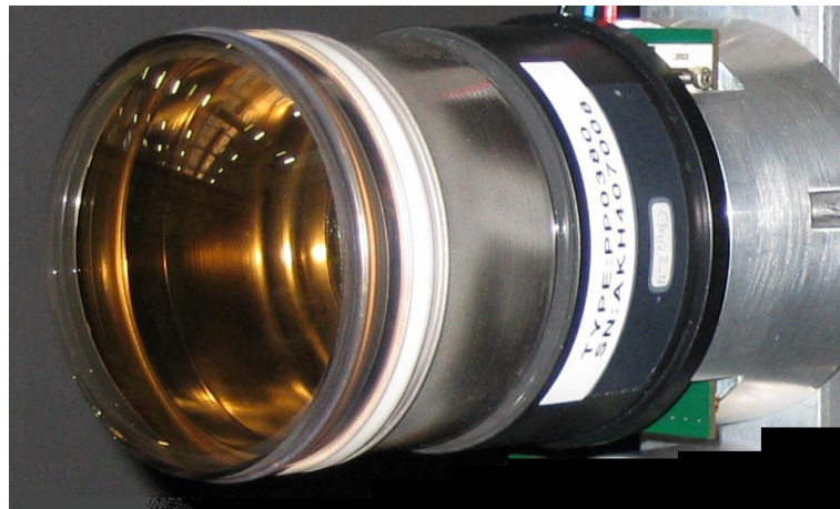
Figure 3.12: (Top) A schematic diagram showing the components of the HPD and the path of a photon \rightarrow e^- \rightarrow sensor. (Bottom) A photograph of a completed HPD.
