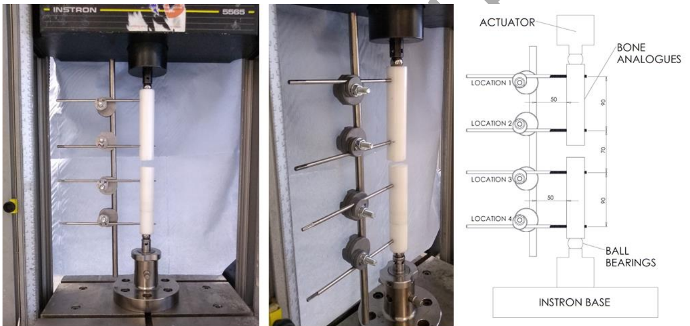
Figure 27 - System mechanical test set up. Moratuwa Mk2 front view (left), Imperial Mk2 isometric view (middle) & CAD drawing (right).
