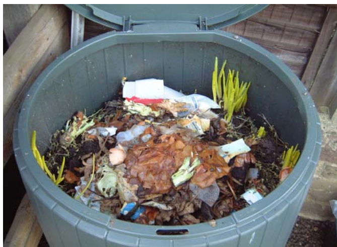
Plate 3.1 Inputs of kitchen, paper and garden waste were recorded by homeowners The Milko standard compost bin has a capacity of 290 l and is fitted with a hinged lid and ventilator. Access to the composted product is provided by a sliding hatch at ground
