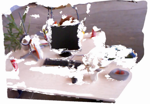
Fig. 1: Fusing the depth predictions of a semi-dense multiview stereo system with the depth and gradient predictions of a CNN allows for the creation of fully dense depth maps at scale. The above projected keyframe depth map was created by DeepFusion from only pose estimates and RGB images.
