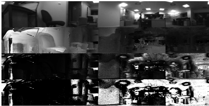
(a) Dataset “Large Office”, one of the measurements, from top to bottom: reference frame, estimated depth map, estimated depth standard deviation map, depth threshold mask.
