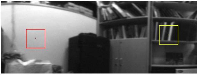
Fig. 2: Depth standard deviation estimation. Patch (A) has low texture and therefore poor depth estimate quality, with patch (B) the opposite. Fitting a parabola provides us with subpixel depth estimate as well as depth standard deviation.
