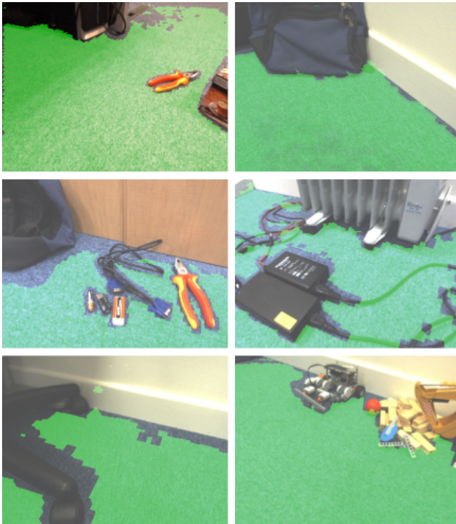
Fig. 9: Free space detected (green overlay) by simple thresholding of the reconstructed elevation map.
