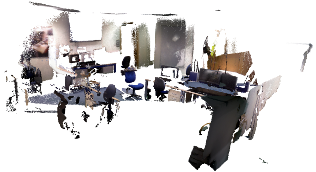
Fig. 1: Tightly integrating pose predictions from the on-board kinematics of a robot arm into RGB-D dense SLAM improves tracking and robustness on challenging trajectories. The above surface reconstruction was captured in challenging conditions with a fast moving robot under conditions where state-of-the-art dense SLAM methods lose tracking.
