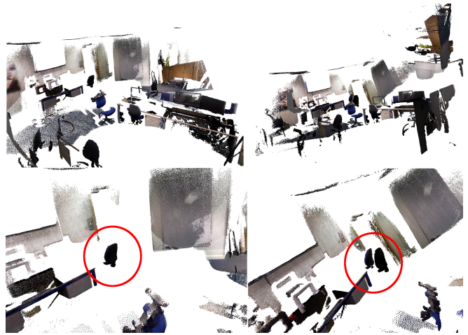
Fig. 4: Qualitative map comparison between KO-Fusion (left) and ElasticFusion (right). The top two images highlight the improvement in global coordinate consistency, whereas the bottom row shows consistency in observing a single object (highlighted in red) before and after a fast rotation.
