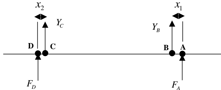
Figure 5.2.13. Illustration of how incorrect assumptions relating to excitation and reference locations lead to reciprocity errors.
