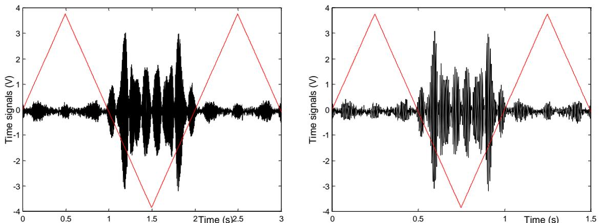
**Figure 7. 28** Time histories (V) for 0.5Hz (left) and 1 Hz (right) scan speed – LDV output (black), mirror driver signal (red).
