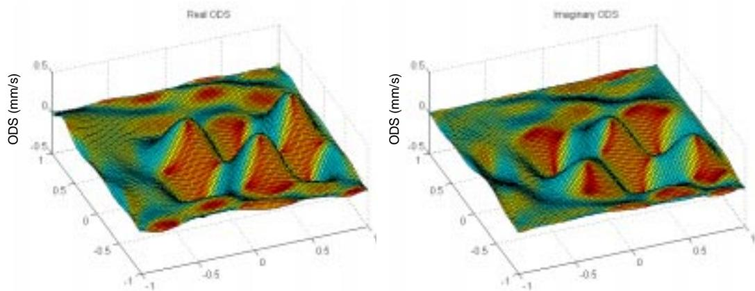
**Figure 7. 66** Real and Imaginary ODS at 211.3 Hz.
