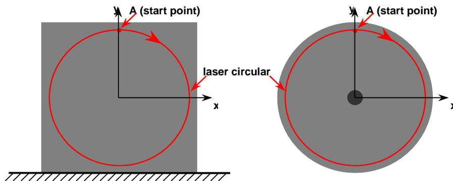
**Figure 5. 32** Cantilever square plate and disc together with the laser beam trajectory.
