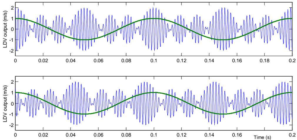
**Figure 5.18** LDV output in the case of ideal and real mirror plotted together with the mirror driver signal.
