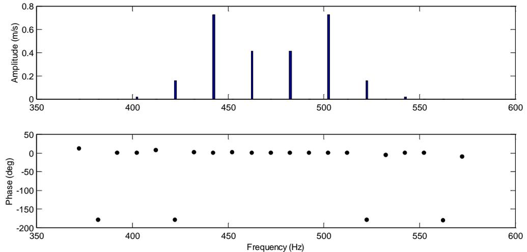
**Figure 5.21** LDV spectrum in the real situation considering the mirror delay in the curve-fit.
