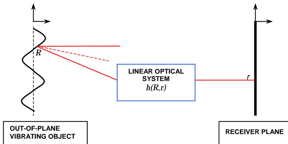
**Figure 2. 8** Schematic of the laser optical path.
