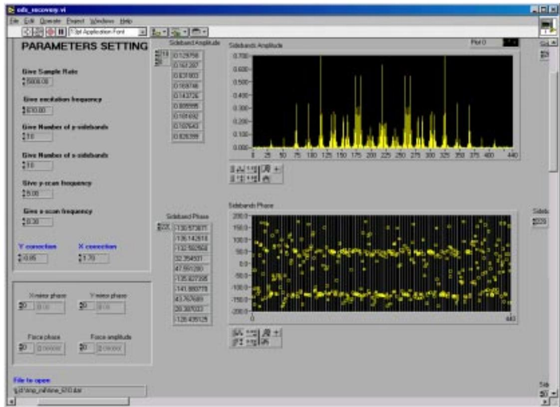
**Figure A. 7** ODS recovery control panel – parameter settings and spectral components visualisation.
