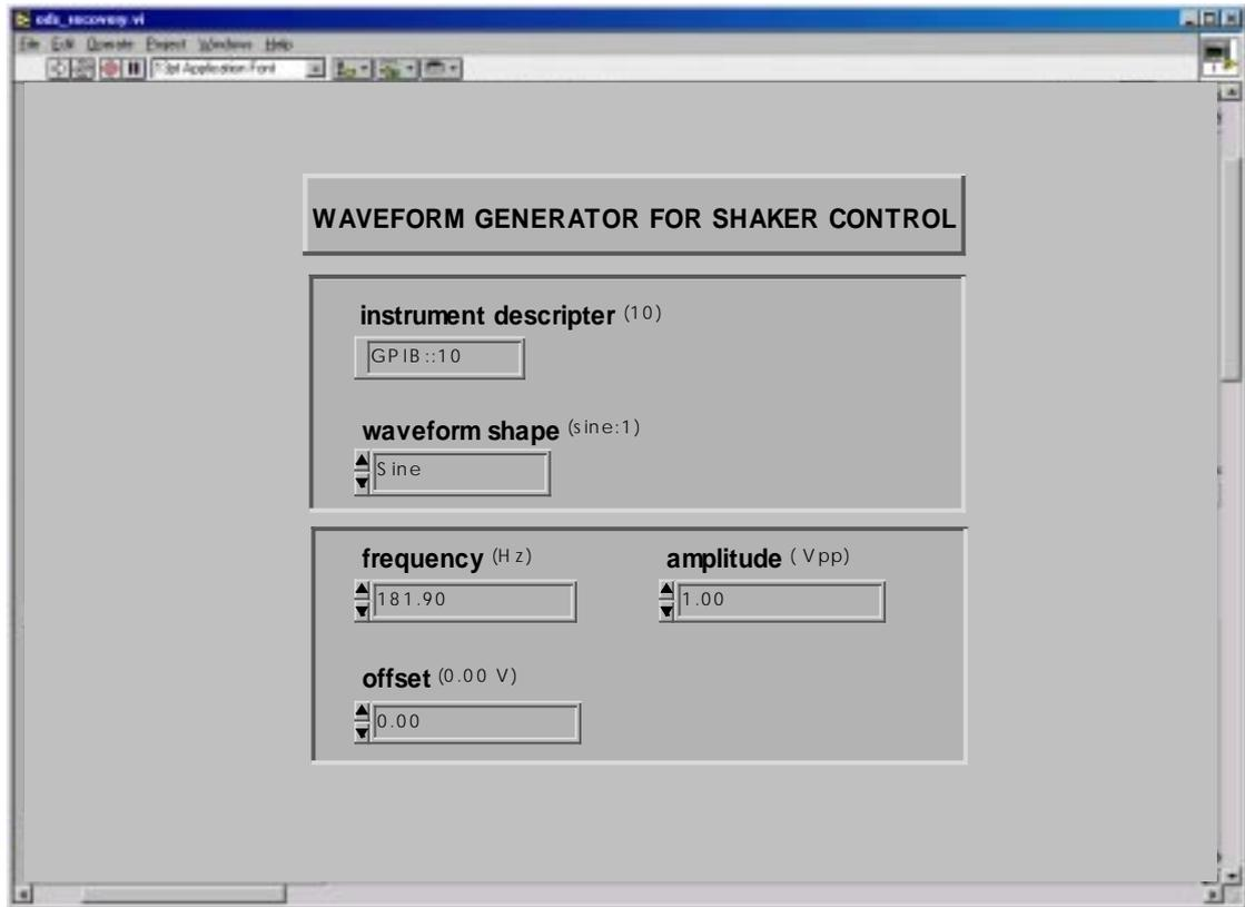
**Figure A. 1** Shaker control panel.
