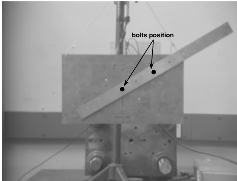
**Figure 7. 4** Assembled structure seen from the laser head position.
