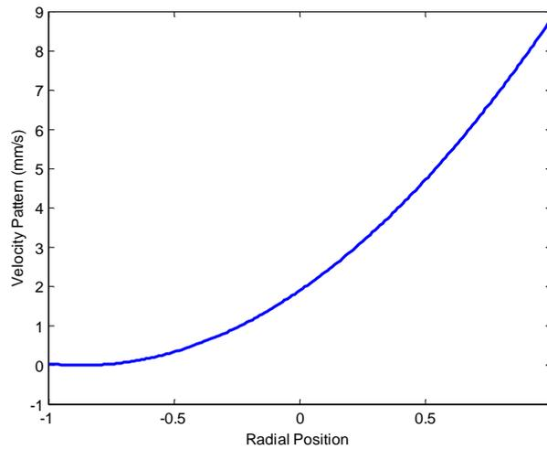
**Figure 5. 101** Radial ODS at 2271 Hz along the radius of the annular disc.
