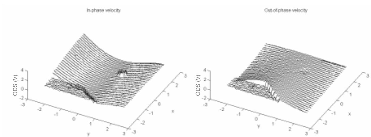
**Figure 7. 54** In-phase ( left ) and out-of-phase ( right ) components of the ODS at 242 Hz.
