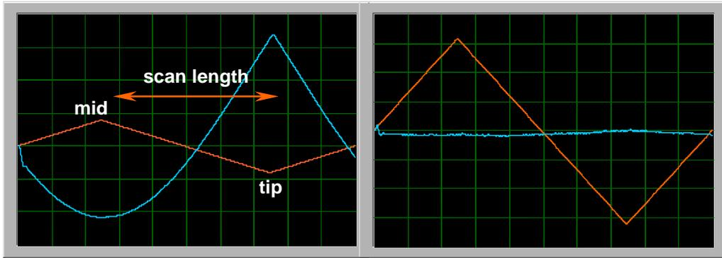
**Figure 5. 5** In-phase and out-of-phase components of the ODS at 58 Hz.
