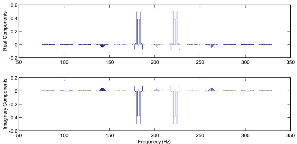
**Figure 5. 63** Real and imaginary components of the LDV output spectrum.
