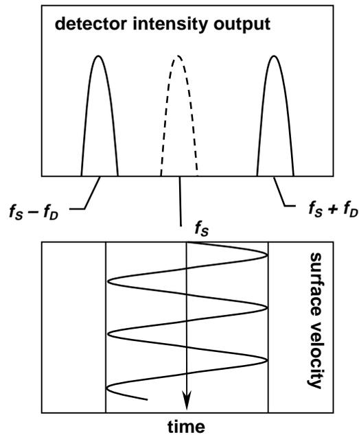
**Figure 2. 20** Frequency shifting and time-resolved velocity, [32].
