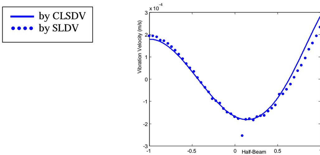
**Figure 5. 30** ODS corresponding to the third mode.
