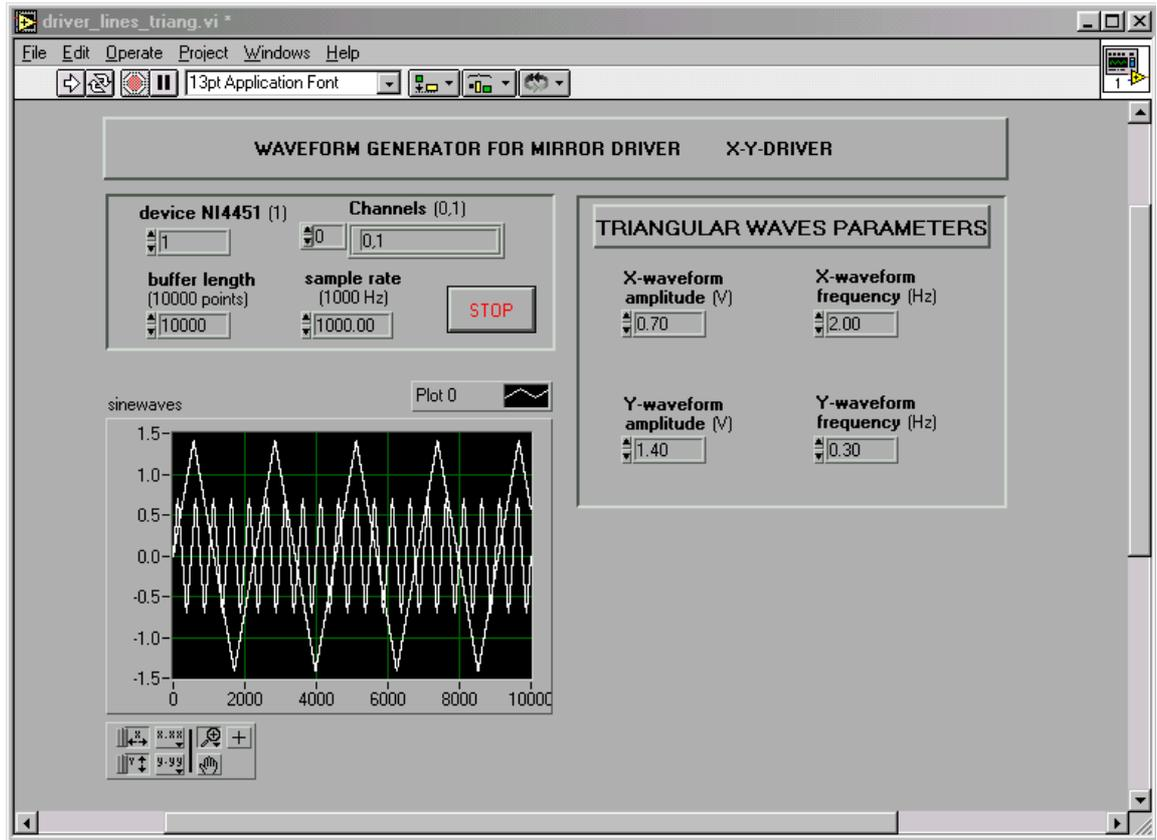
**Figure A. 2** Mirror driver control panel- case of triangular waves.
