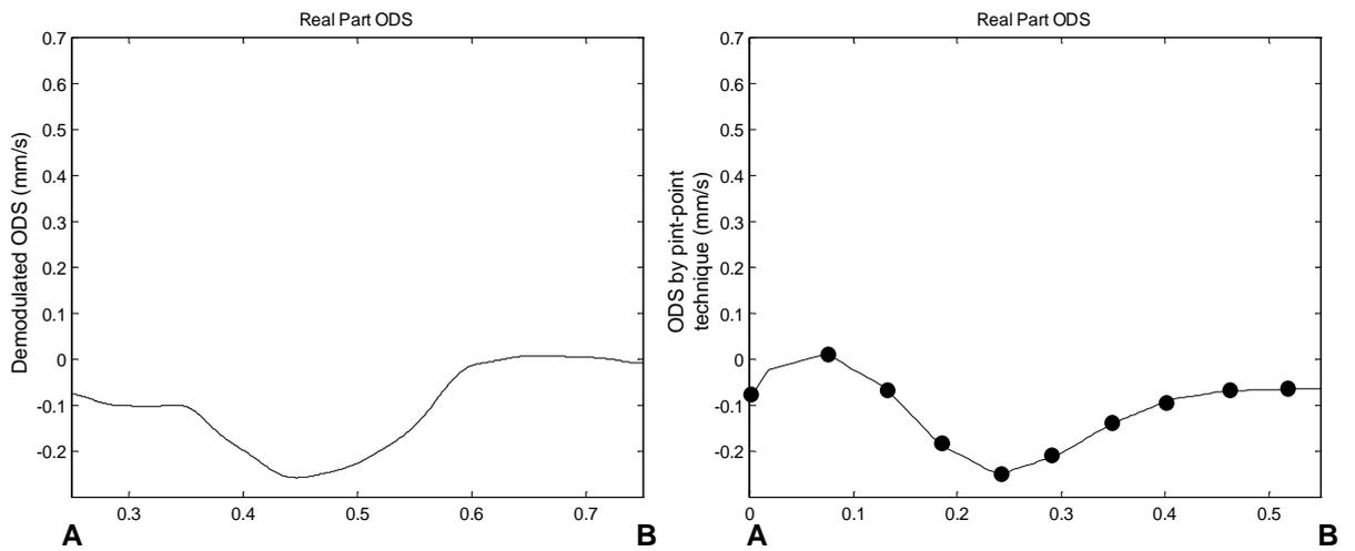
**Figure 7. 36** ODS Real component (mm/s) derived by demodulation (left) and point-by-point scan (right, the vibration response is measured at the marked points only, where the actual measurements have been acquired).
