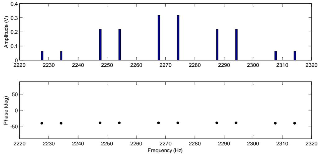
**Figure 5. 100** Sidebands spectral components of the LDV output.
