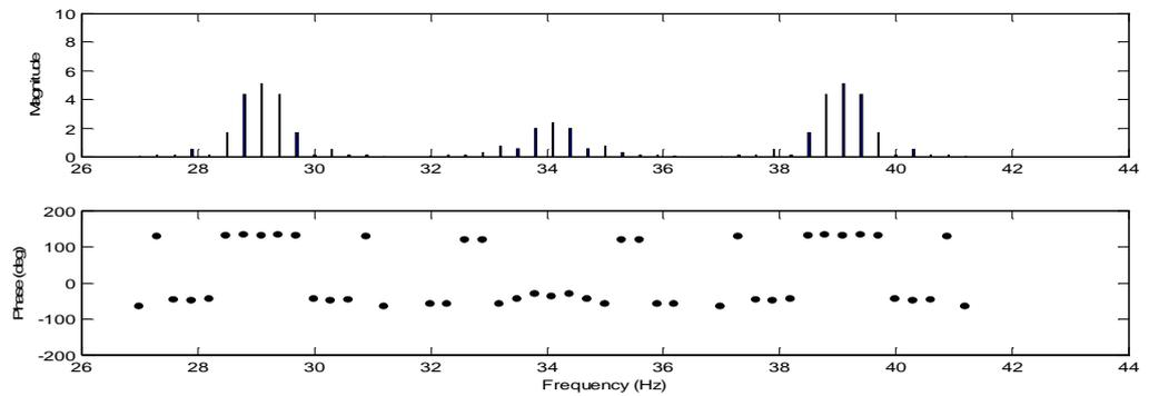
**Figure A. 11** Sideband FRF at the excitation frequency of 34.1 Hz.
