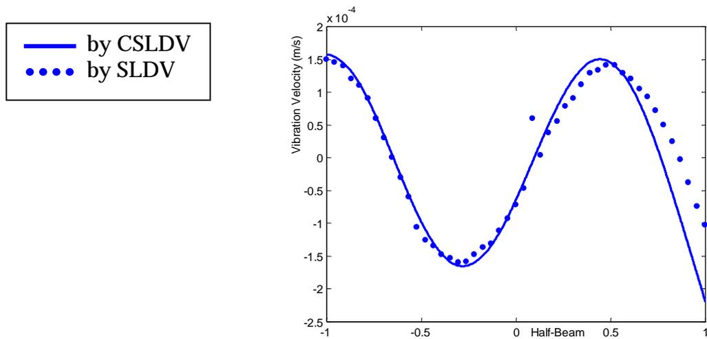
**Figure 5. 31** ODS corresponding to the fifth mode.
