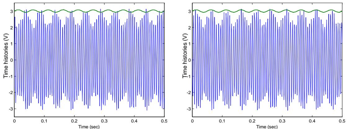
**Figure 4. 26** LDV output signal before and after applying the mirror delay correction.
