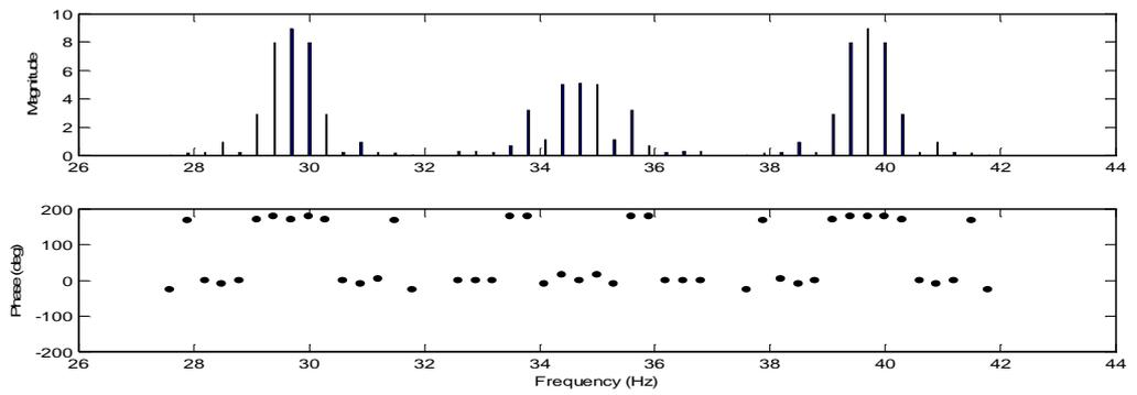
**Figure A. 17** Sideband FRF at the excitation frequency of 34.7 Hz.
