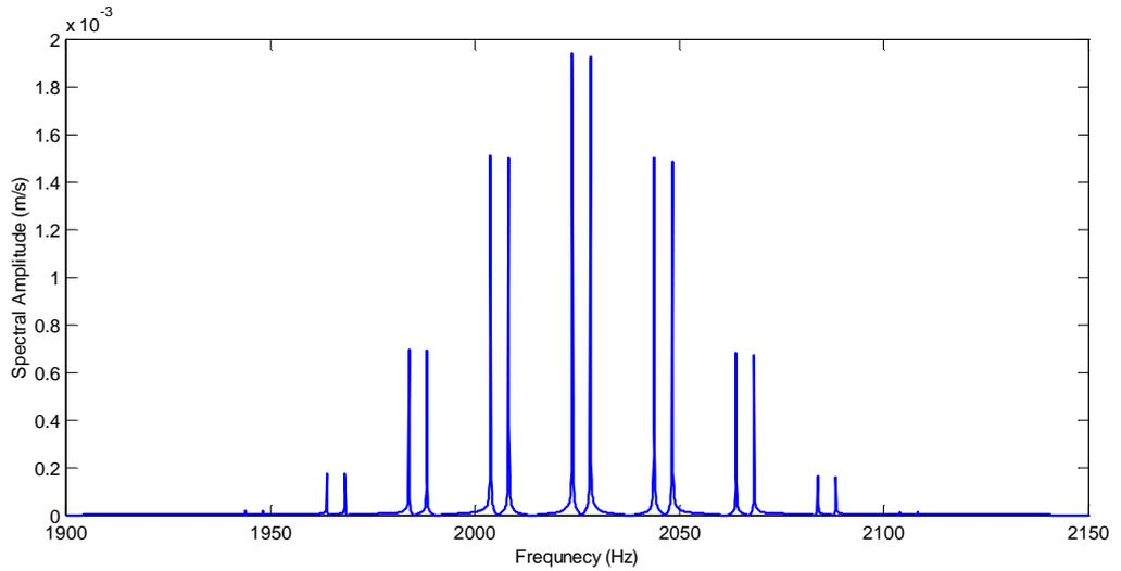
**Figure 5.97** LDV output time history when the laser beam scans in a daisy pattern over the surface of the disc vibrating at the natural frequency of 2026 Hz.
