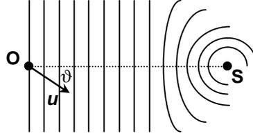
**Figure 2. 2** Doppler effect (Stationary Source-Moving Observer).
