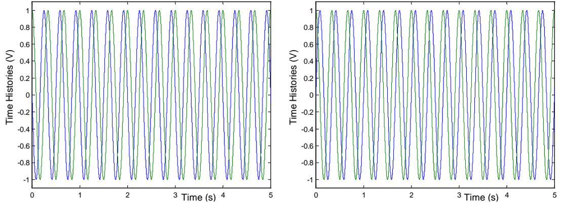
**Figure 2. 24** Doppler signals at the two detectors being the target velocity positive (first) and negative (second).
