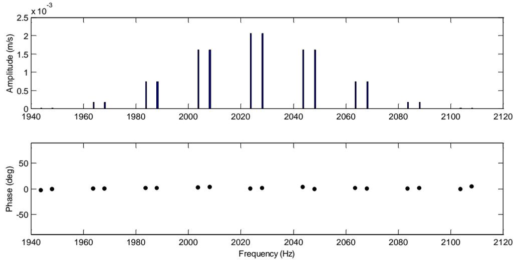
**Figure 5.98** Curve fitted LDV output spectrum in amplitude and phase.
