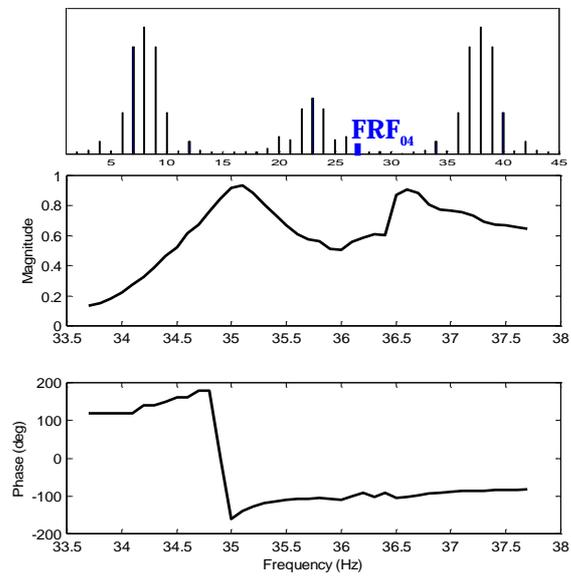
**Figure 5.111** FRF relative to the 4<sup>th</sup> sideband on the central sidebands group in the LDV spectrum ( $n = 0, m = 4$ ) as emphasised in the top diagram.
