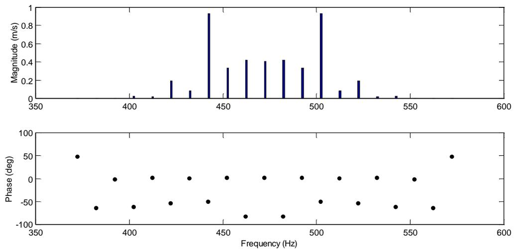
**Figure 5.17** Velocity spectrum.
