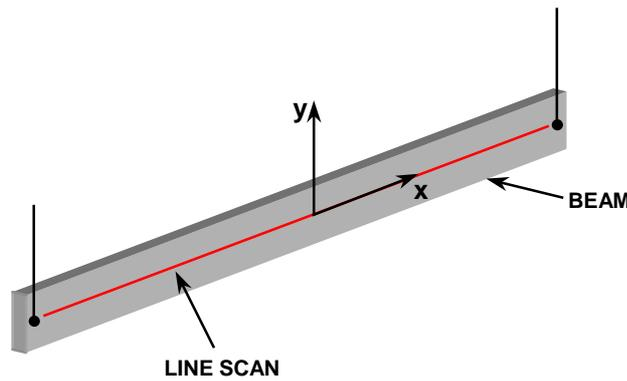
**Figure 5. 1** Laser linear scan on the beam.
