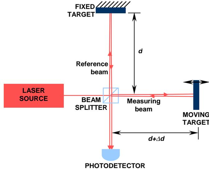
**Figure 2. 16** Schematic representation of Michelson's interferometer.
