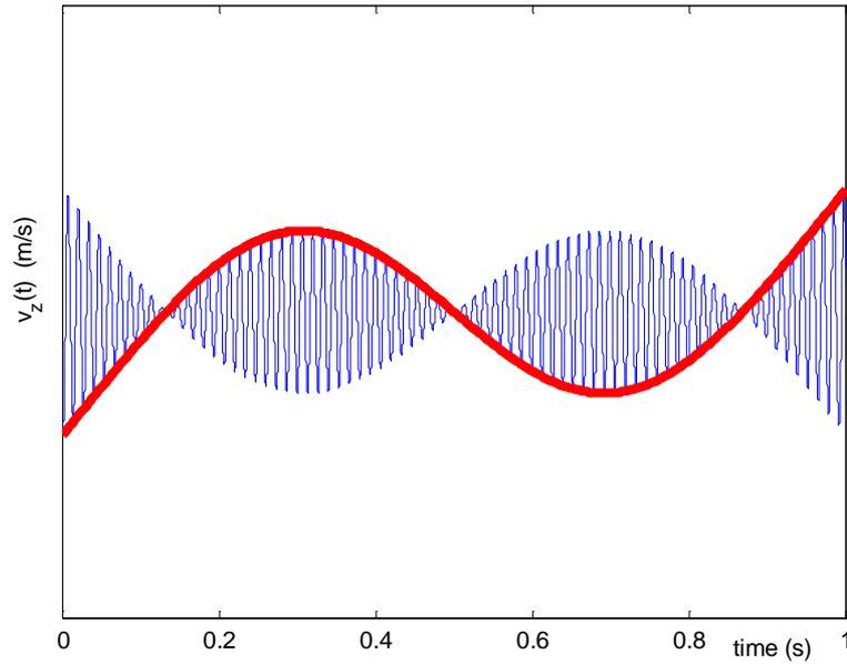
**Figure 5. 3** LDV output modulated by the bending mode shape of the beam (red line).
