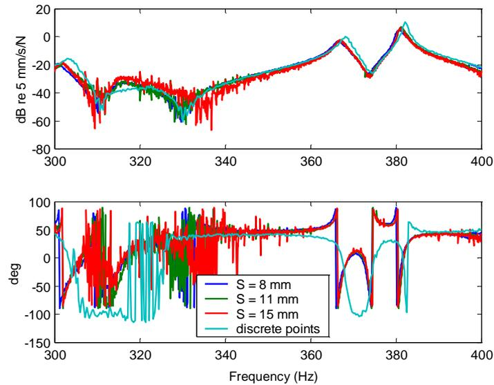
**Figure 7.16** Rotation mobility in  $y$ -direction derived at point 37 by horizontal line scans – amplitude (top) and phase (bottom).
