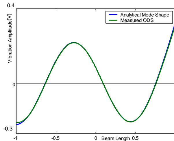
**Figure 5. 27** Analytical mode shape and measured ODS at 766 Hz.
