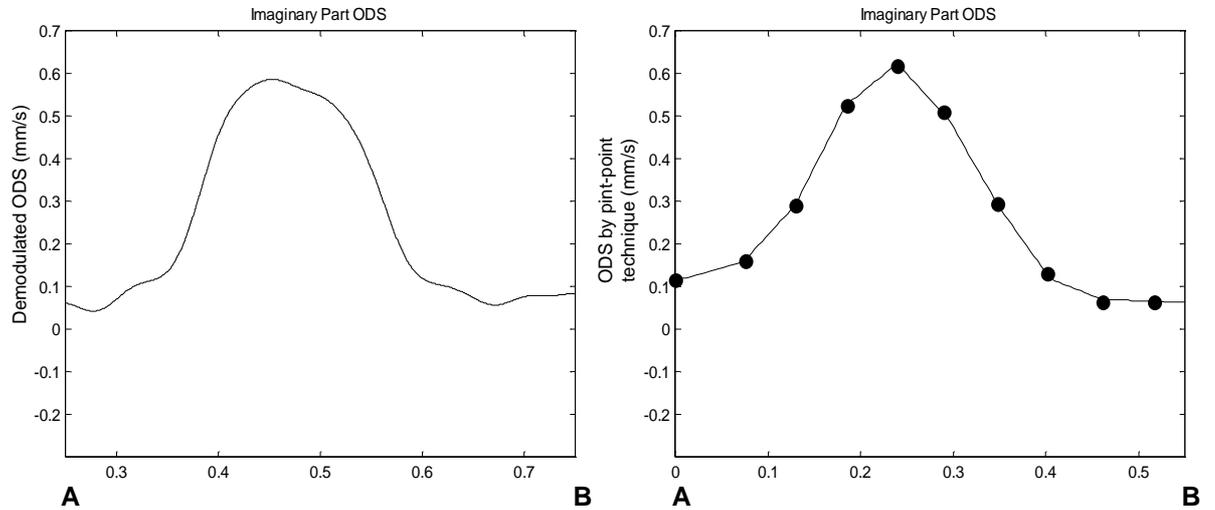
**Figure 7. 37** ODS Imaginary component (mm/s) derived by demodulation (left) and point-by-point scan (right, the vibration response is measured at the marked points only, where the actual measurements have been acquired).
