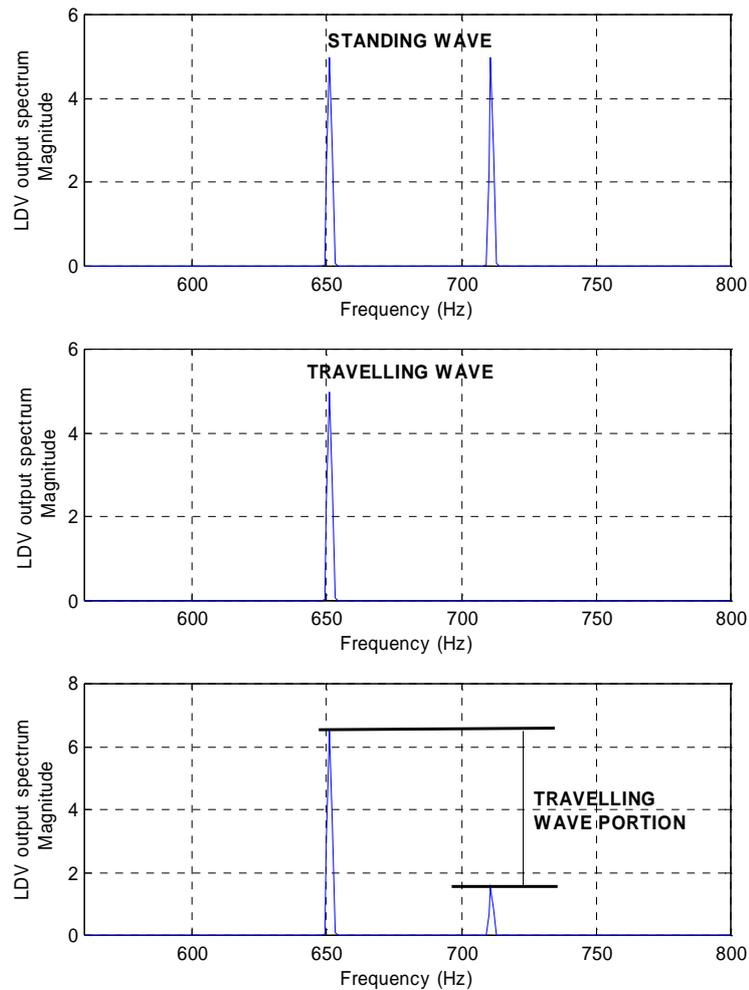
**Figure 5. 41** LDV output spectrum for  $V_{In} = 0$  (top plot),  $V_{In} = V_{Rn}$  (central plot) and  $V_{In} \neq V_{Rn} \neq 0$  (bottom plot).
