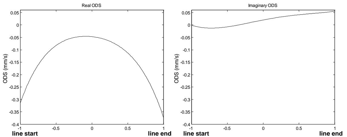
**Figure 7. 49** ODS Real and Imaginary components at the resonance of 142.5 Hz.
