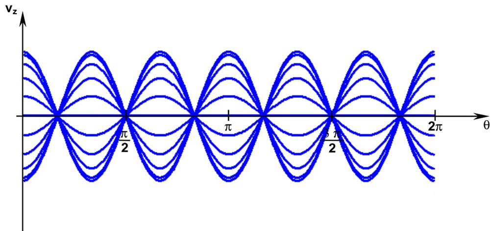
**Figure 5.38** Standing wave on the disc circumference, case of 3-diameter mode.
