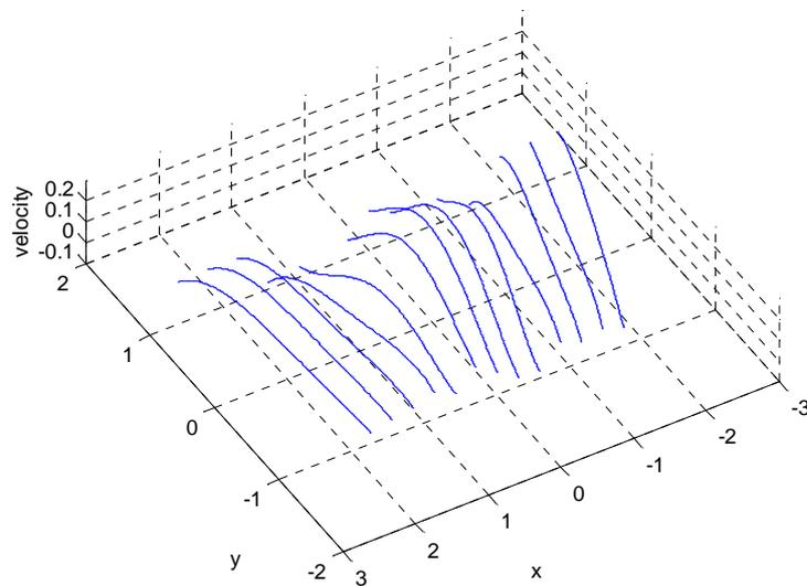
**Figure 7. 50** 2-D ODS at 142.5Hz recovered by raster continuous scanning technique.
