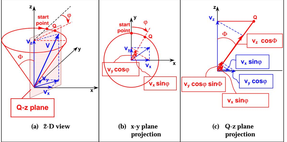
Figure 4. 11 Conical scan configuration.
