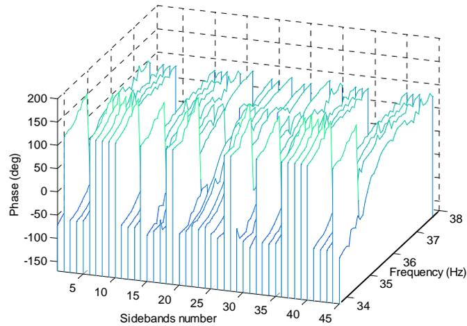
**Figure 5. 116** Waterfall diagram of all the sideband FRFs (phase).
