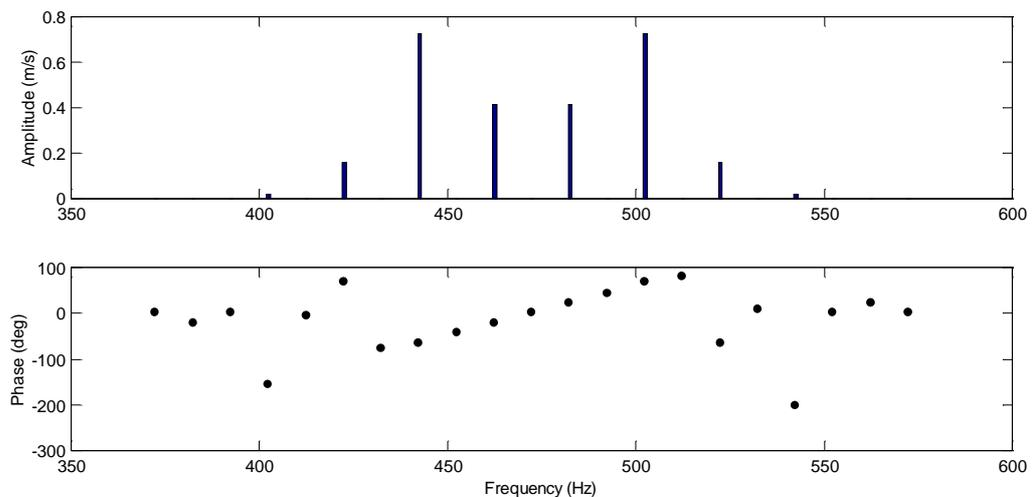
**Figure 5. 20** LDV spectrum in the real situation without considering the mirror delay in the curve-fit.
