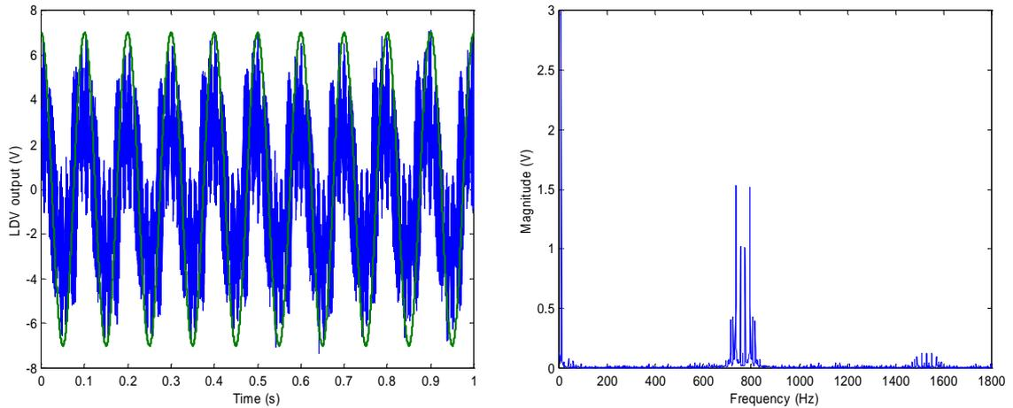
**Figure 6. 23** Measured LDV output spectrum (blue) shown together with the mirror driver signal (green) in the left-hand plot and LDV output spectrum magnitude in the right-hand – Resonance frequency at 766 Hz.
