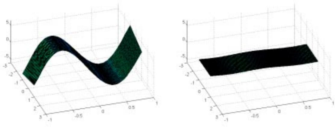
**Figure 5.127** Real and imaginary ODS at 36.6 Hz.
