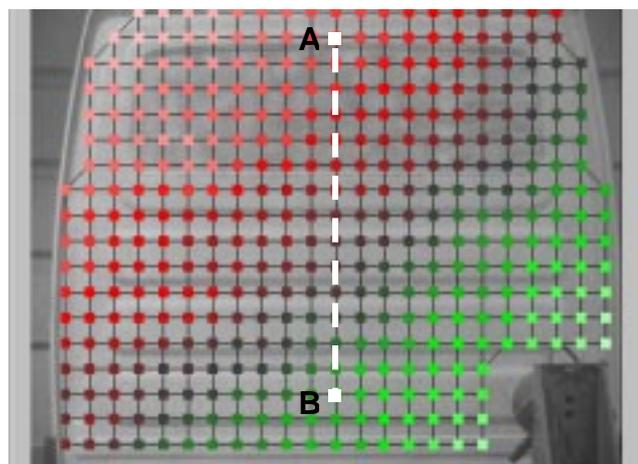
**Figure 7. 27** Line scan superimposed to the grid of points used in the point-by-point technique.
