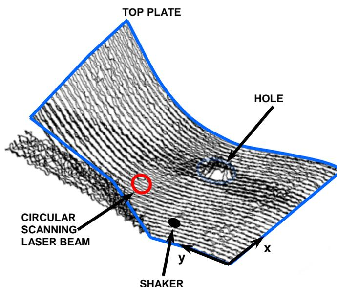
**Figure 7. 6** Plate bending mode and circular scan location.
