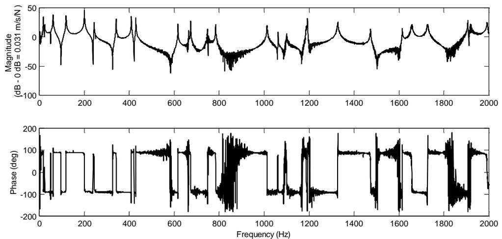
**Figure 5. 53** Transfer FRF at point A on the plate.
