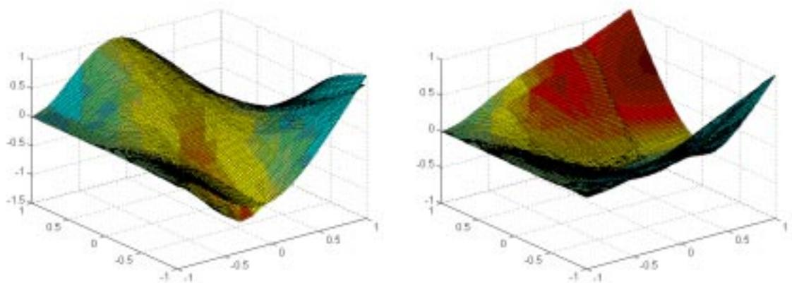
**Figure 3. 10** Measured and theoretical ODSs overlaid for mode 4<sup>th</sup> (left) and mode 5<sup>th</sup> (right).
