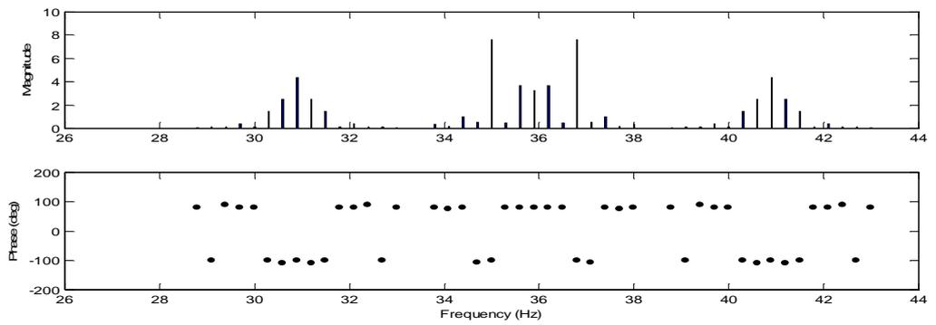
**Figure A. 29** Sideband FRF at the excitation frequency of 35.9 Hz.
