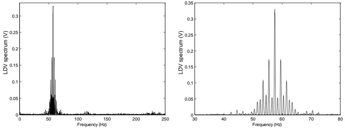
**Figure 7.39** CSLDV output spectrum and its zoom around the excitation frequency 57.5 Hz.
