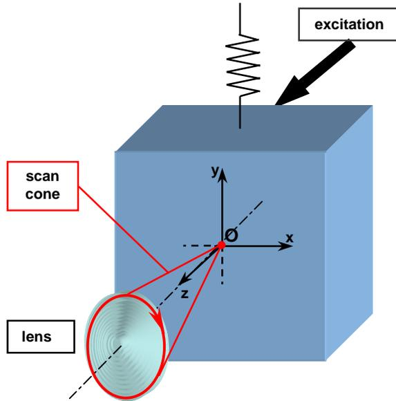
**Figure 4. 12** Conical scan set up.
