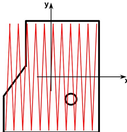
Figure 7. 52 Scanned area over the plate surface.
