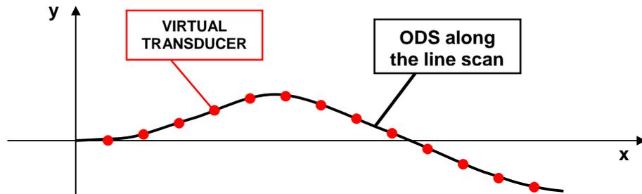
**Figure 1. 1** Virtual transducers location along the laser beam scan line.
