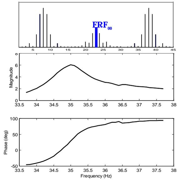
**Figure 5.110** FRF relative to the central component of the LDV spectrum ( $n = 0, m = 0$ ) as emphasised in the top diagram.
