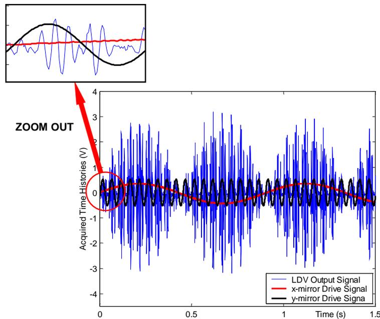
**Figure 5. 74** Measured time signals and zoom on the acquisition initial time instant which shows that the trigger signal employed is the x-mirror driver signal (red line).
