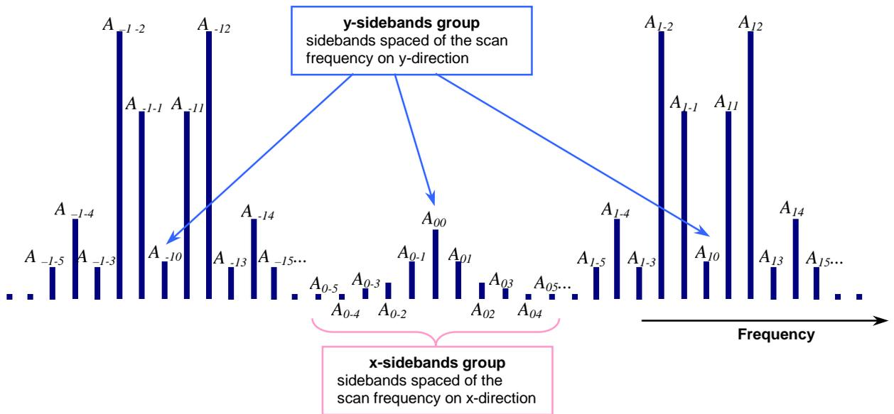
**Figure 5. 62** Association between the LDV spectral amplitudes and the sideband matrix components.
