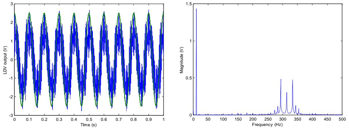
**Figure 6. 17** Measured LDV output spectrum (blue) shown together with the mirror driver signal (green) in the left-hand plot and LDV output spectrum magnitude in the right-hand – Resonance frequency at 311 Hz.
