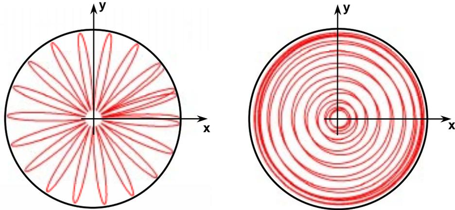
**Figure 5. 90** Laser beam pattern on a disc-like component for circumferential speed (1.1 Hz) lower than the radial (20 Hz) (left), and vice versa (right).
