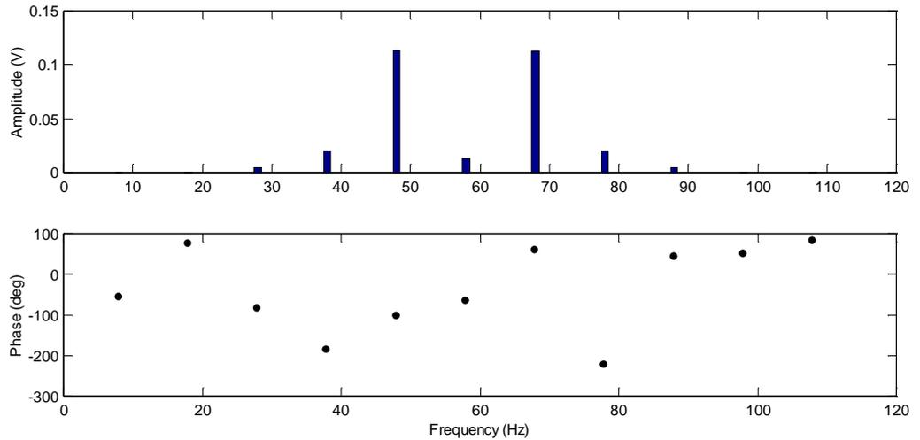
**Figure 5.23** LDV output spectrum without considering the mirror delay.
