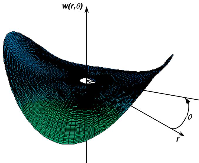
**Figure 5. 93** Mode shape of the disc with two nodal diameters and one nodal circumference.
