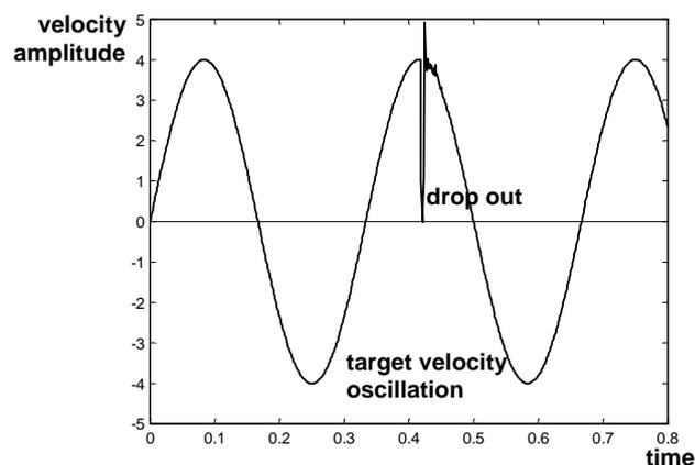
**Figure 2. 7** Velocity Drop out.
