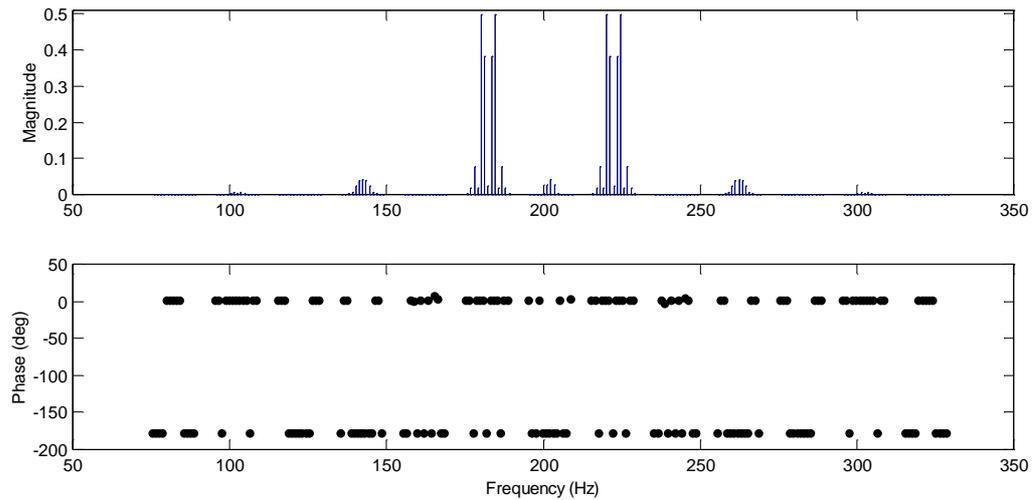
**Figure 5.70** LDV spectrum in the real situation considering the mirror delay.
