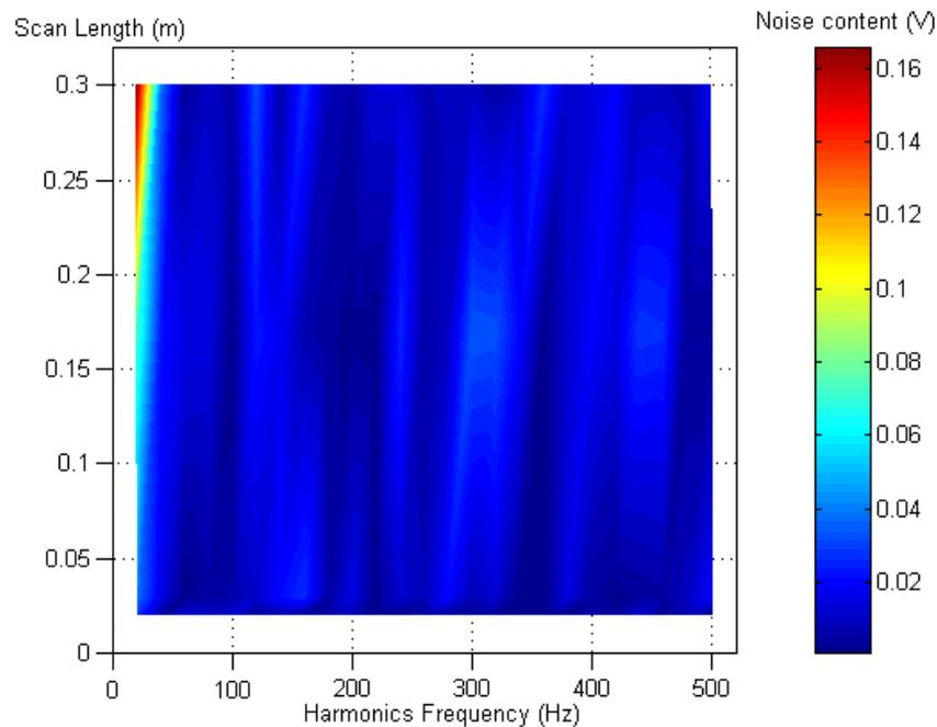
**Figure 6.8** Color-map of the speckle noise level simultaneously plotted against the scan length and the scan frequency and its harmonics.
