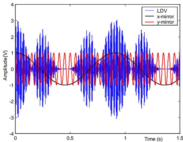
**Figure 5.58** Simulated time histories of the velocity response, together with the time-dependent position of the laser beam on the plate.
