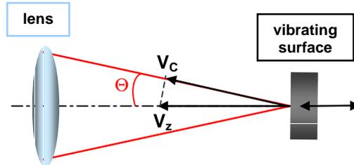
**Figure 4. 30** Conical scan configuration.
