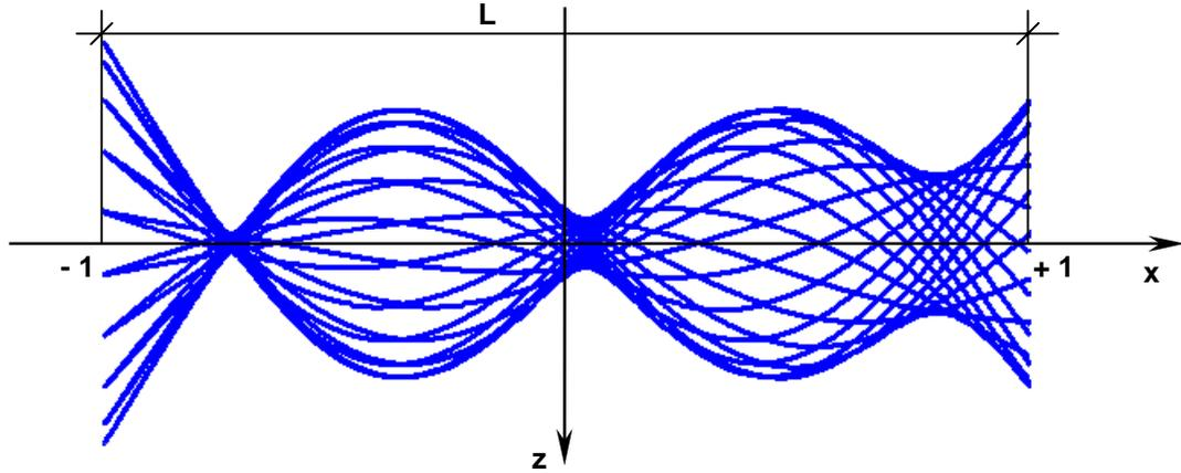
**Figure 5. 15** Vibration pattern at different time instants.
