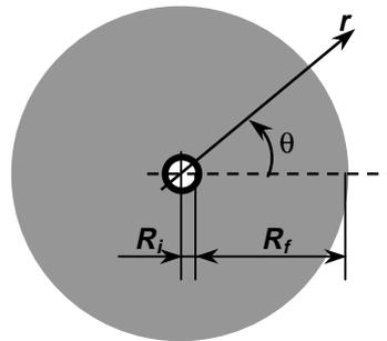
**Figure 5. 91** Annular disc clamped on inside and free on outside.
