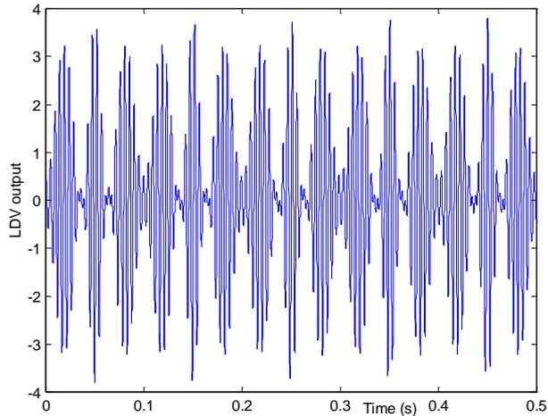
**Figure 5. 34** LDV time history modulated by the circumferential mode shape.
