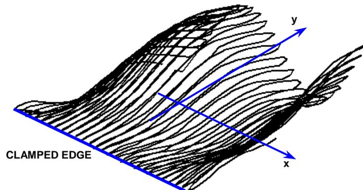
**Figure 5. 55** ODS from demodulation of the LDV output signal with the laser beam scanning at uniform rate across the plate surface.
