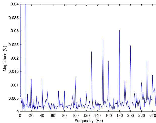
**Figure 6. 18** Zoomed LDV output spectrum in the low-frequency range to emphasize the harmonics of the scan frequency (10 Hz).
