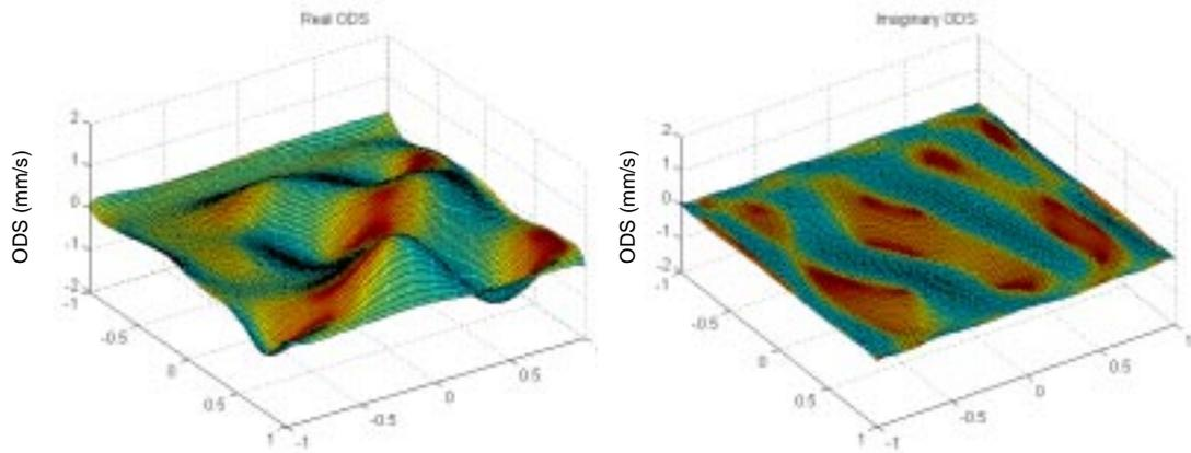
**Figure 7. 65** Real and Imaginary ODS at 191.3 Hz.
