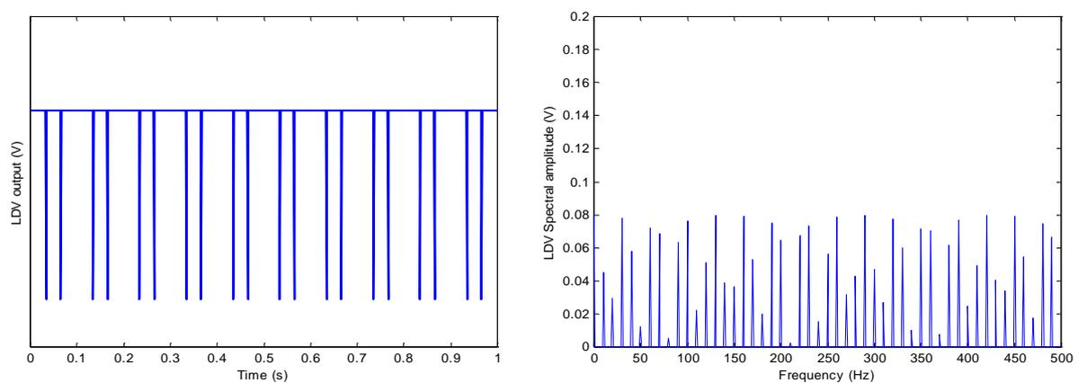
**Figure 6.9** Simulated LDV output time signal showing drop-outs and corresponding Fourier spectrum.
