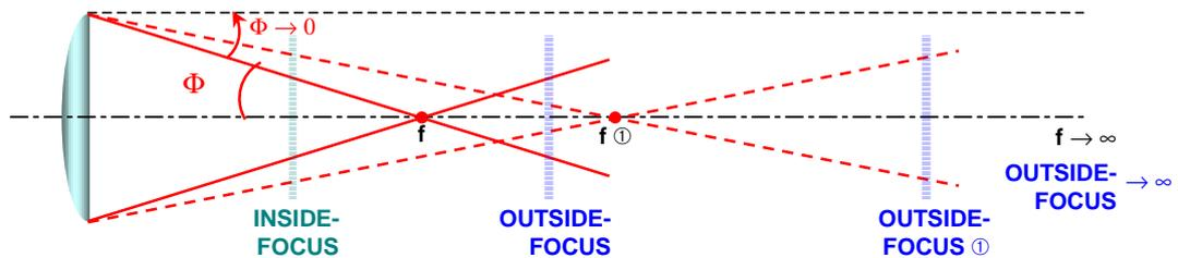
**Figure 4.23** Conical-circular scan degeneration for  $\Phi$  going to zero.
