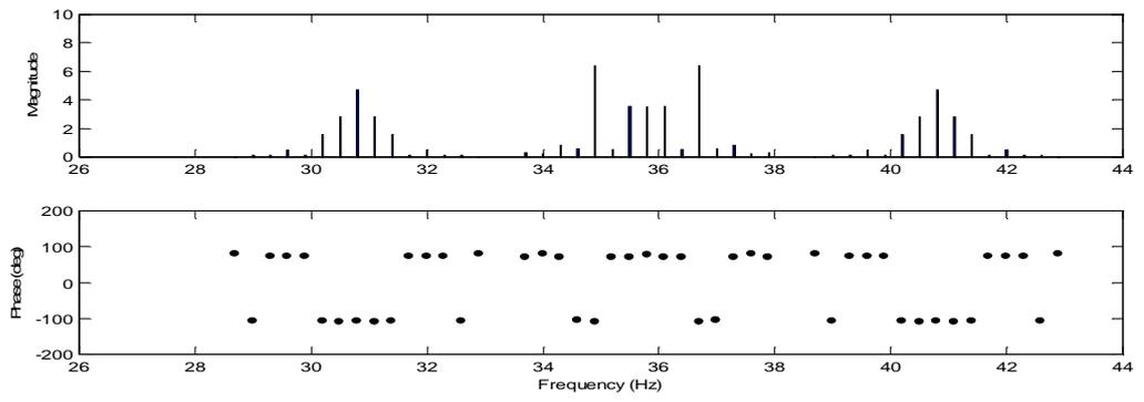
**Figure A. 28** Sideband FRF at the excitation frequency of 35.8 Hz.
