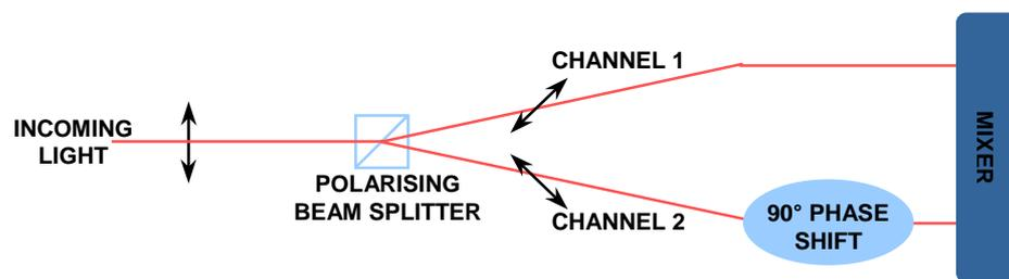
**Figure 2. 19** Schematic of the optical light split and phase shift between the two channels and the mixing of the two outputs after a second phase shift.
