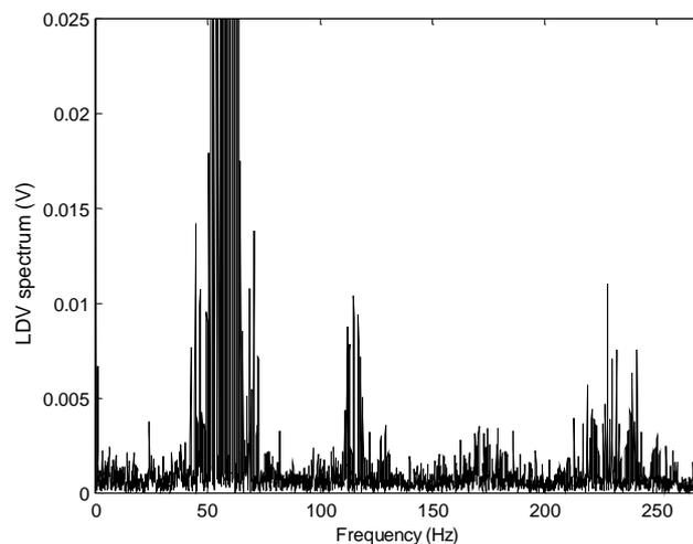
**Figure 7.40** CSLDV output spectrum noise content.
