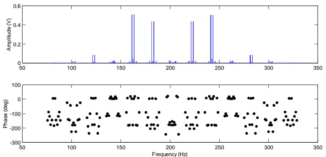
**Figure 5.82** Amplitude and Phase spectrum of the LDV output obtained for imaginary component minimising.
