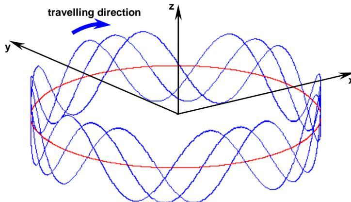
**Figure 5. 40** 2-D view of the travelling wave on the disc circumference.
