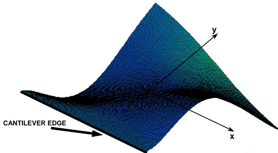
**Figure 5. 80** Plate ODS real component.
