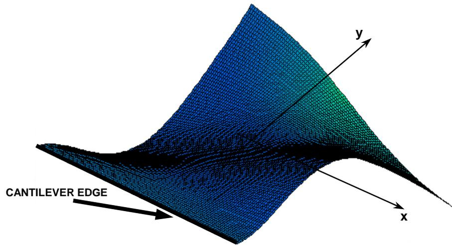
**Figure 5. 65** Real components of the recovered ODS.
