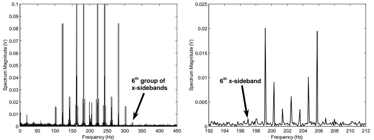
**Figure 5.77** LDV Output Spectrum zoomed in the region of interest (around the excitation frequency). Left plot shows all the  $x$ -sidebands groups (the last visible is the 6<sup>th</sup> one) while right plot is a zoom around the central group where sidebands are important up to the 6<sup>th</sup> only again.
