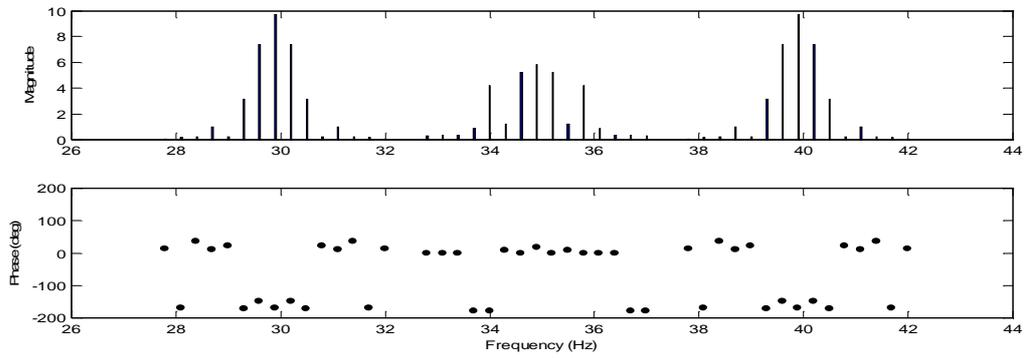
**Figure A. 19** Sideband FRF at the excitation frequency of 34.9 Hz.
