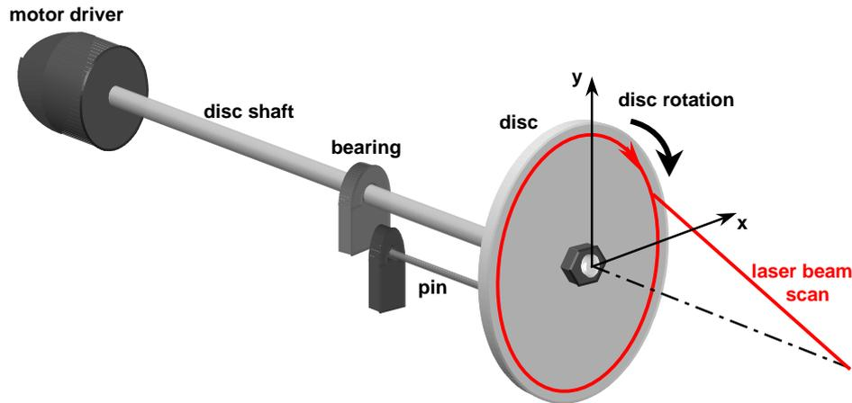
**Figure 5. 48** Pin-on-disc rig – “squeal” excitation.
