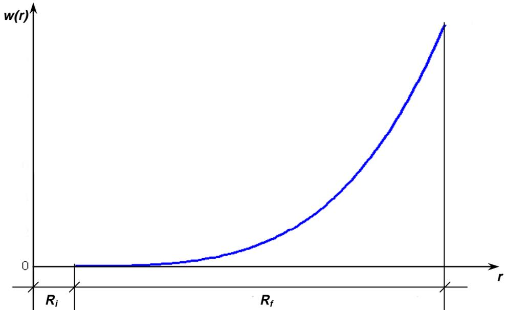
**Figure 5.92** Radial mode shape.
