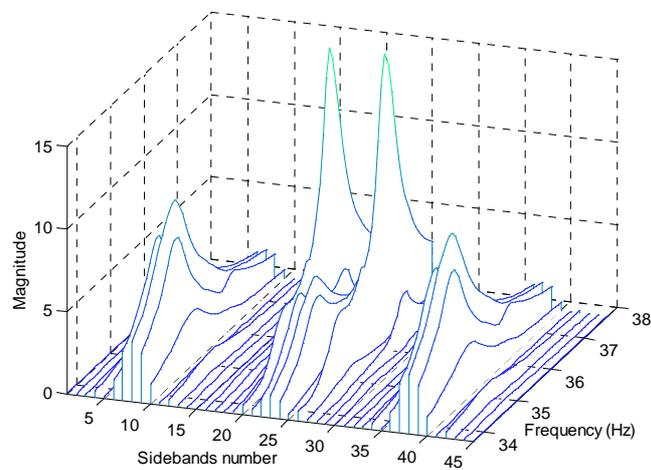
**Figure 5. 114** Waterfall diagram of all the sideband FRFs (amplitude).
