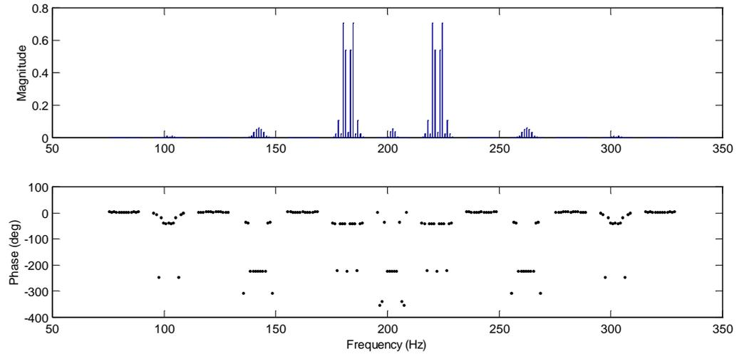
**Figure 5. 64** Magnitude and phase of the LDV output spectrum.
