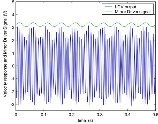
**Figure 4. 8** LDV output and Mirror Drive Signal plotted together.
