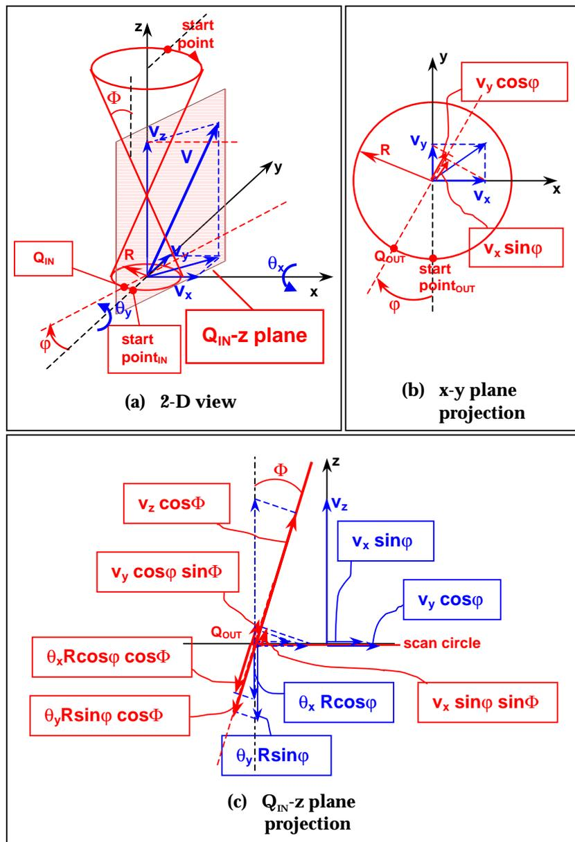
Figure 4.22 Outside-focus conical-circular scan.
