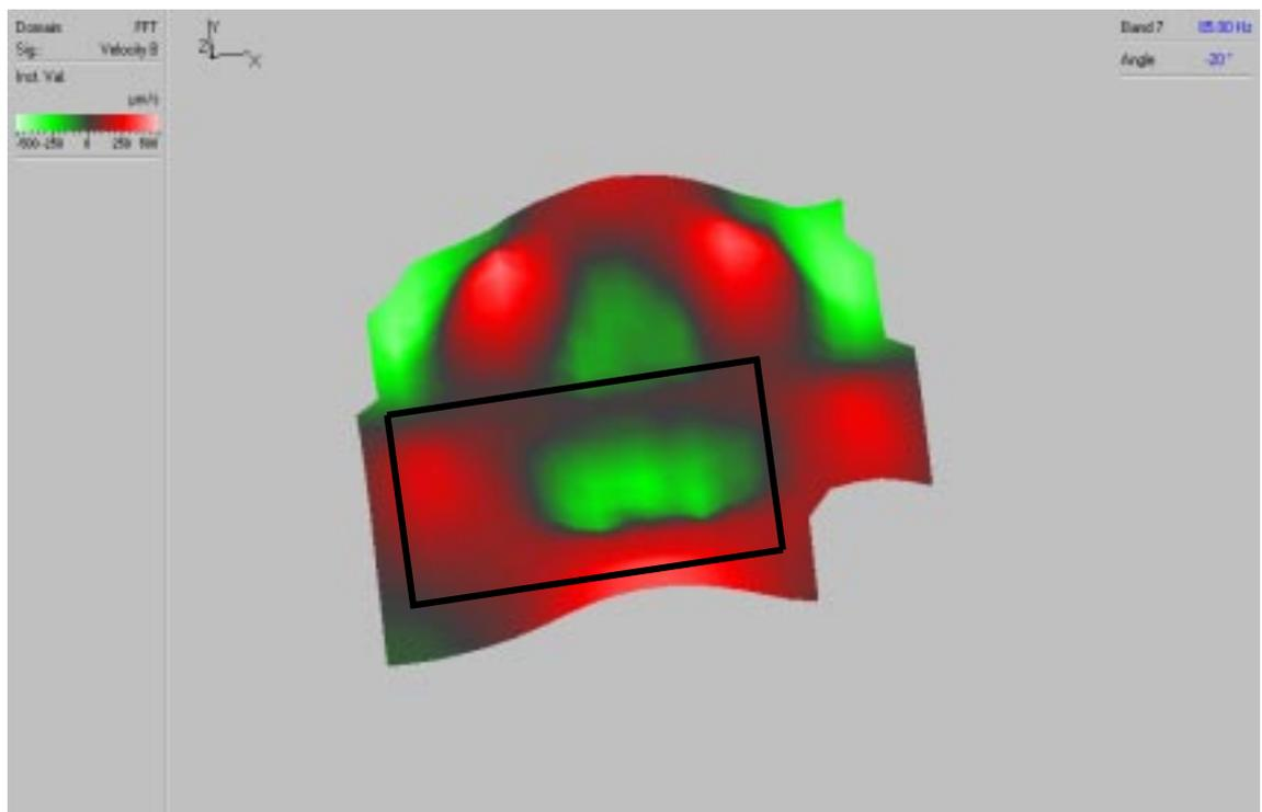
**Figure 7. 60** ODS derived by discrete scan, showing the area where the continuous scan was performed.
