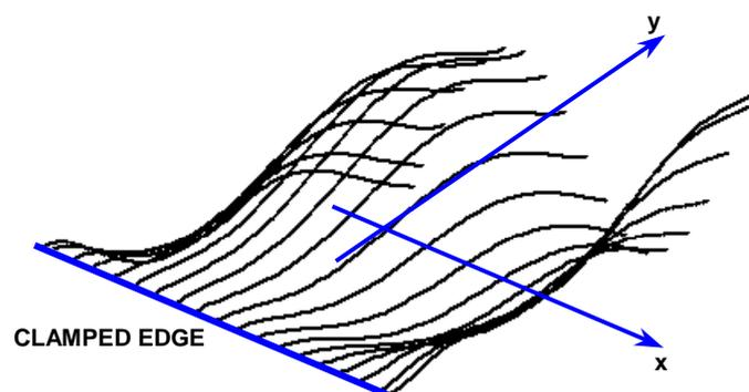
**Figure 5. 56** Polynomial ODSs recovered from the LDV output signal in the frequency domain with the laser beam scanning sinusoidally along a set of parallel straight-lines covering the plate surface.
