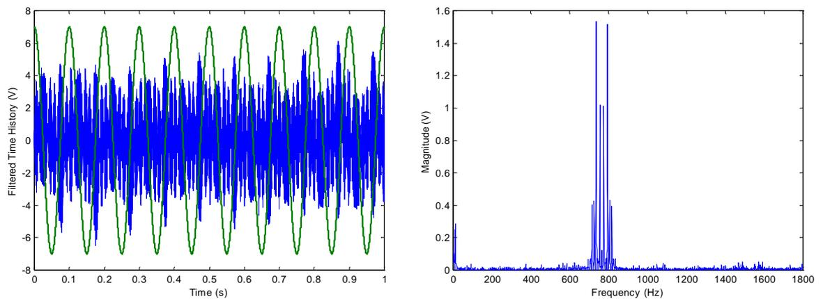
**Figure 6. 24** Time history deprived of the periodic noise (blue) after the averaging process and mirror driver signal (green) in the left-hand plot and its Fourier spectrum in the right-hand – Resonance frequency at 766 Hz.
