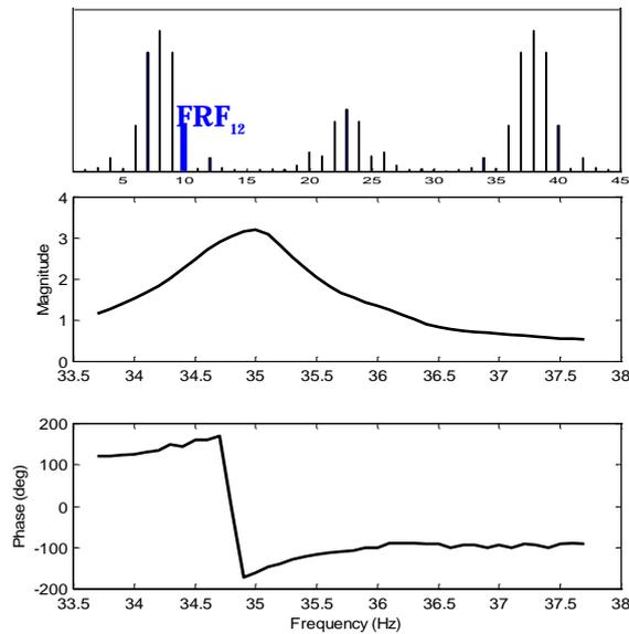
**Figure 5.113** FRF relative to the second sideband of the left sidebands group in the LDV spectrum ( $n = 1, m = 2$ ) as emphasised in the top diagram.
