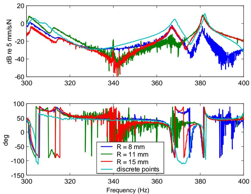
**Figure 7. 18** Rotation mobility in x-direction derived at point 37 by circular scanning – amplitude (top) and phase (bottom).
