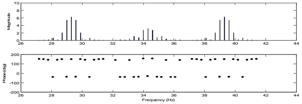
**Figure A. 13** Sideband FRF at the excitation frequency of 34.3 Hz.
