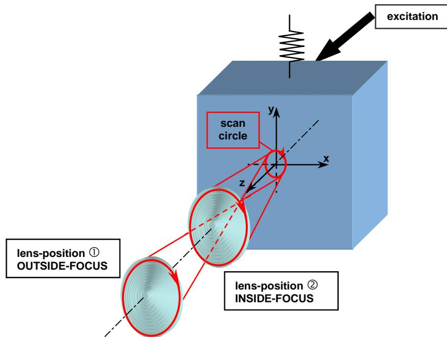
**Figure 4. 24** Conical-Circular scan set-up.
