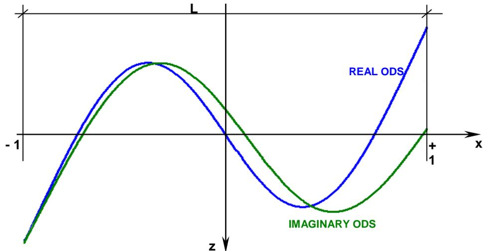
**Figure 5.14** Polynomial description of the real and imaginary components of the vibration.
