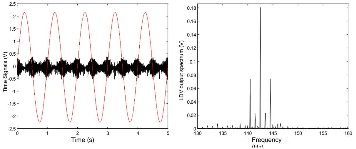
**Figure 7.47** LDV time history (black) and mirror driver signal (red) in the left-hand plot and LDV output spectrum the right-hand plot.
