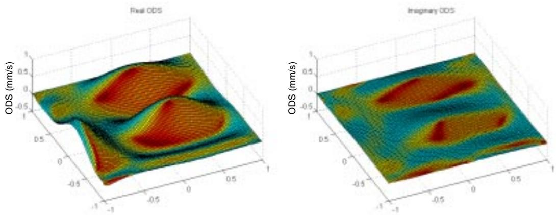
**Figure 7. 63** Real and Imaginary ODS at 146.5 Hz.
