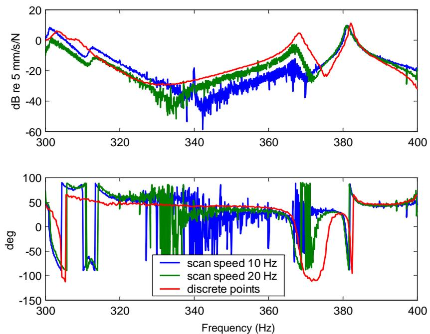
**Figure 7. 21** Rotation mobility in x-direction derived at point 37 by circular scanning- amplitude (top) and phase (bottom).
