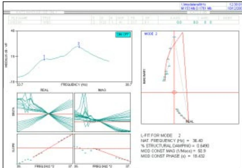
**Figure 5. 122** Modal Analysis by SDOF Line-fit (*ICATS-MODENT*) for  $FRF_{03}$ .
