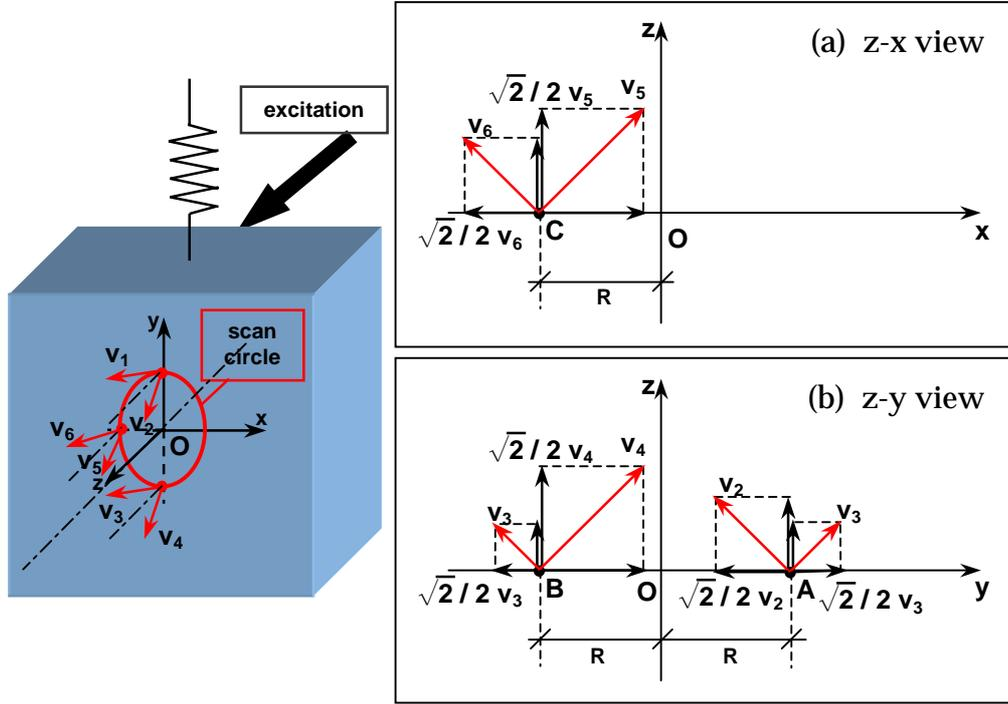
**Figure 4. 25** Single point measurements configuration.
