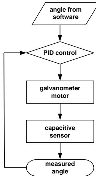
**Figure 3. 2** Flow-chart of the feedback control action.
