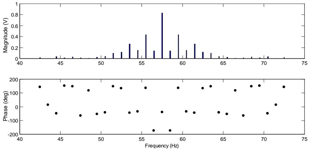
**Figure 7. 42** LDV spectrum magnitude and phase for  $\pm 15$  sidebands.
