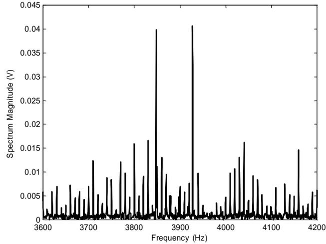
**Figure 5.46** LDV spectrum amplitude (V) at the excitation frequency of 3887.68 Hz. 4-nodal diameter ODS.
