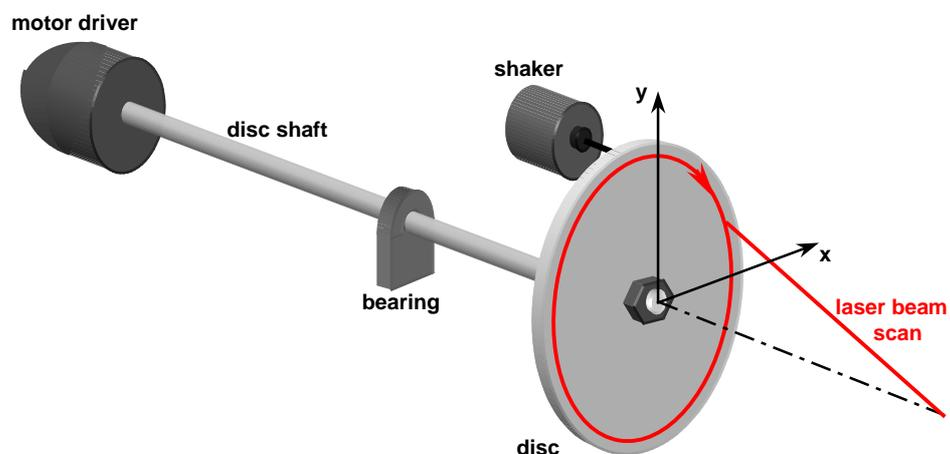
**Figure 5. 42** Disc under direct excitation (pin-on-disc rig).
