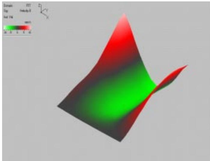
**Figure 3. 7** ODS at 239.1 Hz.
