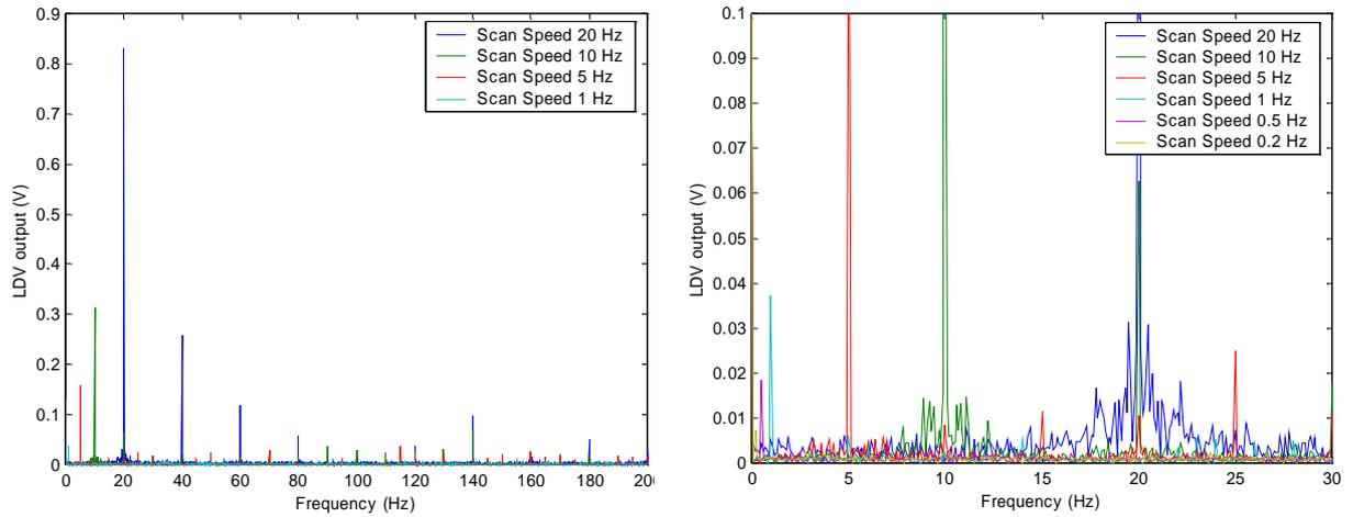
**Figure 6. 3** Measured LDV output spectrum, case of laser beam scanning sinusoidally.
