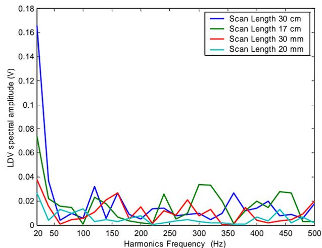
**Figure 6. 7** Speckle noise level plotted against the scan frequency and its harmonics for the different scan length.
