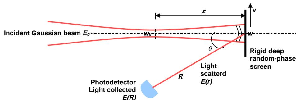
**Figure 2. 6** Light scattering and light collection process.
