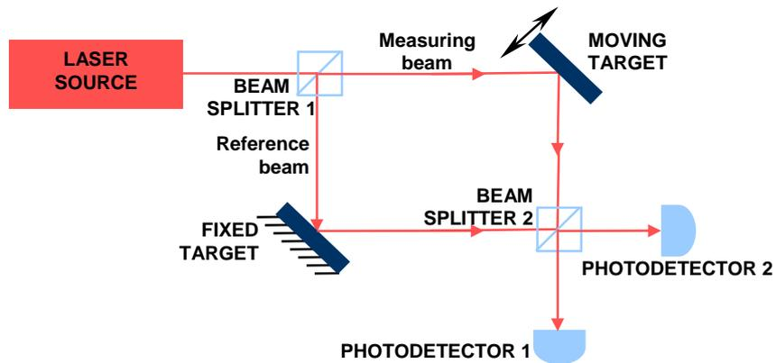
**Figure 2. 17** Schematic representation of Mach-Zehnder interferometer.
