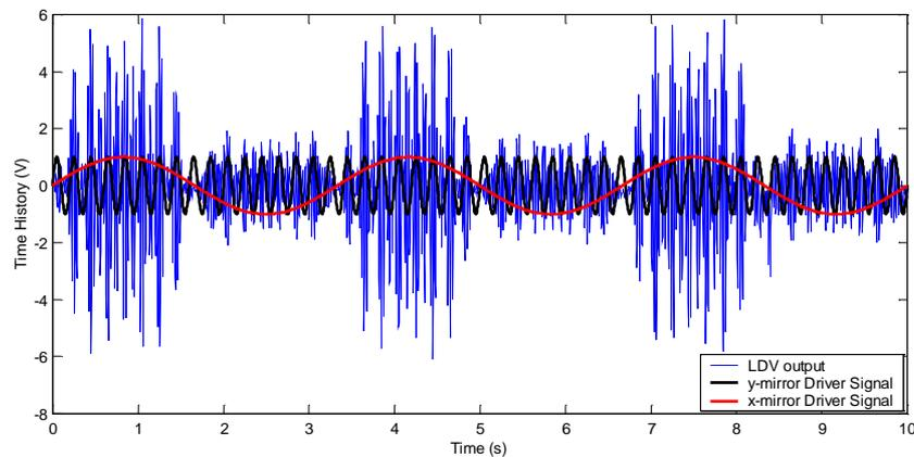
**Figure 5. 107** LDV time-signal obtained by area scan; and  $x$ -axis and  $y$ -axis mirror drive signals.
