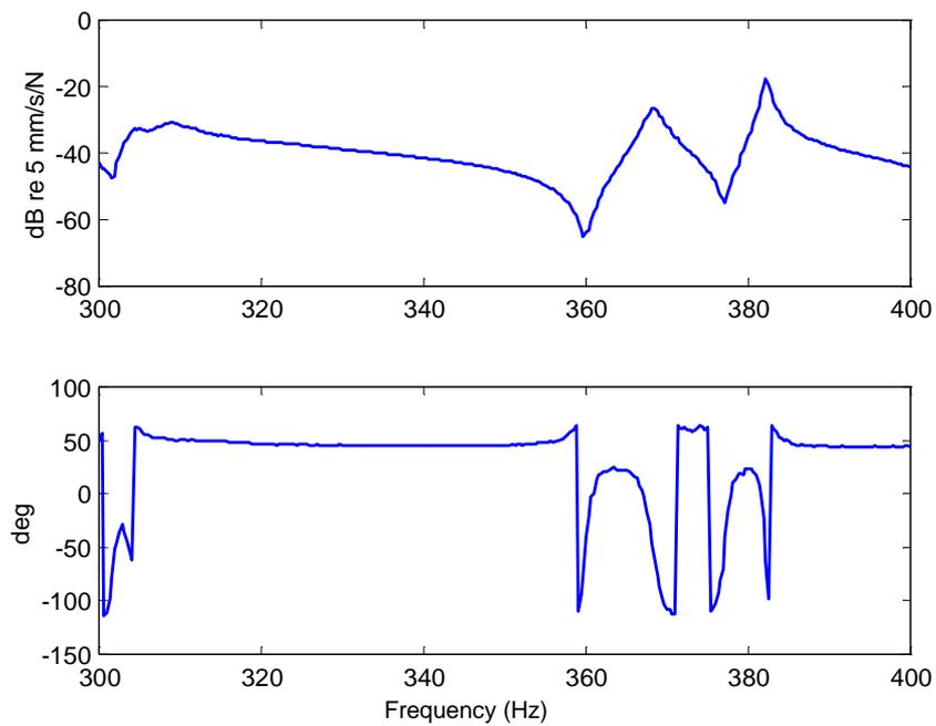
**Figure 7. 11** Translation mobility 37z37z – amplitude (top) and phase (bottom).
