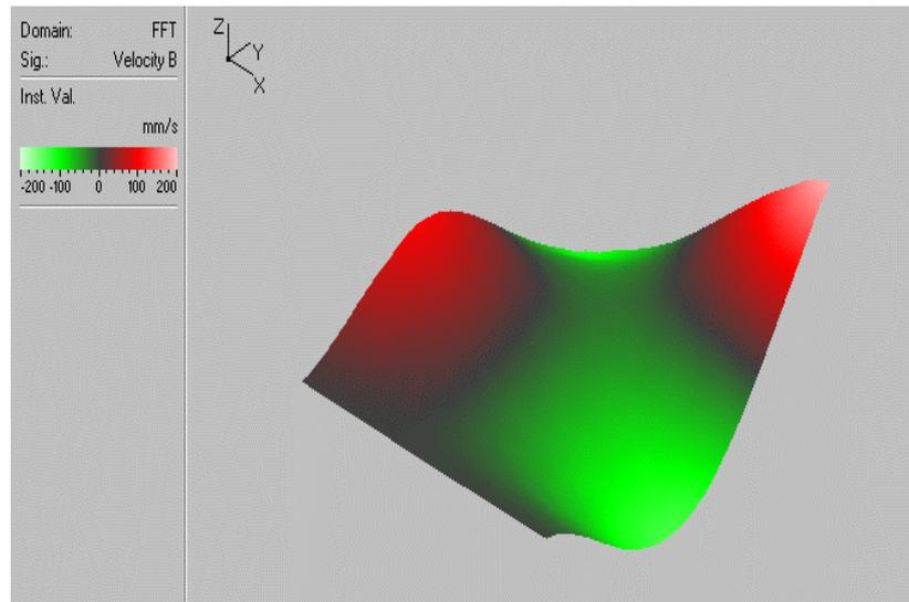
**Figure 3. 11** ODS at 181.9 Hz.
