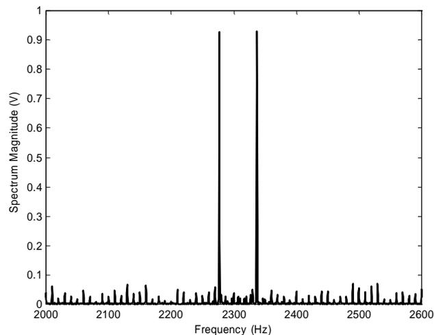
**Figure 5. 45** LDV spectrum amplitude (V) at the excitation frequency of 2307 Hz. 3-nodal diameter ODS.
