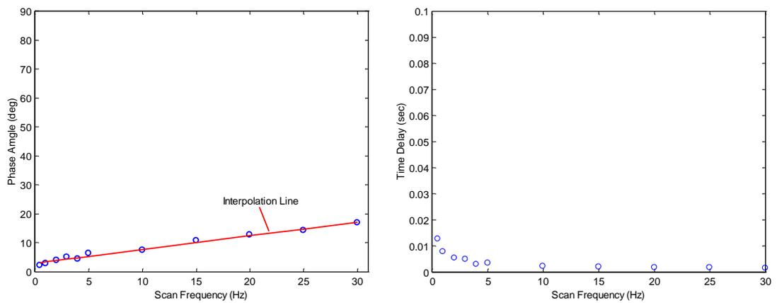
**Figure 4. 27** Phase angles and relative time shifts plotted against the scan frequency.
