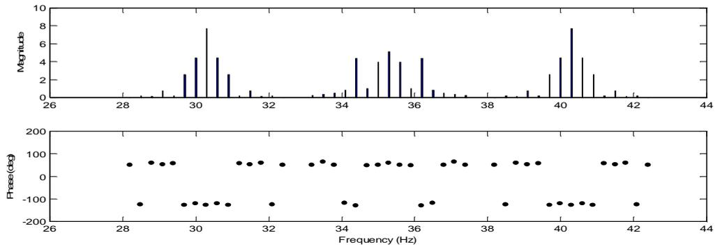
**Figure A. 23** Sideband FRF at the excitation frequency of 35.3 Hz.
