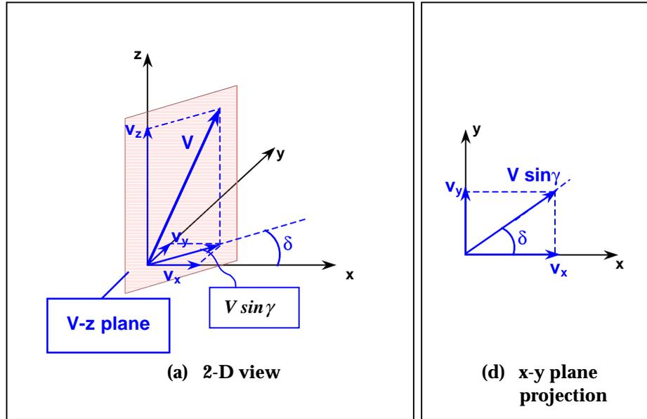
**Figure 4. 14** Cylindrical representation of vibration vector.
