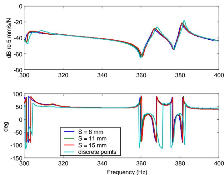
**Figure 7. 15** Translation mobility amplitude and phase derived at point 37 by horizontal line scan with different scan length.
