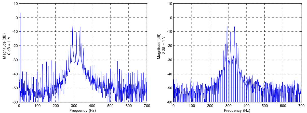
**Figure 6.22** Fourier spectrum amplitude in dB for the original measured signal (left) and the filtered one (right) – Resonance frequency at 311 Hz.
