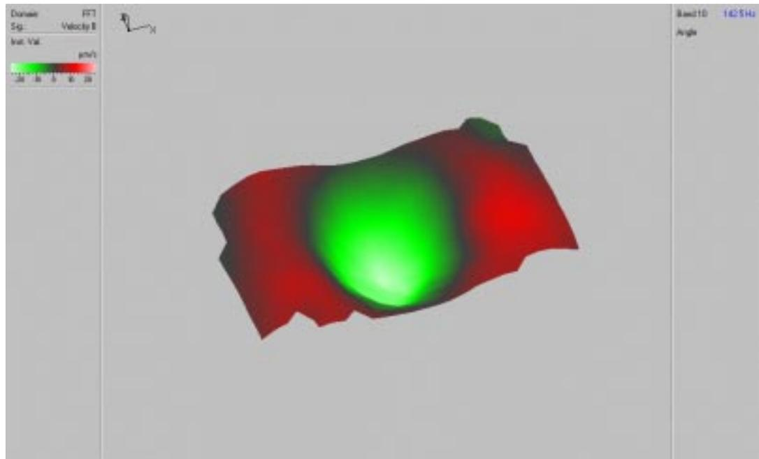
**Figure 7. 51** 2-D ODS at 142.5Hz recovered by single point-by-point scanning technique.
