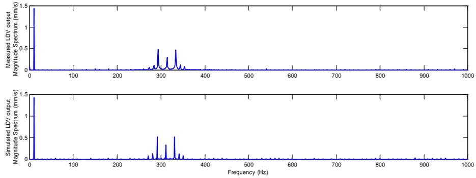
**Figure 6.15** Measured (top) and simulated (bottom) LDV output magnitude spectra.
