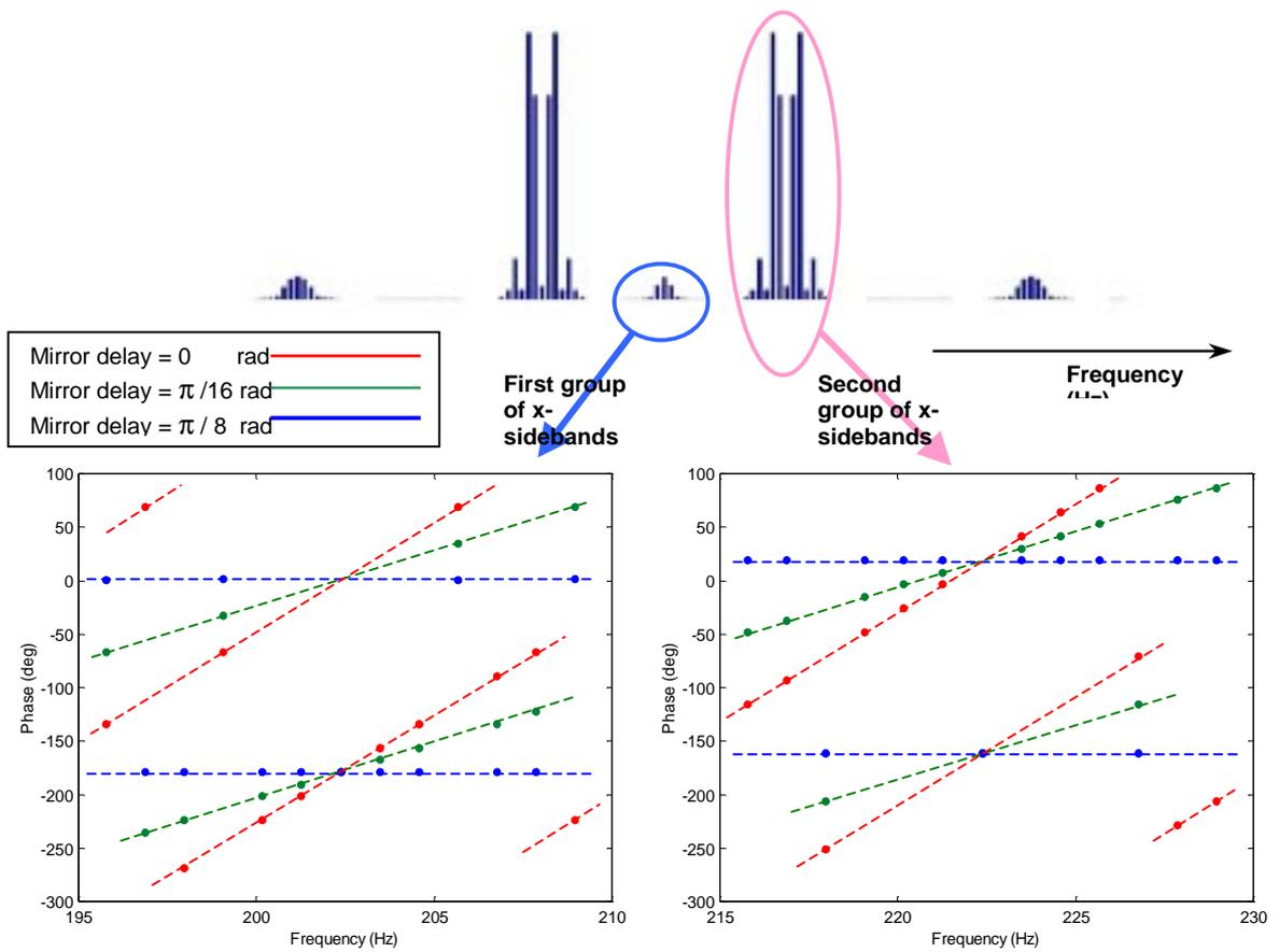
**Figure 5.71** x-group sidebands correction using different values for the mirror delay.
