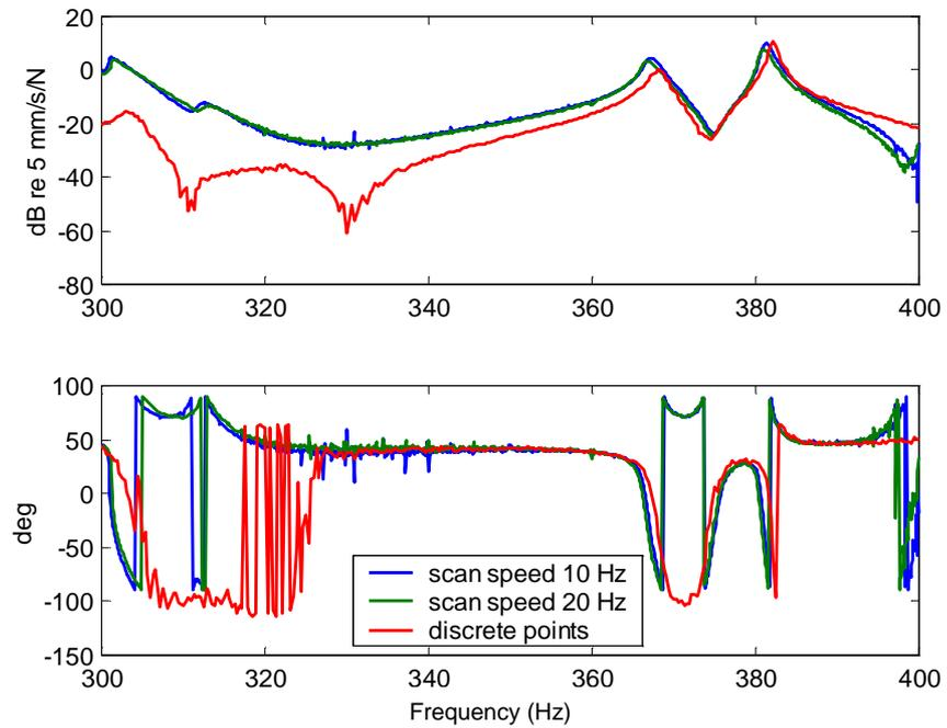
**Figure 7. 22** Rotation mobility in  $y$ -direction derived at point 37 by circular scanning – amplitude (top) and phase (bottom).
