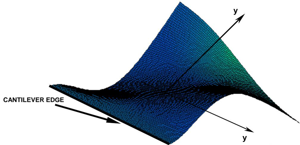
**Figure 5. 57** Analytical mode shape at the natural frequency of 202.4 Hz.
