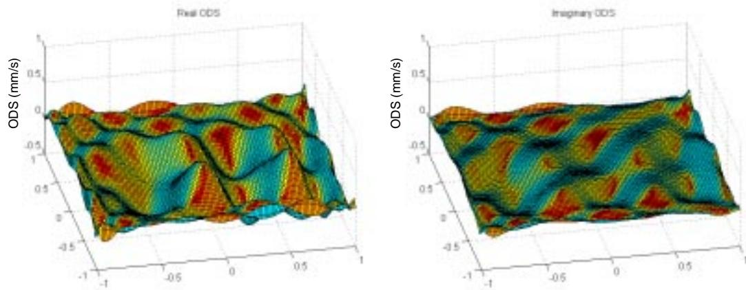
**Figure 7. 67** Real and Imaginary ODS at 230 Hz.
