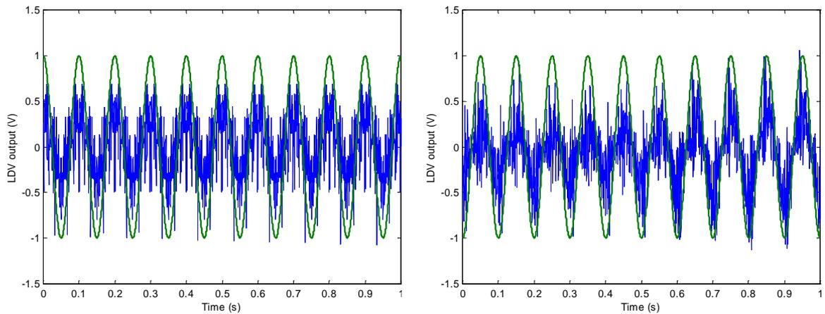
**Figure 6. 11** Simulated (left-hand plot) and measured (right-hand plot) LDV output time histories plotted together with the 10 Hz sinewave.
