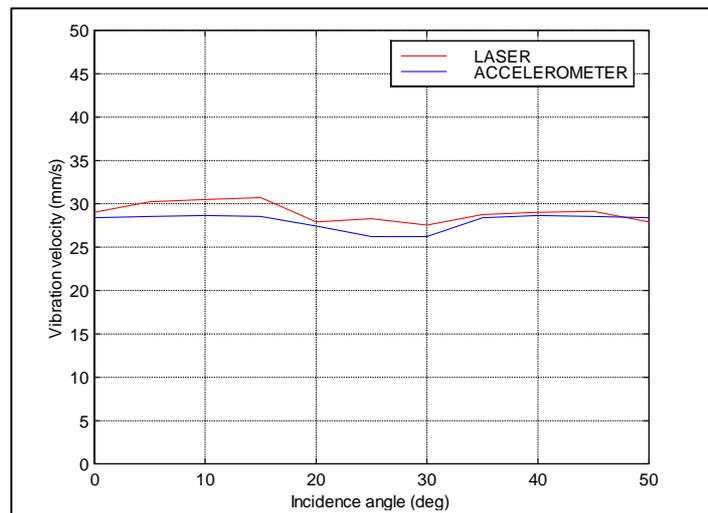
**Figure 4. 16** Vibration velocity amplitude measured with a conical scan LDV and an accelerometer.
