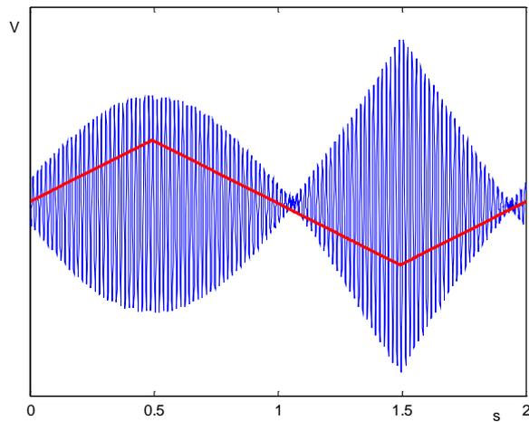
**Figure 5. 4** LDV output signal (blue) and mirror driving signal (red).
