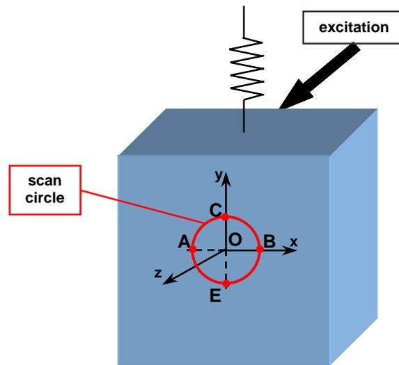
**Figure 4. 10** Circular scan set up.
