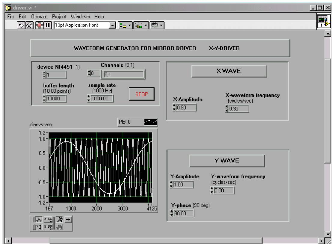
**Figure A. 5** Mirror driver control panel- case of sinewaves.
