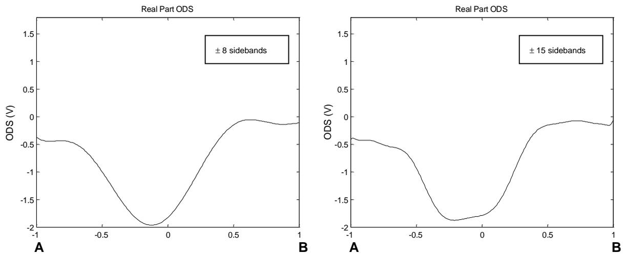
**Figure 7.43** ODS real part derived by polynomial series using 8 (left) and 15 (right) sidebands.
