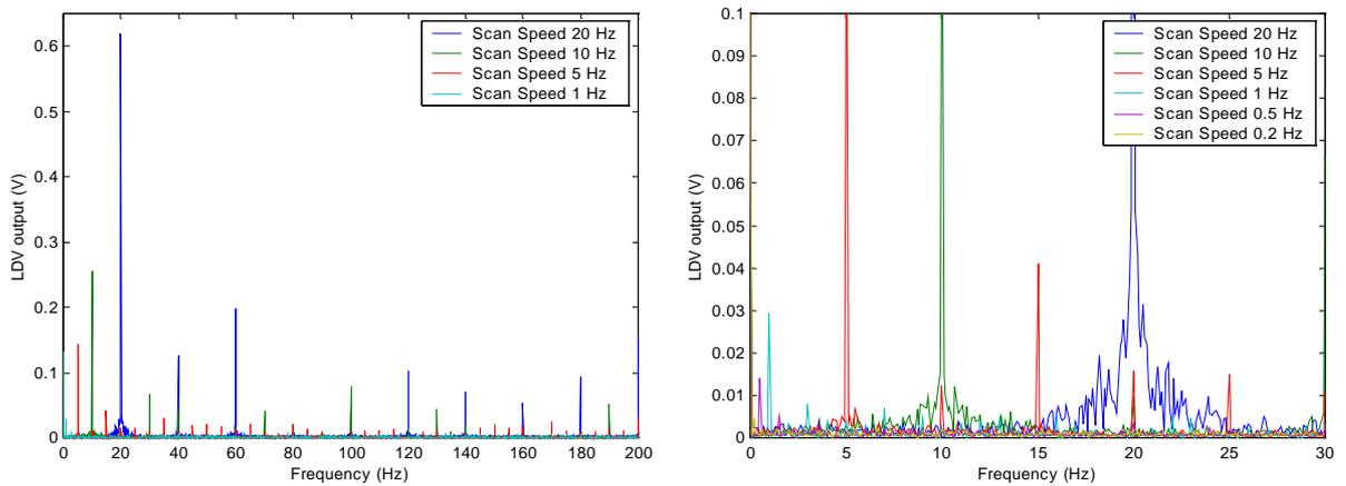
**Figure 6. 5** Measured LDV spectrum, case of laser beam scanning at uniform rate.
