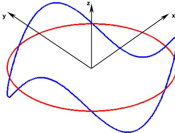
**Figure 5.47** Standing wave along the scanning circle (3-nodal diameter ODS).
