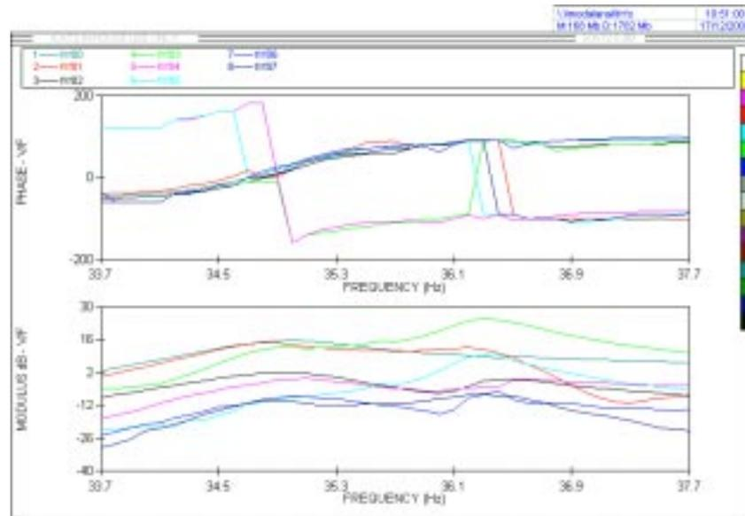
**Figure 5.118** Conventional FRFs analysed by ICATS ( $FRF_{00}$ ,  $FRF_{01}$ , ...,  $FRF_{07}$ ).
