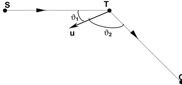
**Figure 2. 3** Doppler effect (Scattering Condition).
