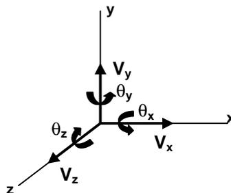
**Figure 4. 1** Vibration decomposition in the Cartesian system of coordinates.
