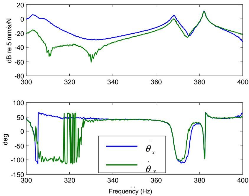
**Figure 7. 12** RDOF mobilities about  $x$ - and  $y$ -direction calculated from translational measurements around point 37 – amplitude (top) and phase (bottom).
