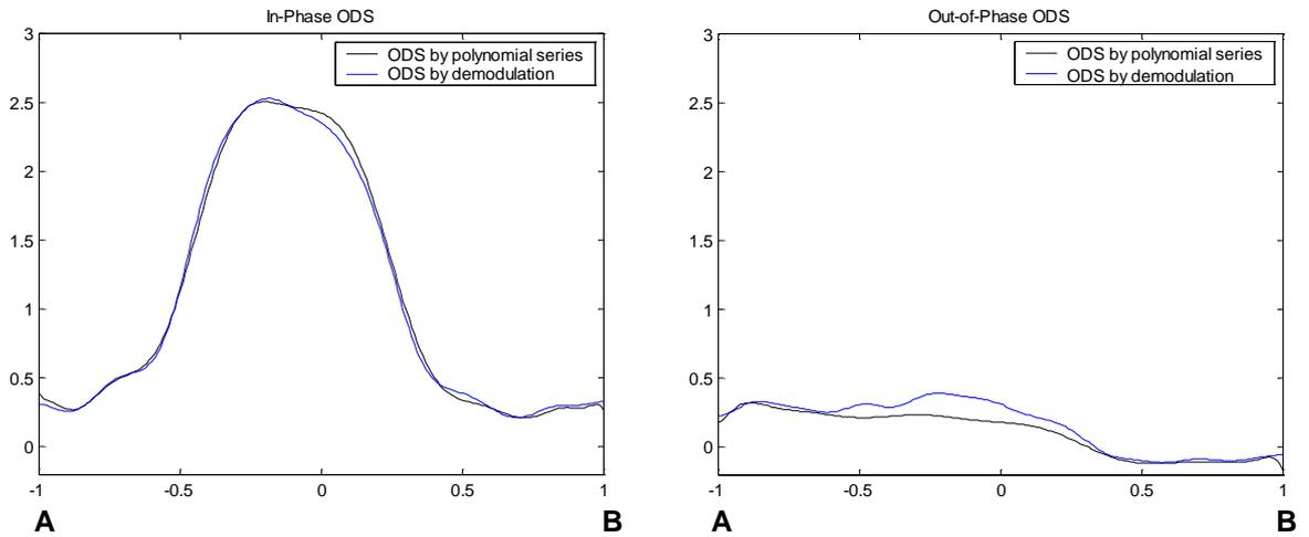
**Figure 7. 45** In-Phase and Out-of-Phase ODS (V) derived by polynomial series ( $\pm 15$  sidebands) and demodulation.
