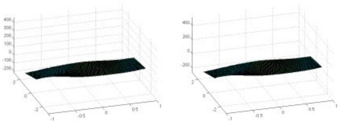
**Figure 5. 125** Imaginary part of the mode shape at the natural frequency of 34.86 Hz derived from original (left) and corrected (right) modal constants.
