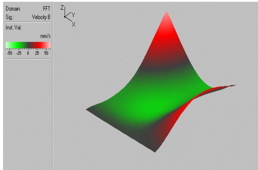
**Figure 3. 12** ODS at 239.1 Hz.
