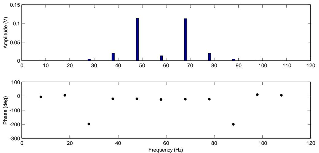
**Figure 5.24** Correct LDV output spectrum.
