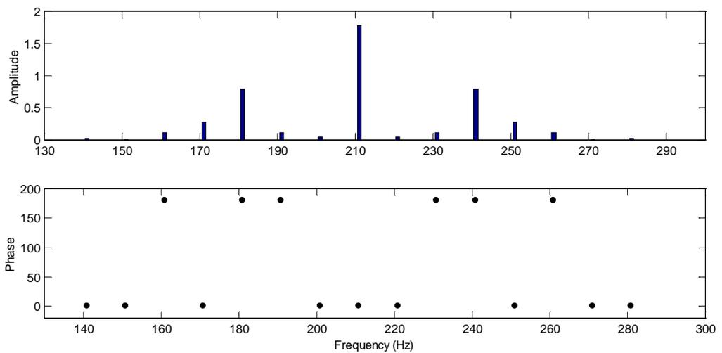
**Figure 5. 35** LDV output spectral components amplitude and phase (°).
