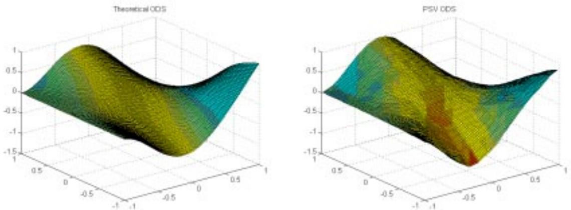
**Figure 3. 8** ODS at 181.9 Hz (4<sup>th</sup> Mode).
