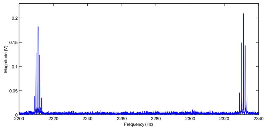
**Figure 5. 103** LDV signal spectrum for the spiral scan and excitation at 2271 Hz.
