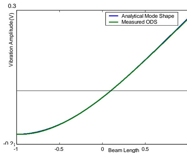
**Figure 5. 25** Analytical mode shape and measured ODS at 58 Hz.
