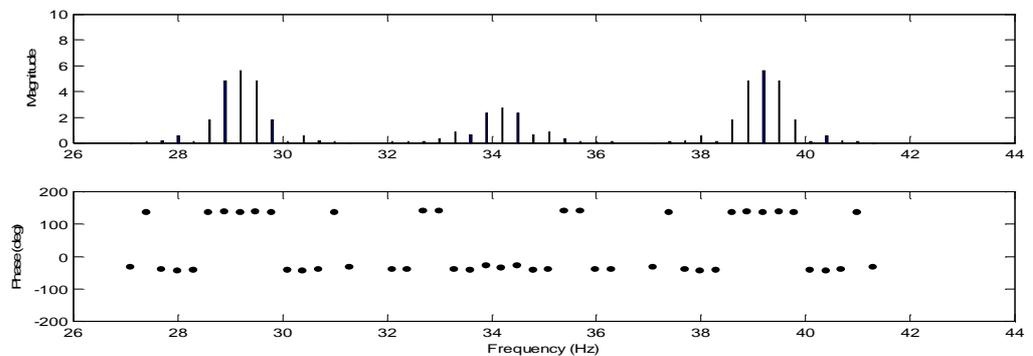
**Figure A. 12** Sideband FRF at the excitation frequency of 34.2 Hz.
