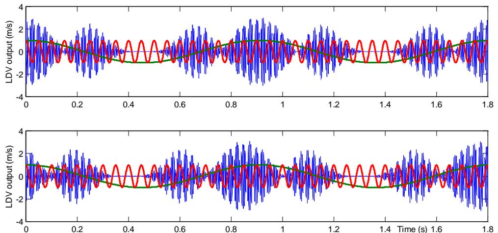
**Figure 5. 67** LDV output signal for the ideal and real situation, considering the delay of the mirrors, which are plotted as well (the  $x$ -mirror is green and the  $y$ -mirror is red).
