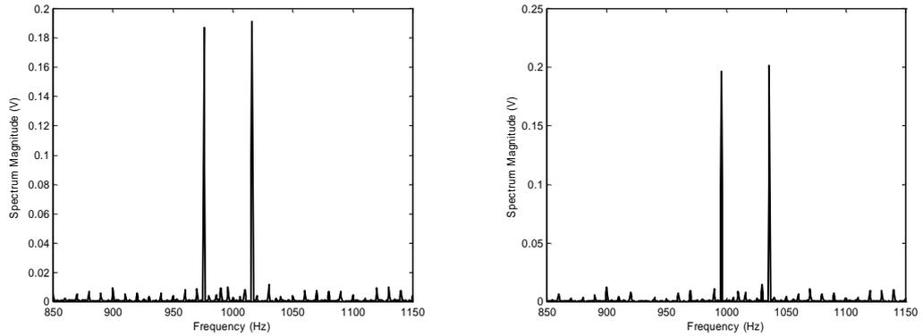
**Figure 5. 44** LDV spectrum amplitude (V) at the excitation frequency of 996 Hz (left) and 1016 Hz (right). 2-nodal diameter ODS.
