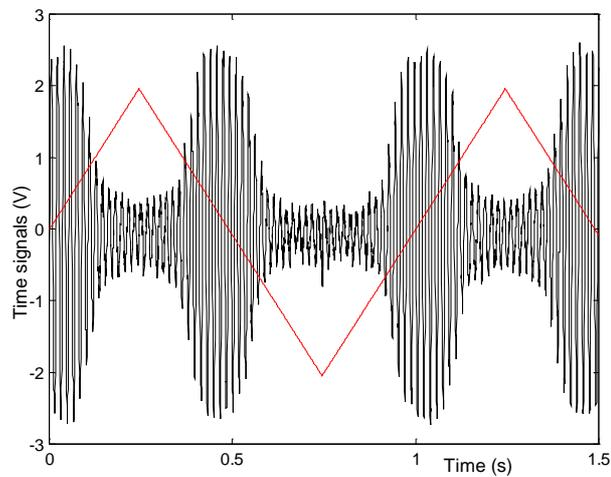
**Figure 7. 34** LDV output time history (V) at 57.5Hz resonant frequency.
