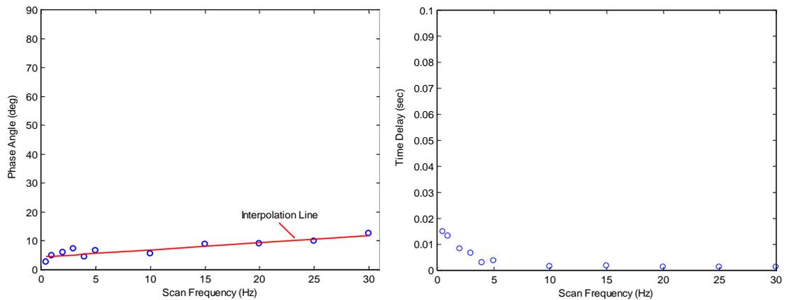
**Figure 4. 28** Phase angles and relative time shifts plotted against the scan frequency.
