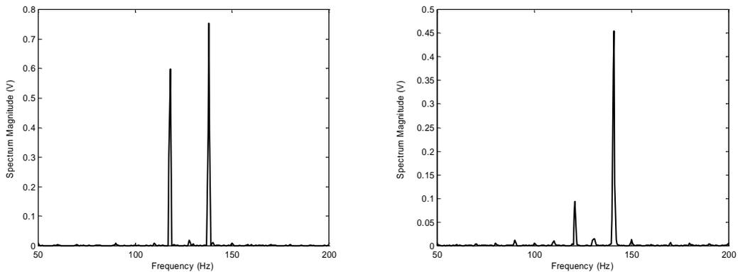
**Figure 5.43** LDV spectrum amplitude (V) at the excitation frequency of 128 Hz (left) and 130.9Hz (right). 1-nodal diameter ODS.
