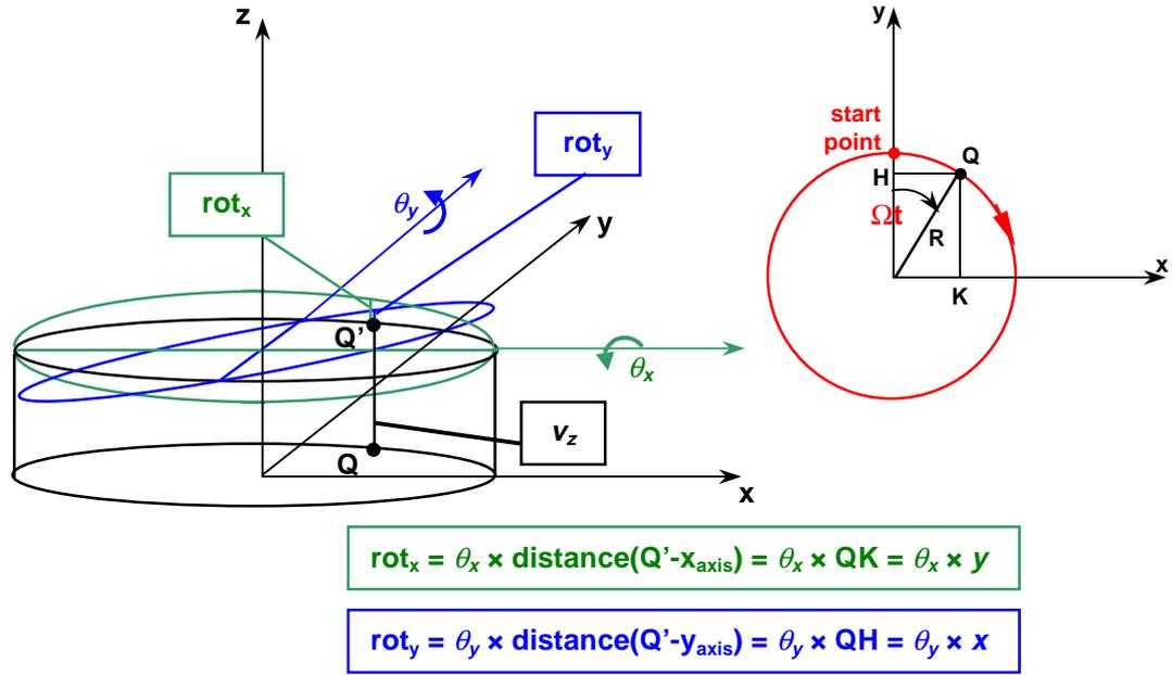
Figure 4. 9 Circular scan configuration.
