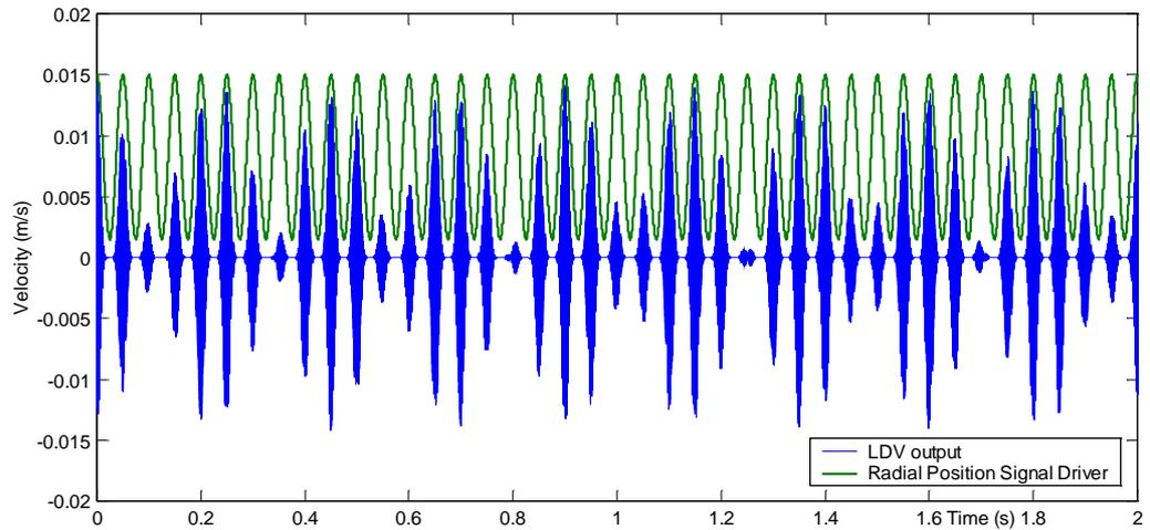
**Figure 5.95** LDV output time history when the laser beam scans in a daisy pattern over the surface of the disc vibrating at the natural frequency of 2026 Hz. The modulation due to the circumferential motion of the laser beam is visible.
