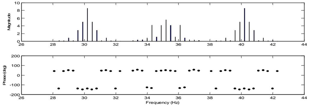
**Figure A. 22** Sideband FRF at the excitation frequency of 35.2 Hz.
