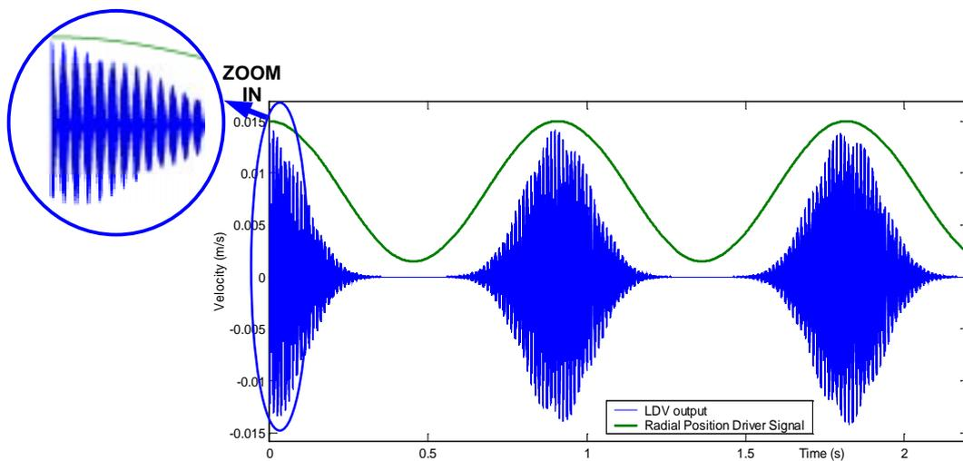
**Figure 5. 94** LDV output time history when the laser beam scans in a spiral pattern over the surface of the disc vibrating at the natural frequency of 2026 Hz. The zoom shows clearly the signal modulation given by the circumferential motion of the laser beam.
