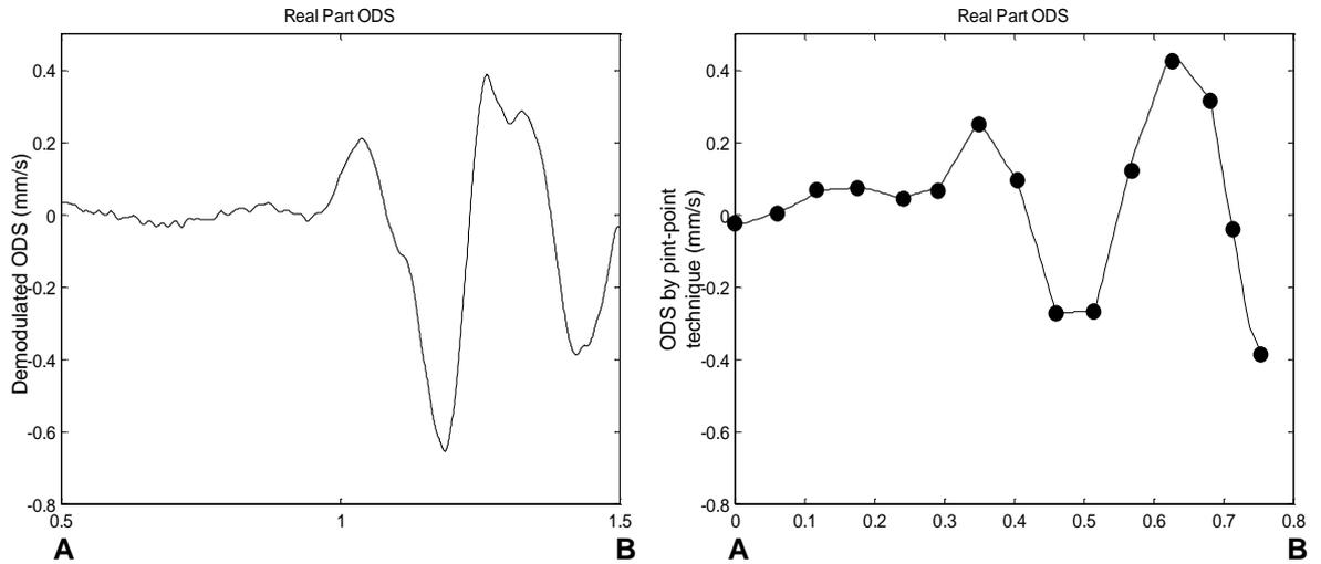
Figure 7. 31 ODS Real component (mm/s) derived by demodulation (left) and point-by-point scan (right, the vibration response is measured at the marked points only, where the actual measurements have been acquired).
