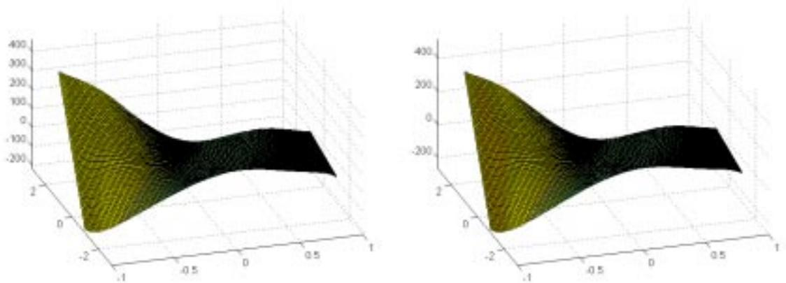
**Figure 5. 124** Real part of the mode shape at the natural frequency of 34.86 Hz derived from original (left) and corrected (right) modal constants.
