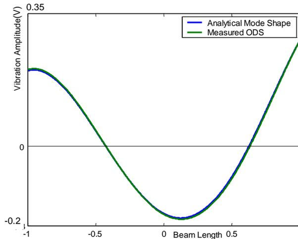
**Figure 5. 26** Analytical mode shape and measured ODS at 311 Hz.
