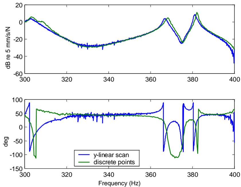
**Figure 7.14** Rotation mobility in x-direction derived at point 37 by vertical line scan – amplitude (top) and phase (bottom).
