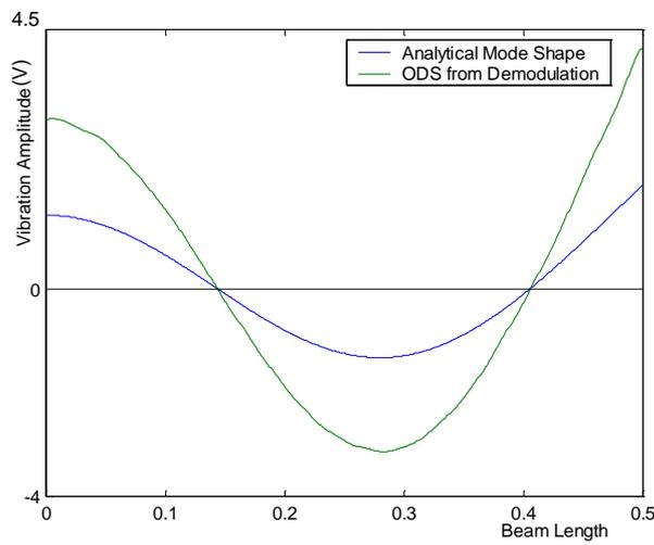
**Figure 5. 9** Analytical mode shape and ODS at 311 Hz.
