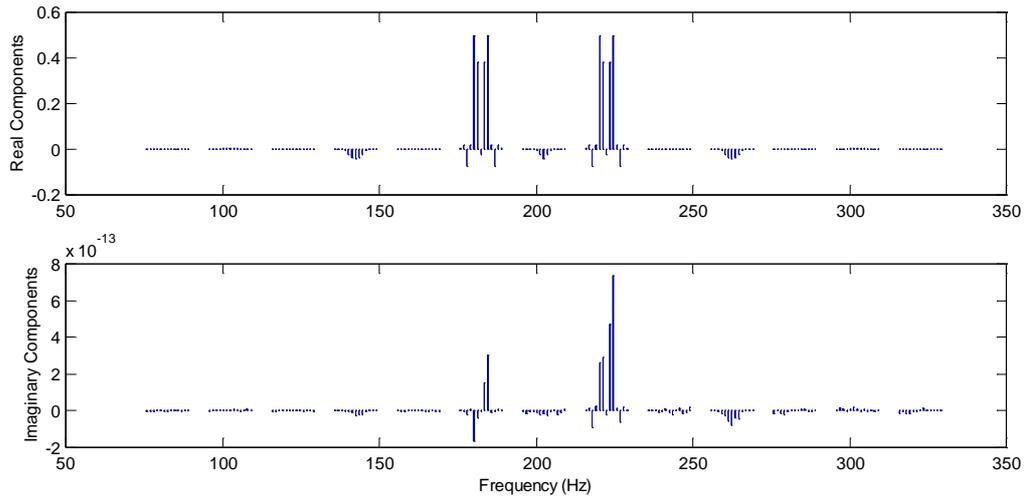
**Figure 5. 60** Real and imaginary components (in V) of the LDV output spectrum.
