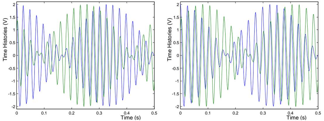
**Figure 2.18** Plot of the output signal from the first detector (blue) and the output signals from the second detector (green) being  $f_D$  positive in the first picture and negative in the second one.
