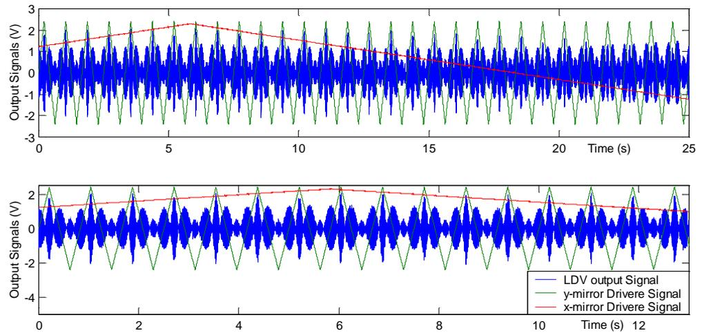
**Figure 7. 53** LDV output signal and mirrors driver signals within a complete acquisition (25 s) in the top plot, and zoomed signals in the bottom plot.
