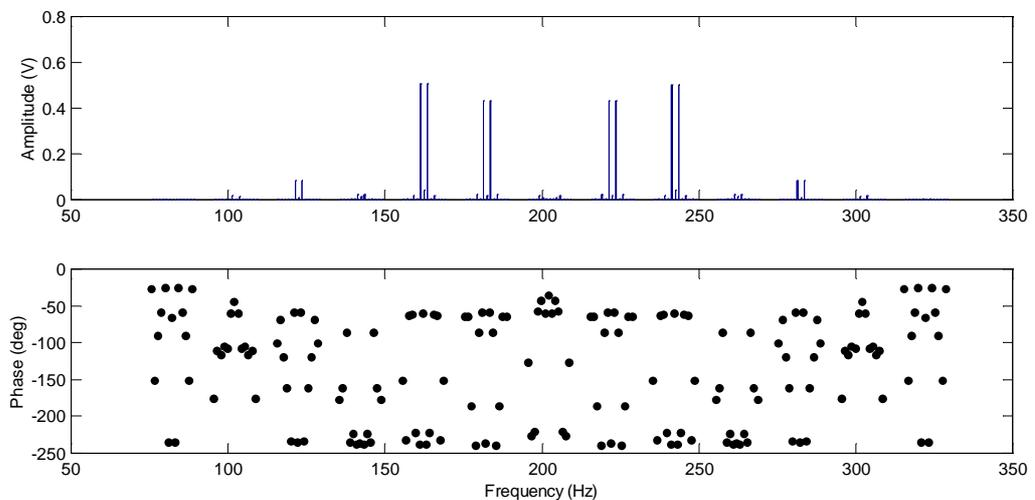
**Figure 5. 78** LDV output spectrum in magnitude and phase format.
