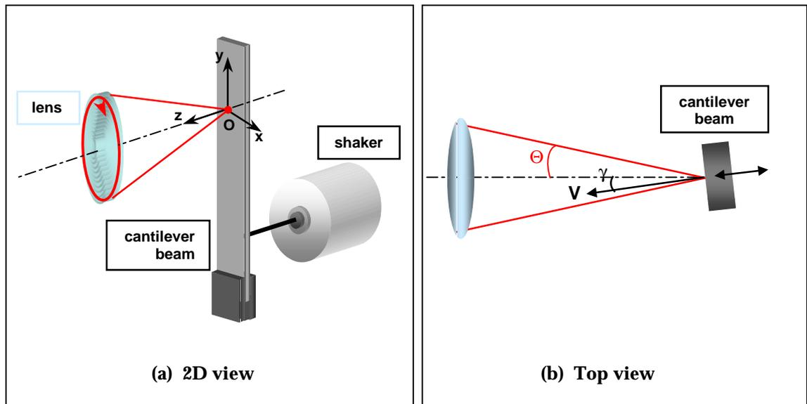
**Figure 4. 17** Conical scan set-up on the beam.
