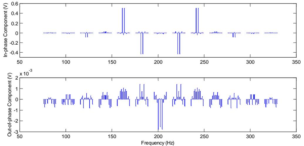
**Figure 5.83** In-phase and Out-of-phase components of the LDV output spectrum.
