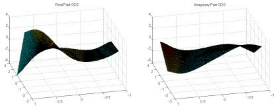
**Figure 5.109** Real and imaginary ODS at 34.8 Hz.
