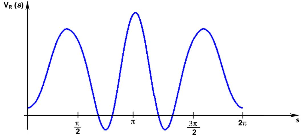
**Figure 5.33** Polynomial ODS along the rectified circle scanned on the plate.
