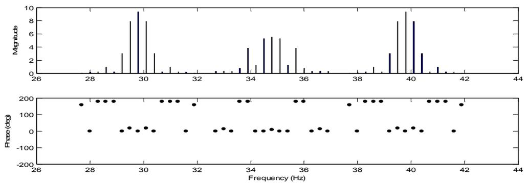
**Figure A. 18** Sideband FRF at the excitation frequency of 34.8 Hz.
