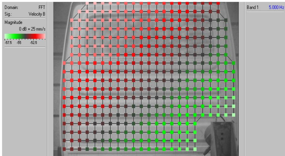
**Figure 7. 24** Acquisition points grid –rear panel of the lorry cab.
