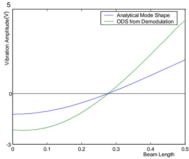
**Figure 5. 8** Analytical mode shape and ODS at 58 Hz.
