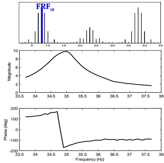
**Figure 5.112** FRF relative to the central component of the left sidebands group in the LDV spectrum ( $n = 1, m = 0$ ) as emphasised in the top diagram.
