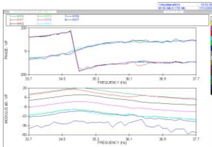
**Figure 5.119** Conventional FRFs analysed by ICATS ( $FRF_{10}$ ,  $FRF_{11}$ , ...,  $FRF_{17}$ ).
