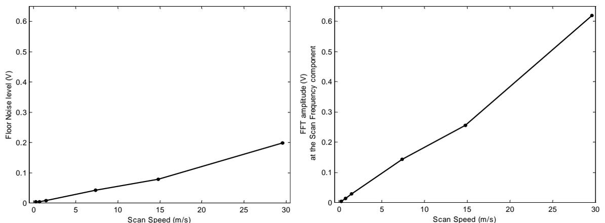
**Figure 6. 6** Noise, plotted against scan speed – scan at uniform rate.
