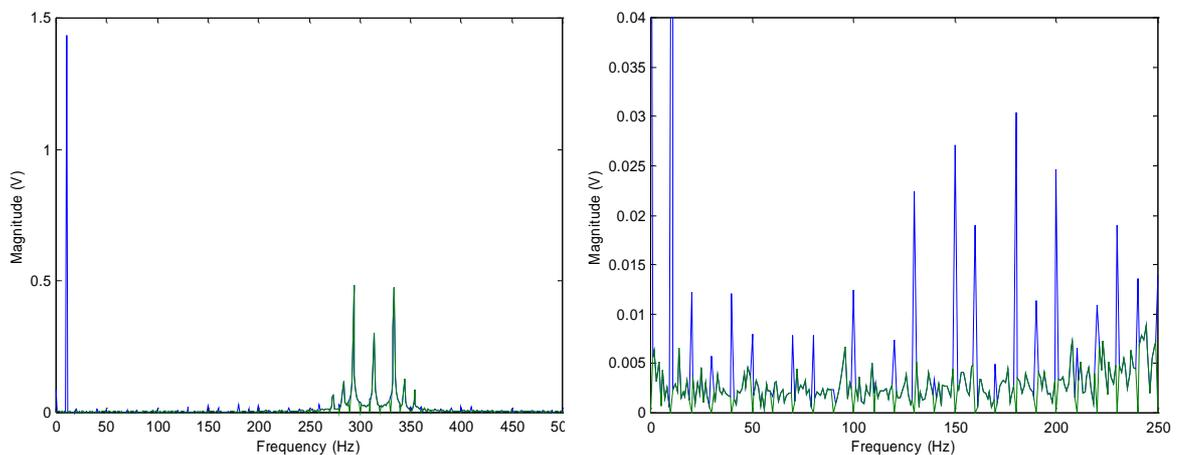
**Figure 6. 21** Spectral components of the original time history (blue) and the filtered one (green). The left plot is a zoom in the low-frequency range – Resonance frequency at 311 Hz.
