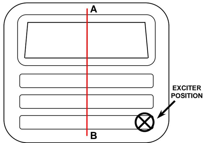
**Figure 7. 26** Linear scan at the middle of the panel.
