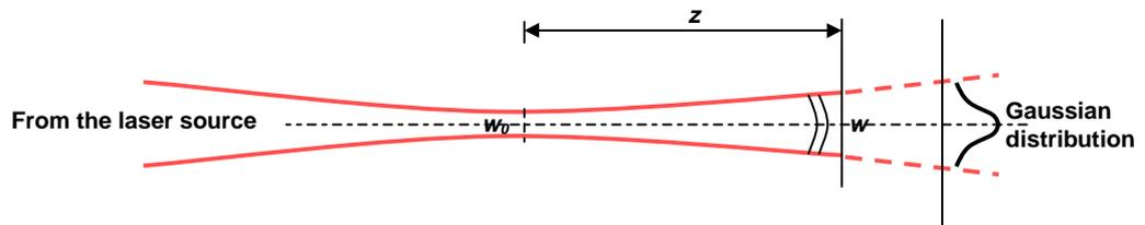
**Figure 2.5** Gaussian light beam profile.
