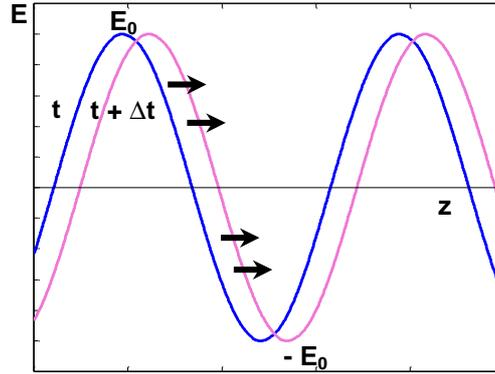
**Figure 2. 4** Electric field fluctuation along its direction of propagation.
