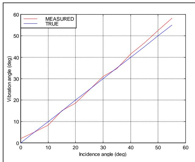
**Figure 4. 18** Accuracy of Vibration Direction measured by Conical Scan.
