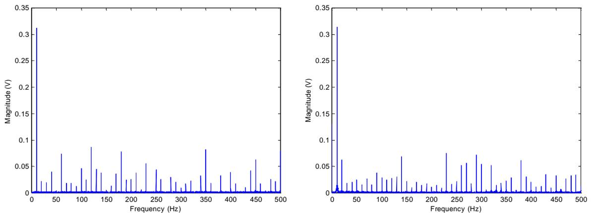
**Figure 6. 12** Simulated (left-hand plot) and measured (right-hand plot) LDV output spectrum.
