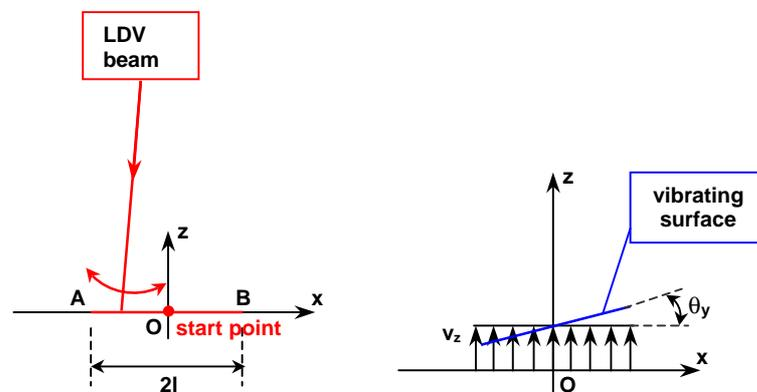
**Figure 4. 6** Laser beam scan and vibration DOFs associated to the surface.
