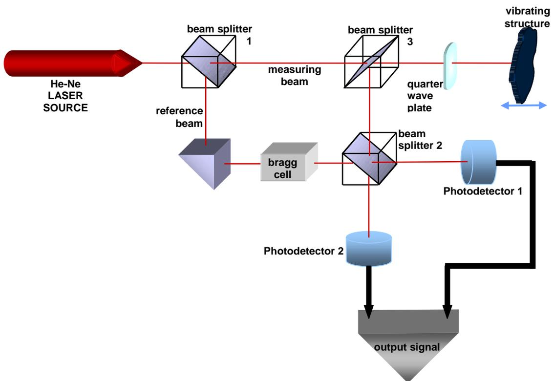
**Figure 2. 21** Polytec LDV arrangement.
