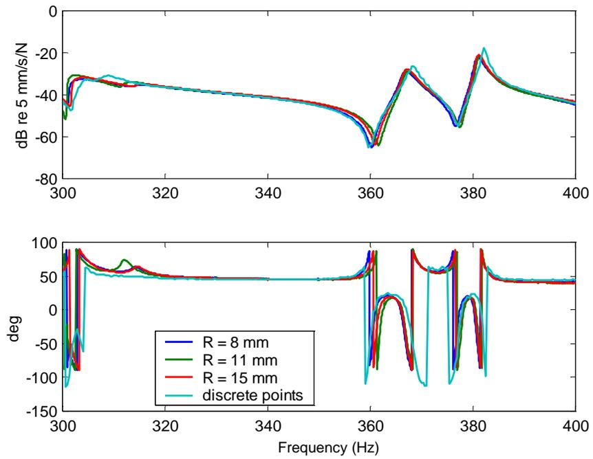
**Figure 7. 17** Translation mobility amplitude and phase derived at point 37 by circular scan with different scan radii.
