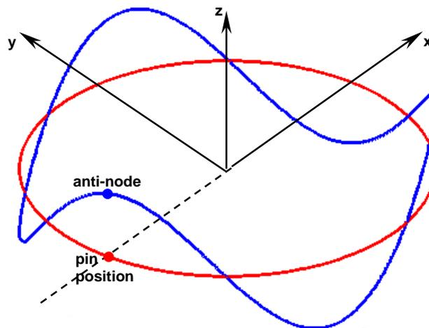
**Figure 5.50** 3-nodal diameter ODS at 2307 Hz. Standing wave with an antinode at the pin position.
