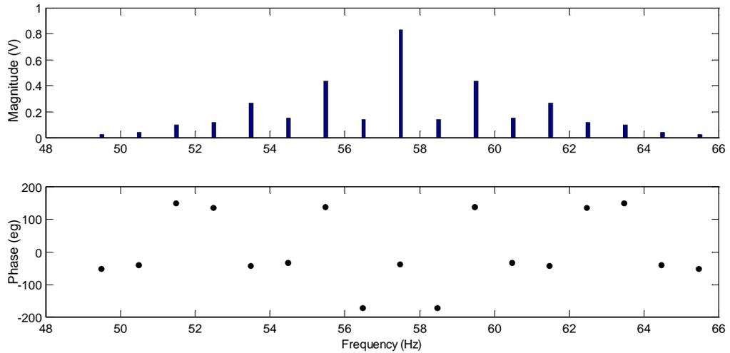
**Figure 7. 41** LDV spectrum magnitude and for  $\pm 8$  sidebands.
