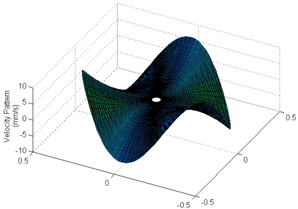
**Figure 5. 102** Two-dimensional ODS at 2271 Hz.
