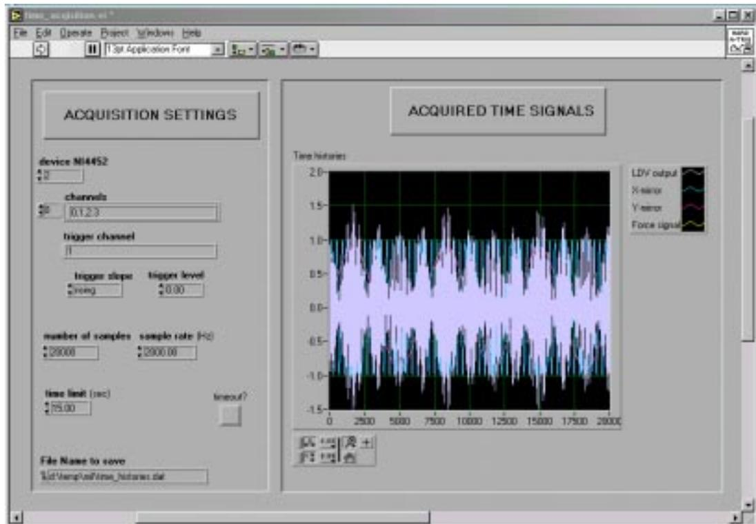
**Figure A. 3** Acquisition control panel.
