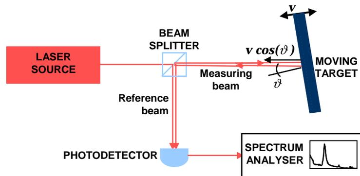
**Figure 2. 1** Basic LDV arrangement.
