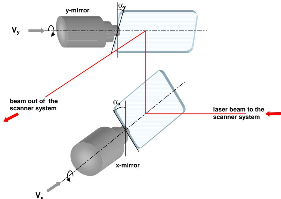
**Figure 3. 1** Schematic representation of the mirrors rotation.
