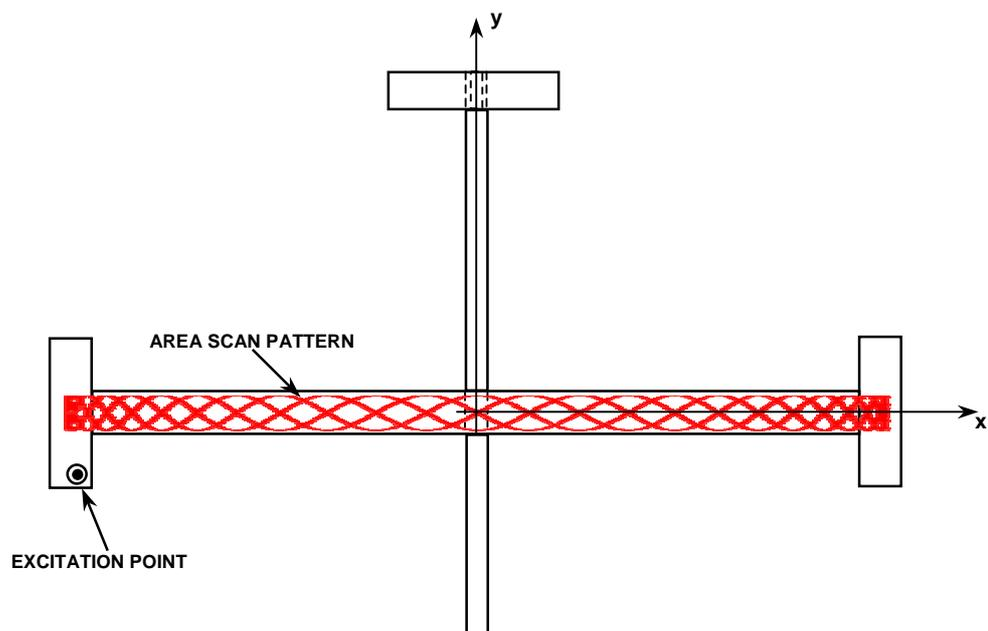
**Figure 5. 105** Excitation and LDV continuous-scan path.
