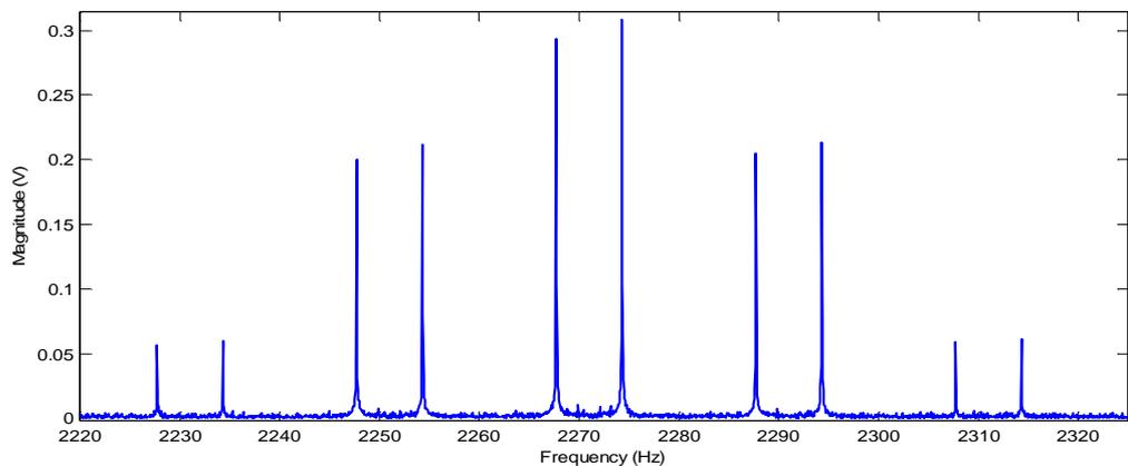
**Figure 5. 99** LDV signal spectrum for the daisy scan and excitation at 2271 Hz.
