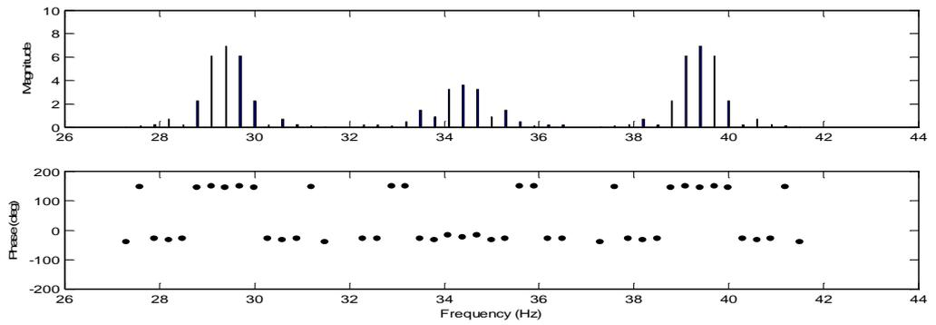
**Figure A. 14** Sideband FRF at the excitation frequency of 34.4 Hz.
