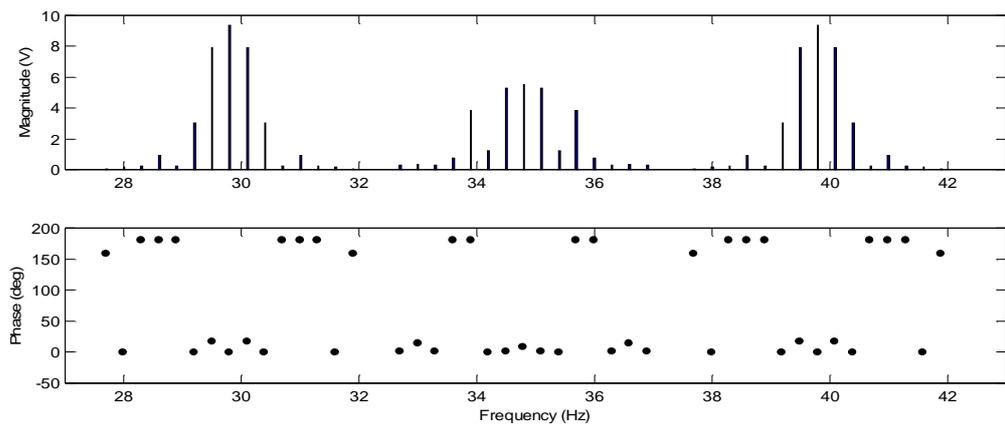
**Figure 5.108** Area scan LDV signal spectrum components.
