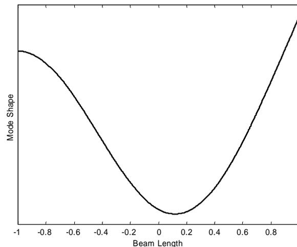
**Figure 6.13** Third mode shape of the beam (311 Hz) derived from the second equation of (5.8) - Timoshenko theory.
