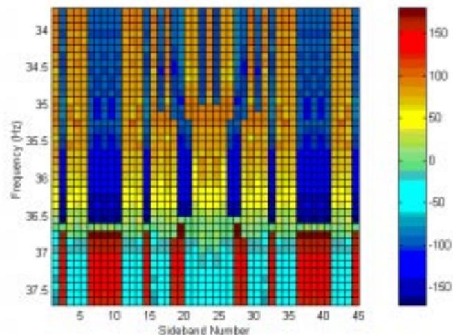
**Figure 5. 117** Color map of the overall plot of the sideband FRFs in phase.
