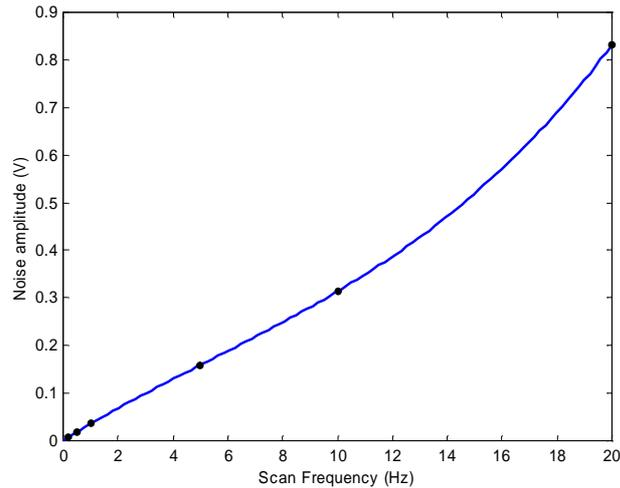
**Figure 6.10** Measured noise level data (black dots) and their polynomial curve-fit (blue line).
