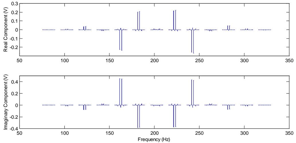
**Figure 5. 79** Real and imaginary components of the LDV output spectrum.
