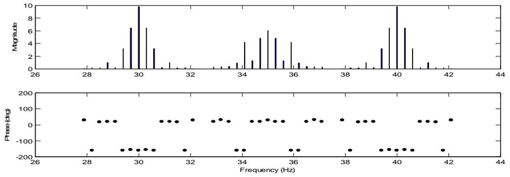
**Figure A. 20** Sideband FRF at the excitation frequency of 35 Hz.
