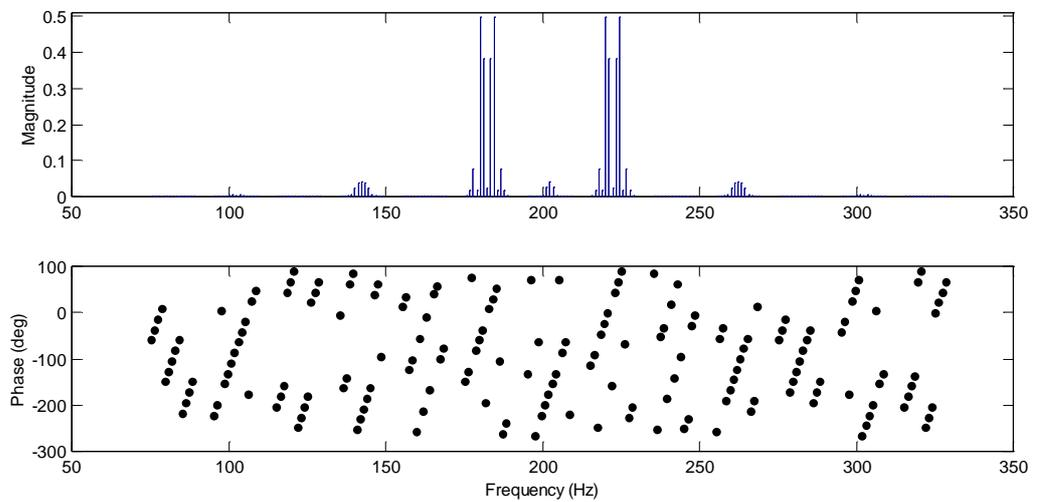
**Figure 5.69** LDV spectrum in the real situation without considering the mirror delay.
