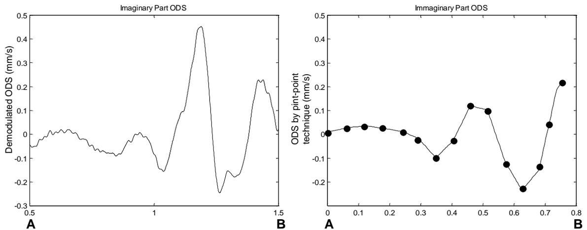
**Figure 7.32** ODS Imaginary component (mm/s) derived by demodulation (left) and point-by-point scan (right, the vibration response is measured at the marked points only, where the actual measurements have been acquired).
