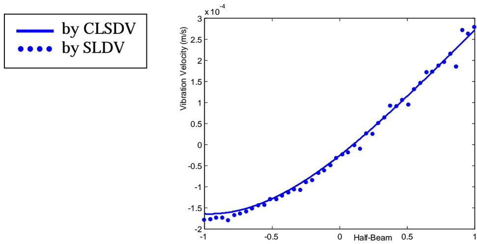
**Figure 5. 29** ODS corresponding to the first mode.
