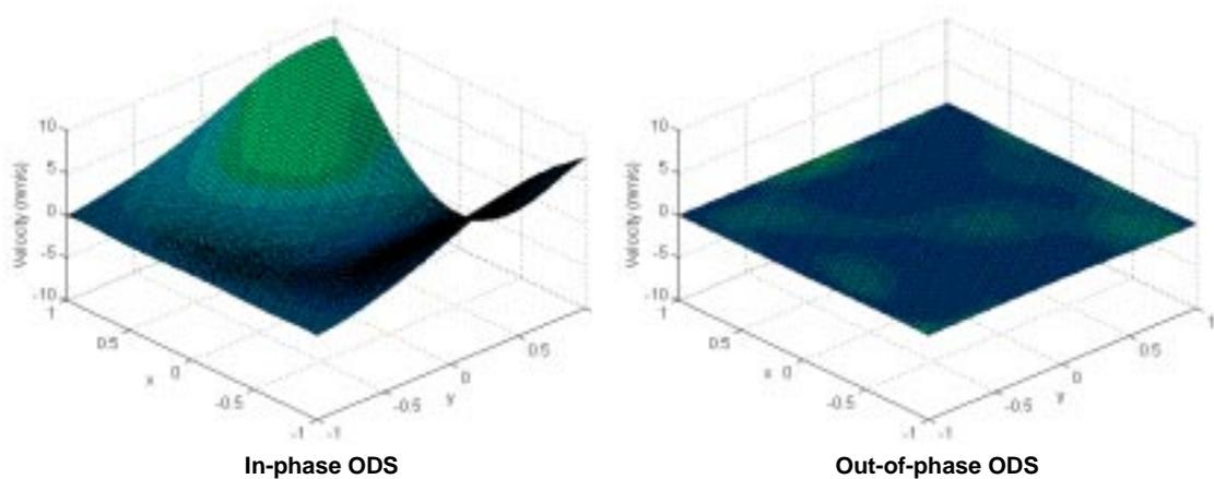
**Figure 5. 87** Vibration pattern from the continuous area scan at 241.25 Hz.
