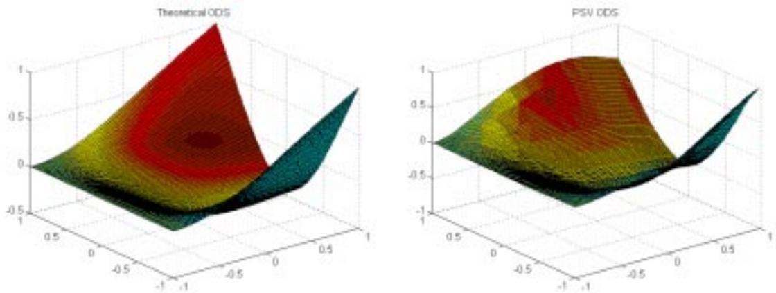
**Figure 3. 9** ODS at 239.1 Hz (5<sup>th</sup> Mode).
