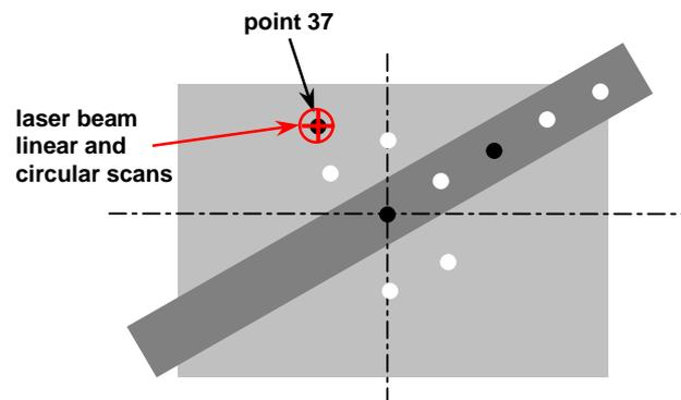
**Figure 7. 9** Point measurement on the “breadboard” structure.
