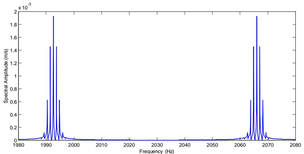
**Figure 5.96** LDV output time history when the laser beam scans over a spiral pattern on the surface of the disc vibrating at the natural frequency of 2026 Hz.
