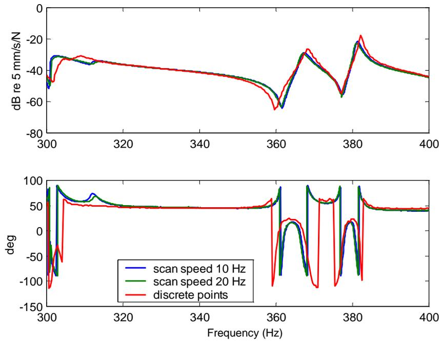
**Figure 7. 20** Translation mobility amplitude and phase derived at point 37 by circular scan with different scan speeds.
