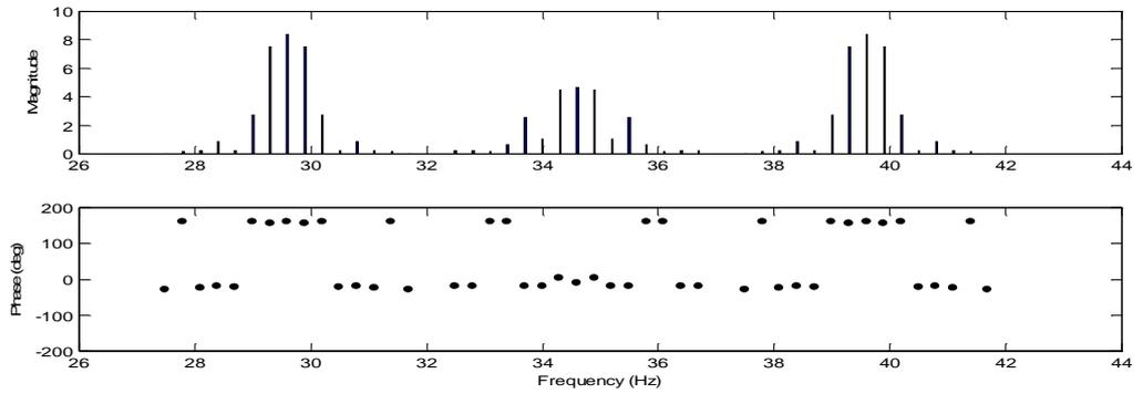
**Figure A. 16** Sideband FRF at the excitation frequency of 34.6 Hz.
