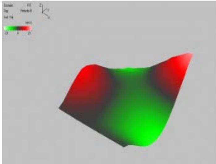
**Figure 3. 6** ODS at 181.9 Hz.
