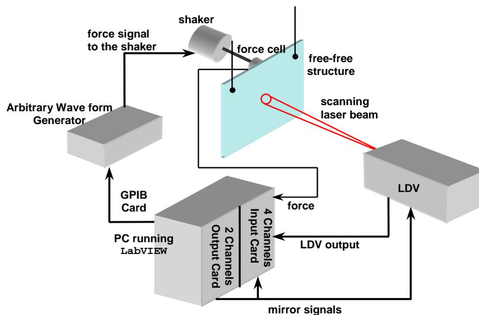
**Figure 7. 5** Schematic representation of measurement system.
