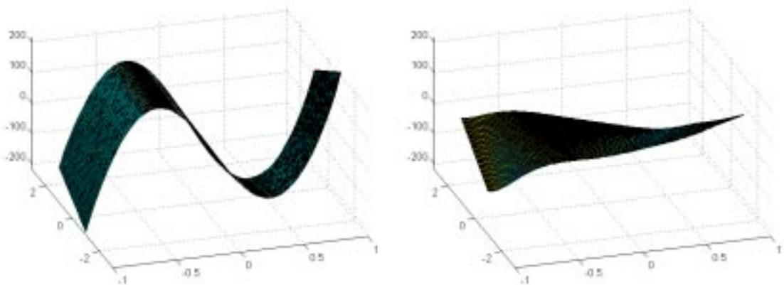
**Figure 5. 126** Real (left) and imaginary (right) part of the mode shape at the natural frequency of 36.55 Hz derived from corrected modal constants.
