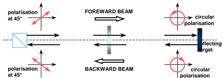
**Figure 2. 22** Quarter wave plate working principle.
