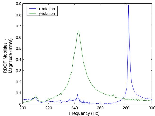
**Figure 7.8** Angular mobilities amplitude.
