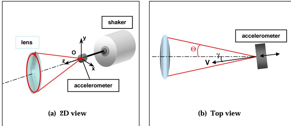
**Figure 4. 15** Accelerometer/Shaker set-up for Conical Scan trial.
