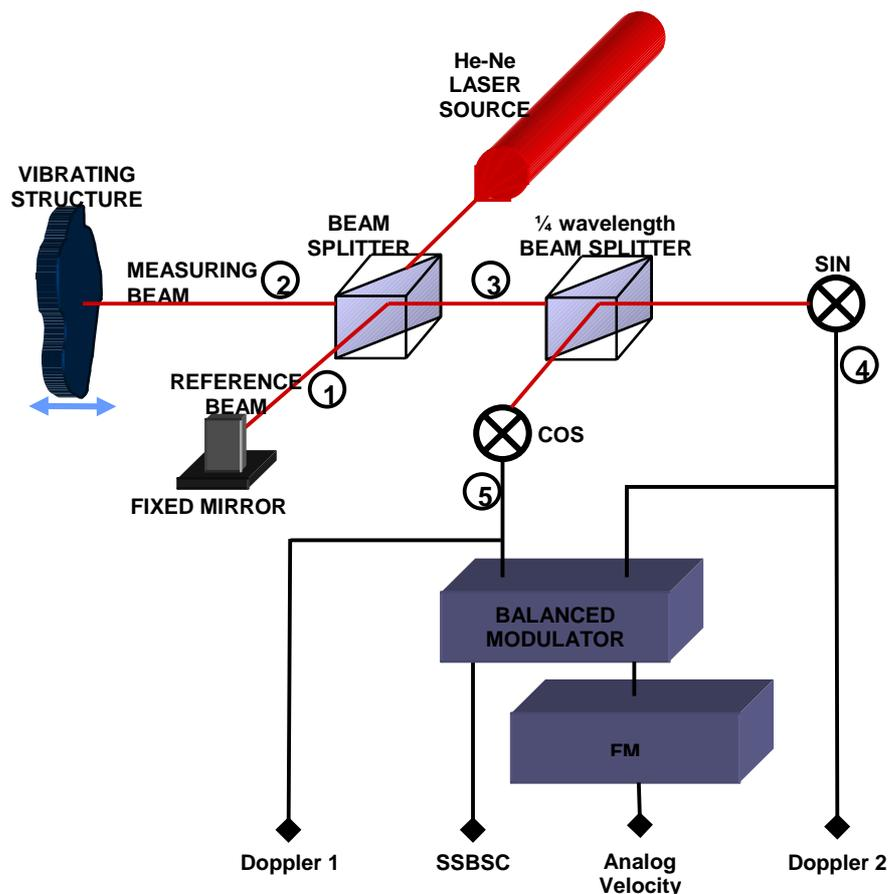
Figure 2. 23 Ometron VPI configuration.
