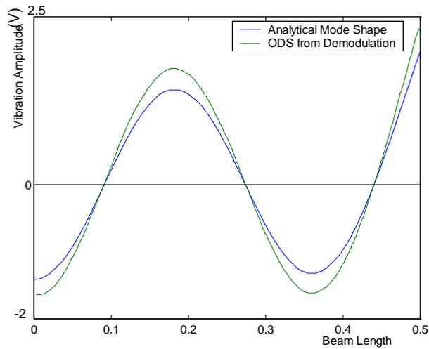
**Figure 5. 10** Analytical mode shape and ODS at 766 Hz.
