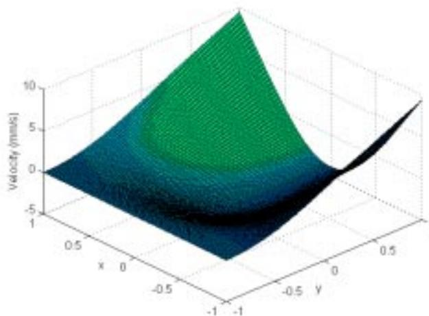
**Figure 5. 89** Analytical 5<sup>th</sup> mode shape at 242.68 Hz.
