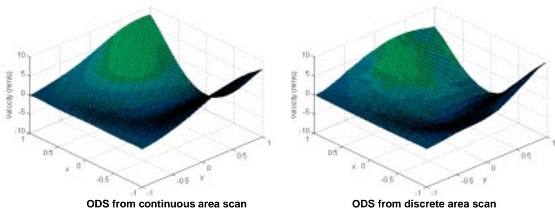
**Figure 5. 88** Vibration patterns at 241.25 Hz from continuous area scan and the conventional Polytec step-point area scan.
