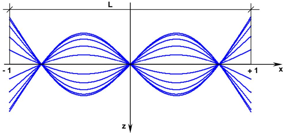
**Figure 5.11** Vibration pattern at different time instants.
