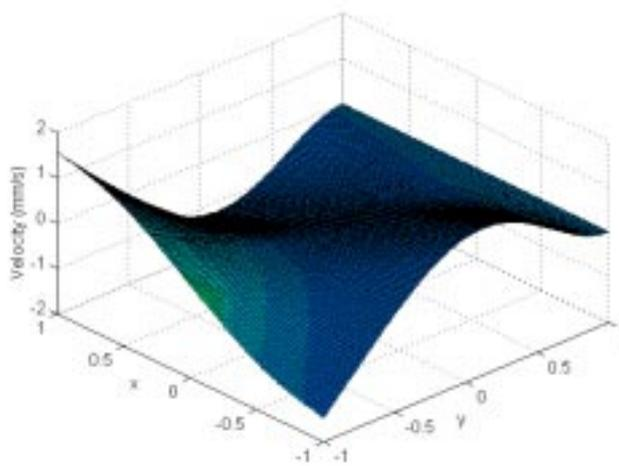
**Figure 5. 86** Analytical 4<sup>th</sup> mode shape at 202.4 Hz.
