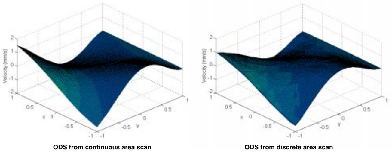
**Figure 5. 85** Vibration patterns at 202.5 Hz from continuous area scan and the conventional Polytec step-point area scan.
