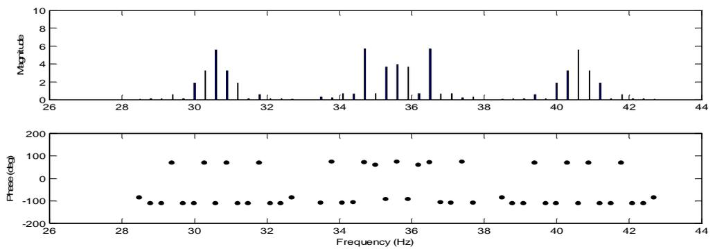
**Figure A. 26** Sideband FRF at the excitation frequency of 35.6 Hz.
