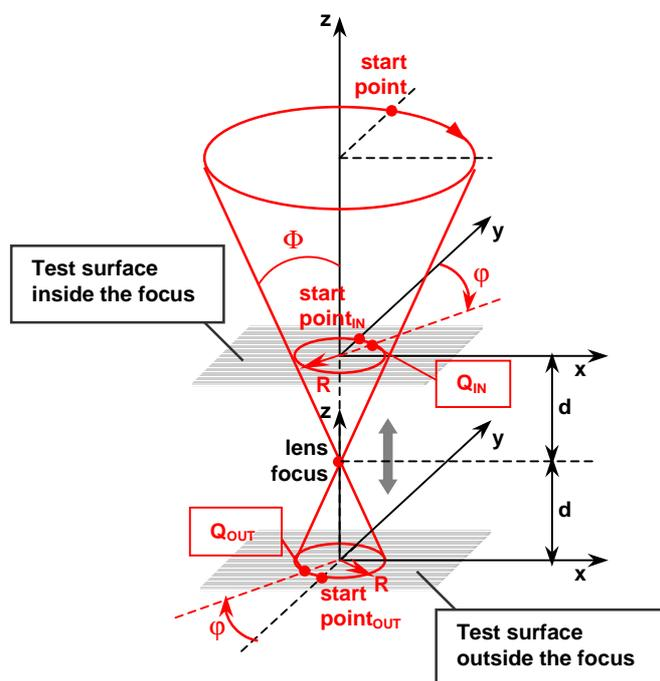
**Figure 4. 20** Conical-circular scan configuration.
