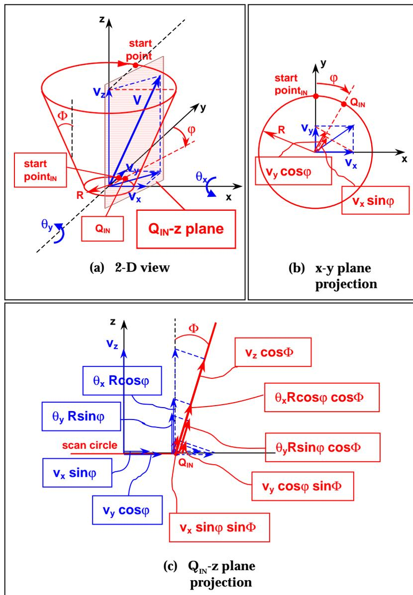
Figure 4. 21 Inside-focus conical-circular scan.
