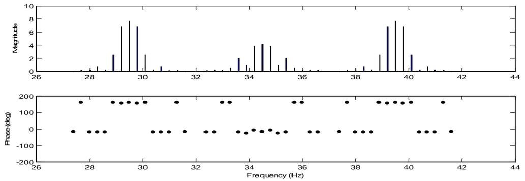
**Figure A. 15** Sideband FRF at the excitation frequency of 34.5 Hz.
