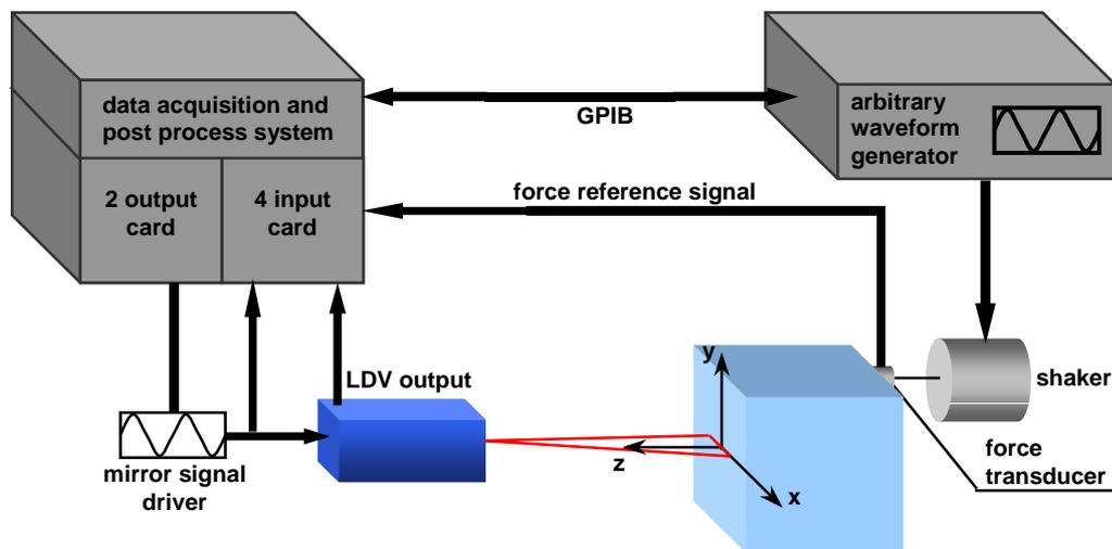
**Figure 4. 5** Schematic of the tested structure and the measurement equipment.
