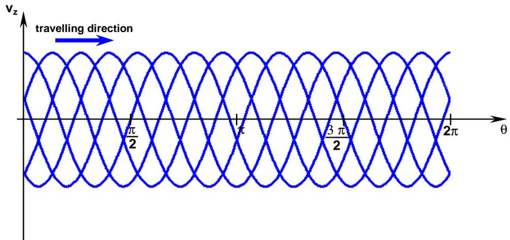
**Figure 5. 39** Travelling wave on the disc circumference, case of 3-diameter mode.
