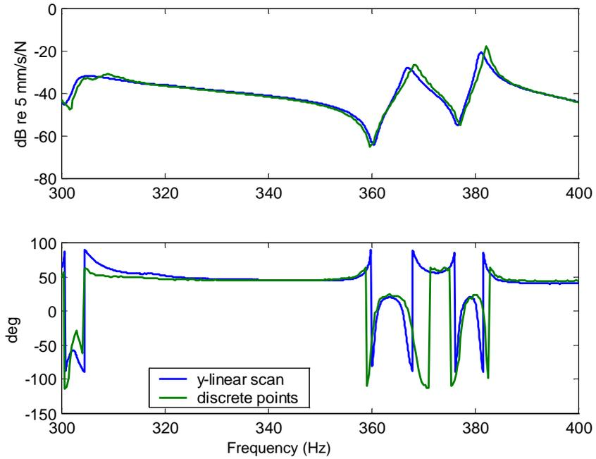
**Figure 7.13** Translation mobility amplitude and phase derived at point 37 by vertical line scan.
