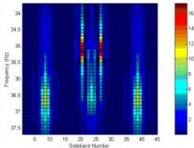
**Figure 5. 115** Color map of the overall plot of the sideband FRFs in magnitude (red color corresponds to the maximum vibration response).
