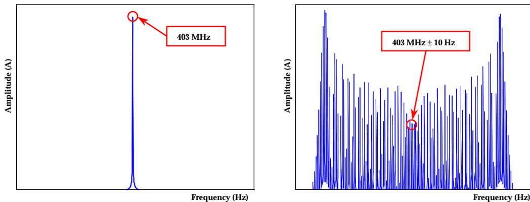
**Figure 6. 1** Simulated light intensity collected at the photodetector (which is sensitive to current signals, i.e. Ampere) for phase fluctuation zero (left) and non-zero (right).
