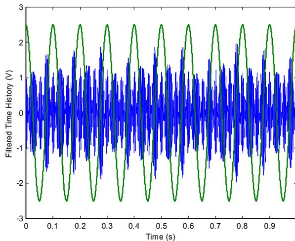
**Figure 6. 20** Time history deprived of the periodic noise (blue) and mirror driver signal (green) – Resonance frequency at 311 Hz.
