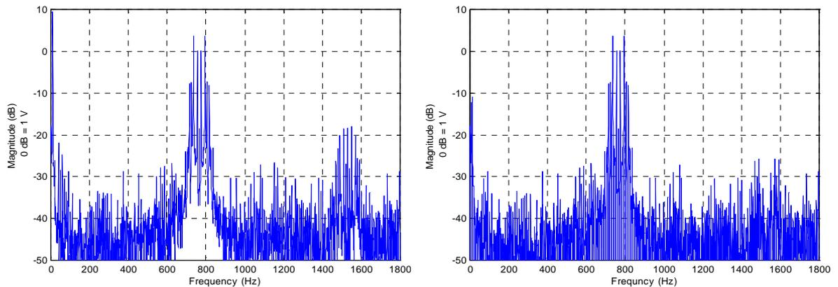
**Figure 6. 25** Fourier spectrum amplitude in dB for the original measured signal (left) and the filtered one (right).
