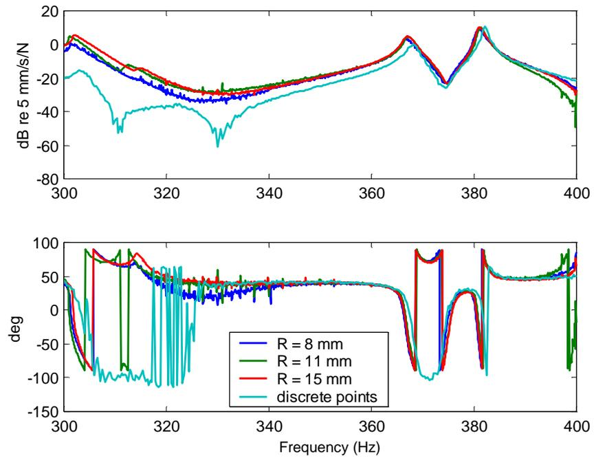
**Figure 7. 19** Rotation mobility in y-direction derived at point 37 by circular scanning- amplitude (top) and phase (bottom).
