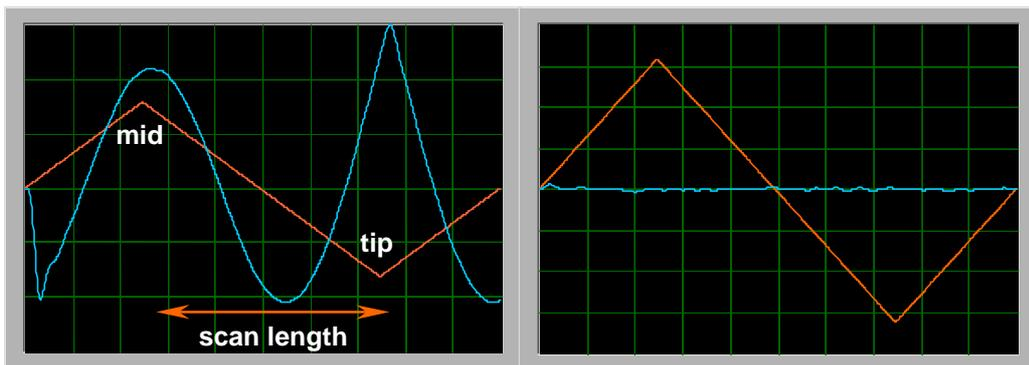
**Figure 5. 6** In-phase and out-of-phase components of the ODS at 311 Hz.
