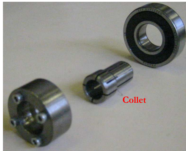
Figure 7 - 6 Bearing-shaft adaptor and collet fixture
