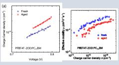
The burn-in process induced the formation of additional intra bandgap states, causes more severer charge trapping and leads to reduced charge carrier mobility.
