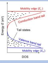
The tail states distribution can be described by exponentially decay towards the bandgap (similar distribution to Gaussian) below the band edge.
