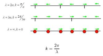
In this case, as k increases, the energy of vibration increases and the frequency too.
