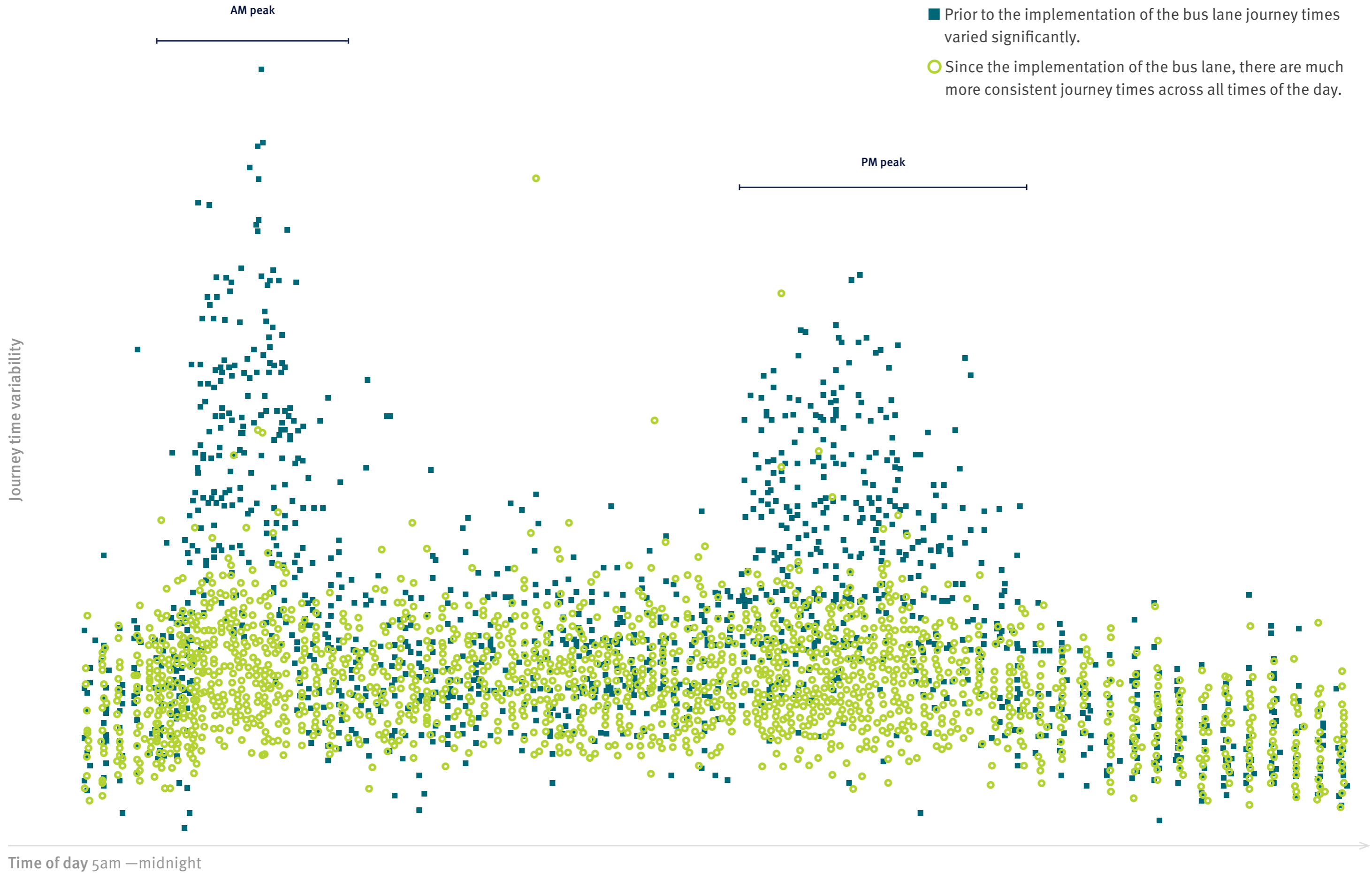
Figure 2 Bus journey time variability pre- and post-implementation of bus lane Original source: Société des Transports Intercommunaux de Bruxelles, 2012
