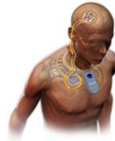
Wireless, multi-channel neural recording interface with on-node spike sorting for real-time motor prosthetic control
