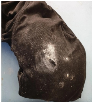
Figure 14: Tier 1 pelvic personal protective equipment worn on cadaveric thigh; post-impact delivered to region of two-layer high-performance knitted silk protection
