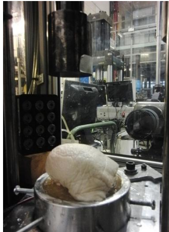
Figure 22: Testing apparatus for drop tests on a cadaveric human heel fat pad.
