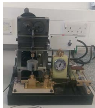
Pressure generating unit
