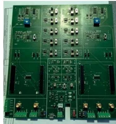
A PCB platform for testing the multichannel pH and CAP recording chip.
