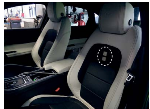
Overview of static radar measurements of heart and respiration motions (left) using a car seat equipped with a single UWB sensor located in the backrest (right)
