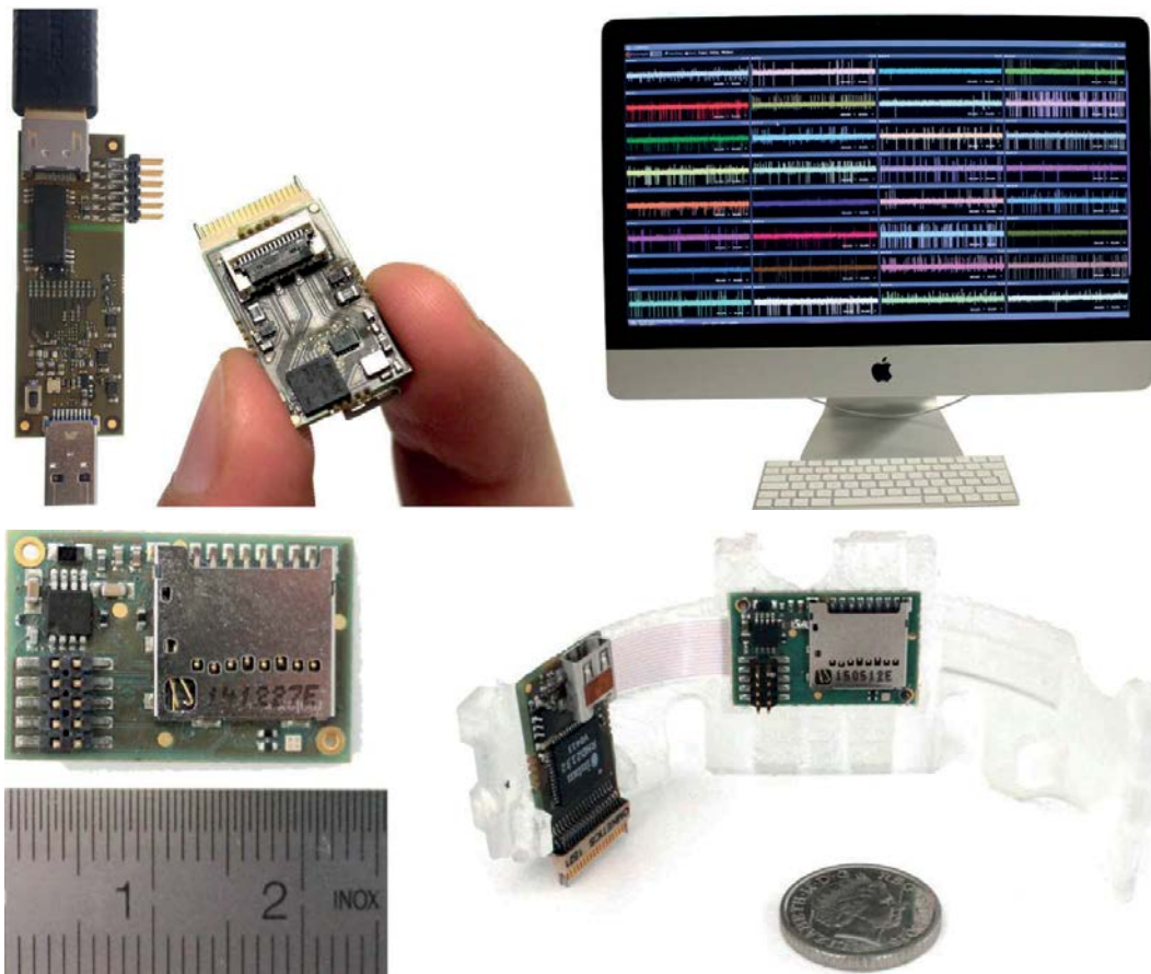
NGNIv1 hardware spike sorting headstage. Shown are: USB3.0 SuperSpeed bridge (top left); 32-channel spike sorting headstage (top centre); and software environment for configuration and real-time visualization (top right); controller with MicroSD logger (bottom left); and standalone configuration for chronic recordings (bottom right).
