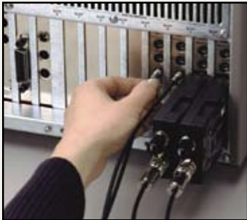
It's easy to connect the Model 4200-SCS to a probe station or a switch matrix with standard triax cables.
