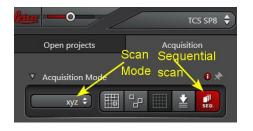
• Re-load the same settings as used in a previous image. Open the image library and select the image, then click on the APPLY icon above (check the pixel number, bit depth and zoom and averaging as these are not always re-loaded).
