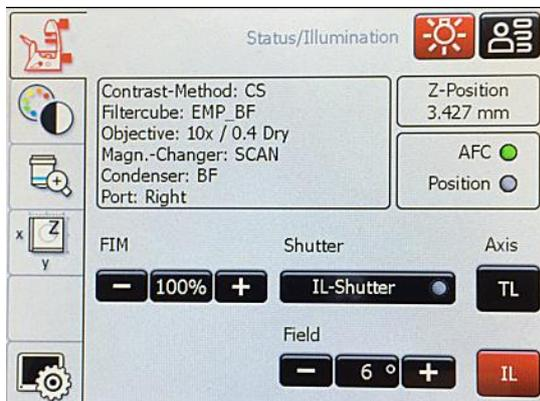
To Adjust the Brightfield use the microscope tab, open the brightfield (IL) shutter, and adjust intensity and condenser aperture, using the controls on the left side of the microscope stand
