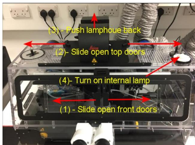
The chamber light can also be controlled with a footswitch once turned on
