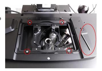
Mount the incubator base in the galvo stage and fasten the 4 screws. You can adjust the little spring brackets to better fit the 35 mm dish (use screwdriver). Fill the water reservoir if needed. Take care not to spill water inside the
