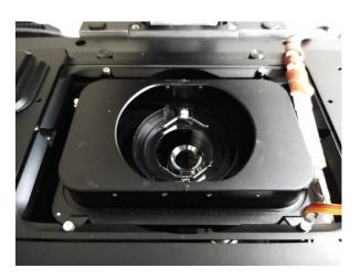
Fit the required insert (10x or 25x) that matches the detection objective into the round top plate. The 20x objective fits the 10x insert.
