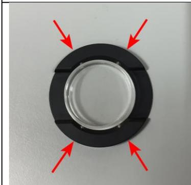
Loosen the screws on the ring clamp and on a flat surface, place the 35mm dish into the clamp. Tighten screws to just hold the dish (DO NOT OVER TIGHTEN).
