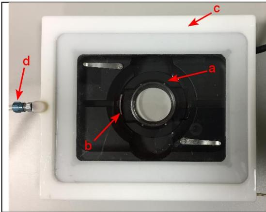
Inset the clamp and dish (a) into the stage by sliding the clamp against the spring plate (b).
